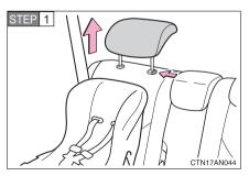
Remove the head restraint.
