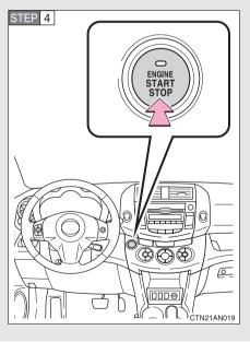
Press the "ENGINE START STOP" switch.
