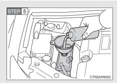
Add engine coolant if necessary.
