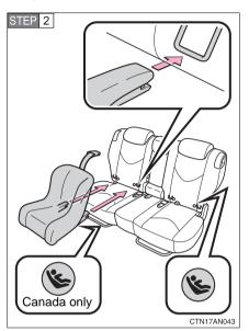
Latch the buckles onto the LATCH anchors.
