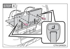
Pull the seatback lock release strap to fold down the seatback.
