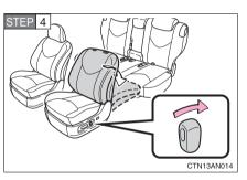
Move the seatback angle adjusting switch backward to flatten the seatback.
