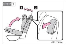
Fold the seatback while pulling the lever. Return the seatback and secure it at the 1st lock position (most upright position). Adjust the seatback to the 3rd lock position. (→P. 54)
