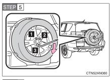
Using the wheel nut wrench, tighten the hold-down nuts by turning them clockwise. Follow the order shown in the illustration.
