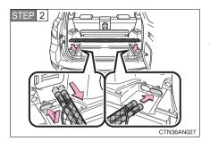
Insert the right end of the pipe into the recess, then compress the left end of the pipe and insert it into the recess.
