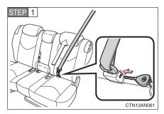
Insert the key into the hole on the center seat belt buckle to release the tab (with hook end), and allow the belt to retract.
