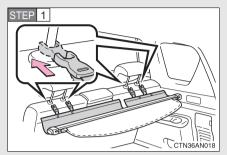
Attach the hooks to the head restraints.
