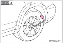
Slightly loosen the wheel nuts (one turn).
