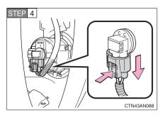
To unplug the connector, depress the lock release while pulling downward.
