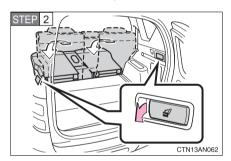
Open the back door and pull the lock release lever to fold down the second seat.
