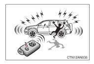
When (t) is pushed for longer than about one second, an alarm will sound for about 60 seconds and the vehicle lights will flash to deter any person from trying to break into or damage your vehicle.
