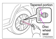
Tighten the nuts until the tapered portion comes into loose contact with the disc wheel seat.
