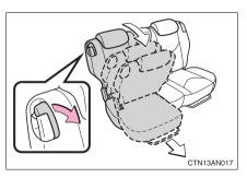
Pull the lever forward and fold down the seatback. The seat will slide forward.
