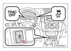
Push and hold the button while the vehicle is stopped to turn off TRAC and Enhanced VSC.
