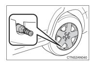
Align the cutout of the wheel ornament with the valve stem as shown.
