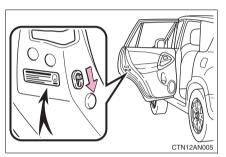
The door cannot be opened from inside the vehicle when the child-protector lock is set.
