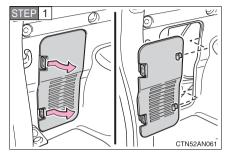
Disengage the claws and remove the cover.
