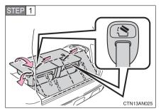
Pull and hold the seat lock release strap and lift up the seat rearward and then push the seat down.
