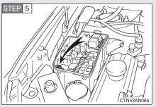
Remove the fuse with the pullout tool.
