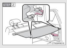
Pull out the luggage cover and hook onto the anchors.
