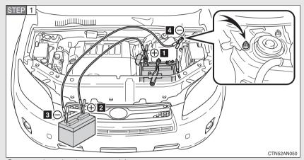
Connecting the jumper cables
