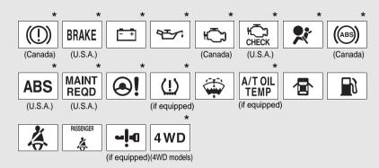
\*: These lights turn on when the "ENGINE START STOP" switch is turned to IGNITION ON mode (vehicles with smart key system) or the engine switch is turned to the "ON" position (vehicles without smart key system) to indicate that a system check is being performed. They will turn off after the engine is started, or after a few seconds. There may be a malfunction in a system if a light does not come on, or if the lights do not turn off. Have the vehicle inspected by your Toyota dealer for details.
