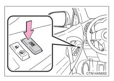
Press the switch down to lock the passenger window switches.
