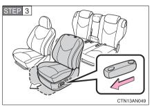
Push the seat position adjusting switch forward to slide the seat to the front-most position.
