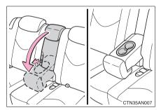
To use the cup holders, pull the strap forward and fold down the center seatback.
