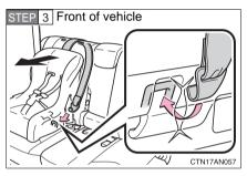
Secure the child restraint using the seat belt. Latch the hook onto the anchor bracket and tighten the top tether strap.
