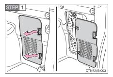
Disengage the claws and remove the cover.
