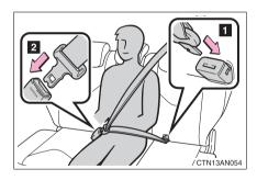
Make sure that the buckle **1** is securely latched ready for use of the center seat belt.
