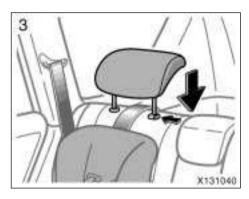
3. Insert the head restraint and push it down to the lock position.
