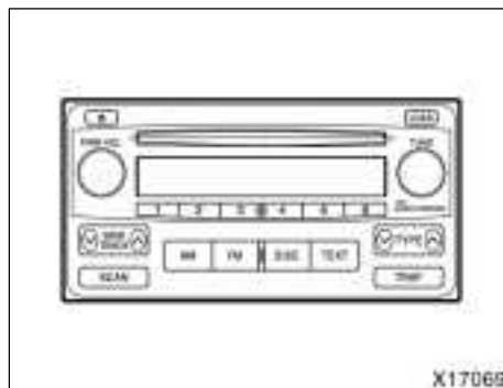
Type 2: AM-FM radio/compact disc player with changer
