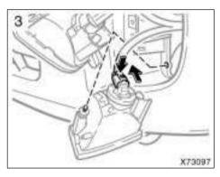
3. Unplug the connector while depressing on the tab.
