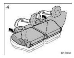
4. Pull the seatback lock release strap and swing the seatback up.
