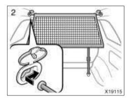
Insert one side of the net stay into the net fixing hole. Press the stay to contract and insert the other side of the stay into the other fixing hole. Push the net forward.
