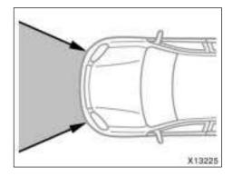
The SRS airbag system is designed to activate in response to a severe frontal impact within the shaded area between the arrows in the illustration.
