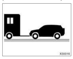
Your vehicle can be dinghy towed (with four wheels on the ground) from the front behind a motorhome.
