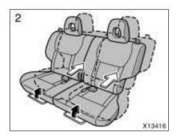
Hold the center of the lever and pull it up. Then slide the rear seat fully backward and pull it forward slightly till it locks.
