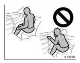
• Do not sit on the edge of the seat or lean over the dashboard when the vehicle is in use, since the airbags inflate with considerable speed and force. Otherwise you may be killed or seriously injured. Sit up straight and well back in the seat, and always use your seat belt properly.
