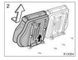
2. Unlock the seat by pulling the lock release lever. Pull the seat toward you slightly and lift.
