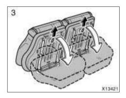
3. To unlock the seat, hold the upper back of the seat with your hand and pull the lock release strap up. Swing the whole seat down and set the rear legs to the hooks on the floor. Make sure the rear legs are securely set to the hooks by trying to pull up the rear part of the seat.
