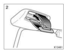
Insert the round end tab into the cover. You will hear a click when the tabs are locked in the seat belt cover. Make sure the tabs are securely locked in the cover.
