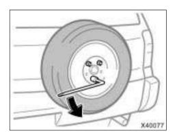
Turn the hold-down nuts counterclockwise with the wheel nut wrench and remove them.
