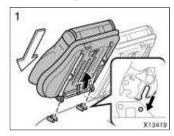
1. While pulling up the lock release lever, place the rear hinge into the rear hook on the floor.
