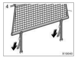
4. Pull the end of the belt to stretch the net securely.
