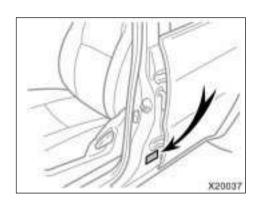
The vehicle identification number (VIN) is also on the Certification Regulation Label.
