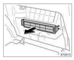
2. Remove the filter case from the filter outlet as shown in the illustration.
