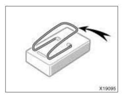
Please note if transmitter has wire clip for sun visor, this clip must be removed prior to adhesion of the Velcro.
