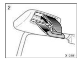
Insert the round end tab into the cover. You will hear a click when the tabs are locked in the seat belt cover. Make sure the tabs are securely locked in the cover.
