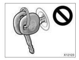
♦ When starting the engine, do not use the key with other transponder keys around (including keys of other vehicles) and do not press other key plates against the key grip. Otherwise the engine may not start, or may stop soon after it starts. If this happens, remove the key once and then insert it again after taking off other transponder keys (including keys of other vehicles) from the ring or while gripping or covering them with your hand to start the engine.
