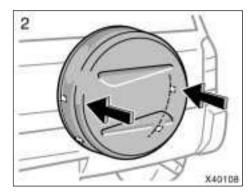
Push both sides of the cover and set the cover by hooking the 4 inside protrusions.
