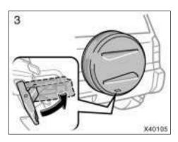
3. Lock the latch handle which is on the bottom of the cover.
