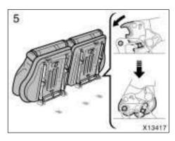
Make sure the front legs are locked and the seat is securely locked in position.
