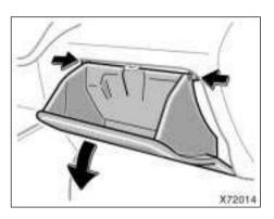
1. Push each side of the glove box to disconnect the claws.
