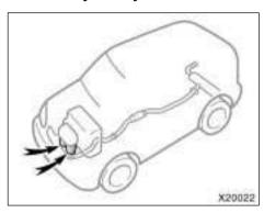
The three-way catalytic converter is an emission control device installed in the exhaust system.
