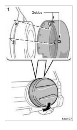
1. Insert the hooks under the guides to the upper slots and lower the cover.
