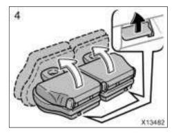
Pull up the seat cushion lock release lever and swing the whole seat up and forward.
