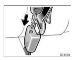
To release the concave end tab, insert the key into the hole on buckle 1 (with light gray buckle-release button) and allow the belt to retract.
