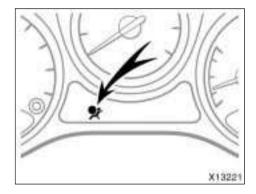
This front seat belt pretensioner system has a service reminder indicator to inform the driver of operating problems. If any of the following conditions occurs, this indicates a malfunction of the airbags or pretensioners. Contact your Toyota dealer as soon as possible to service the vehicle.
