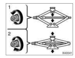
To remove the jack, move the seat to the rear-most position and turn the jack joint by hand.
