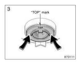
Install the rubber cover with the "TOP" mark upward, and fit it securely on the boss. Plug in the connector.
