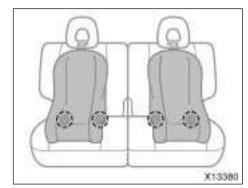
The lower anchorages for the child restraint system interfaced with the FMVSS225 specification are installed in the rear seat.
