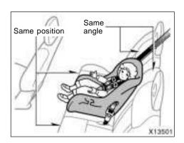
• When installing a child restraint system on the rear center position, adjust both seat cushions to the same position and align both seatbacks at the same angle. Otherwise, the child restraint system cannot be securely restrained and this may cause death or serious injuries in a collision.
