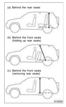
You can separate the luggage compartment by installing the separation net. You can choose one of the three positions.
