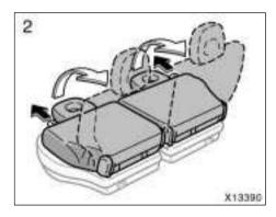
2. Pull the seatback lock release strap and swing the seatback up.
