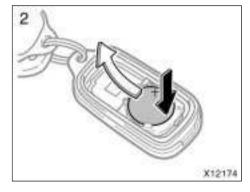
Remove the discharged transmitter battery.
