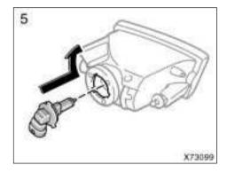
Install a new bulb and the connector into the mounting hole. Install the front fog light unit then the front turn signal light unit, and tighten the retainer screw.
