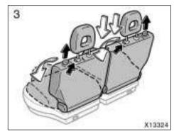
3. Lower the head restraint to the lowest position. Pull up the strap to unlock the seatback and fold the seatback forward until it locks.
