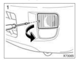
Loosen the retainer screw with a Phillips-head screwdriver and take out the front turn signal light unit.
