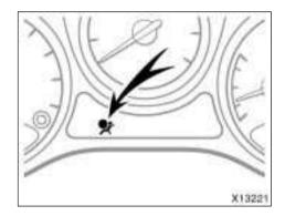
This SRS airbag system has a service reminder indicator to inform the driver of operating problems. If either of the following conditions occurs, this indicates a malfunction of the airbags. Contact your Toyota dealer as soon as possible to service the vehicle.
