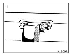
Remove the holder from the tailgate by turning the bolts counterclockwise.
