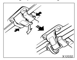
To tilt up the sun roof, first pull down on the handle while pushing in one of the lock buttons. Then push up the sun roof until it locks.
