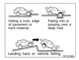
The SRS airbags may deploy if a serious impact occurs to the underside of your vehicle. Some examples are shown in the illustration.
