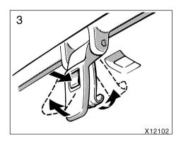
Separate the latch handle and hook while pressing the lock release button.
