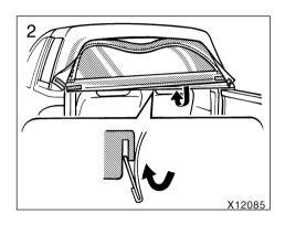
2. Align the retainer on the bottom of the window with the groove.
