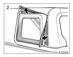
Remove the Velcros on the quarter window from the outside of the vehicle.
