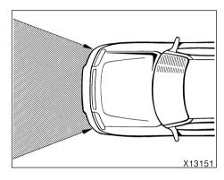
The SRS airbag system is designed to activate in response to a severe frontal impact within the shaded area between the arrows in the illustration.
