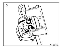
2. Press in the retaining spring arms and insert them into the holes. Then lock the sun roof by pushing the handle up with the palm of your hand until the handle clicks.
