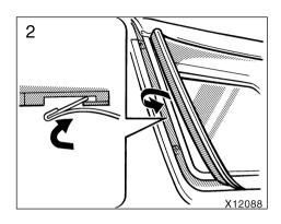
Insert the retainer on the side of the window into the groove on the vehicle side.
