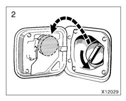
2. To remove the fuel tank cap, turn the cap slowly counterclockwise, then pause slightly before removing it. After removing the cap, hang it on the cap hanger.
