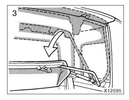
Fold the soft-top. Make sure to place the soft-top between the rear seat backs and tailgate.
