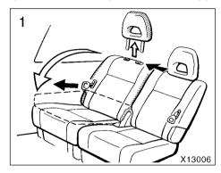
1. Remove the head restraint. Unlock the seatback and fold it down.
