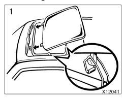
Insert the flat hinges of the sun roof panel into the hinge cases on the body. Then slowly lower it while holding the roof with your hands.
