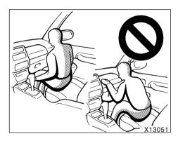
• Do not sit on the edge of the seat or lean over the dashboard when the vehicle is in use. The airbags inflate with considerable speed and force; you may be killed or seriously injured. Sit up straight and well back in the seat, and always use your seat belt.
