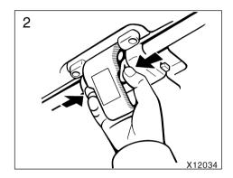
2. Push in the retaining spring arms as shown and push up the sun roof.
