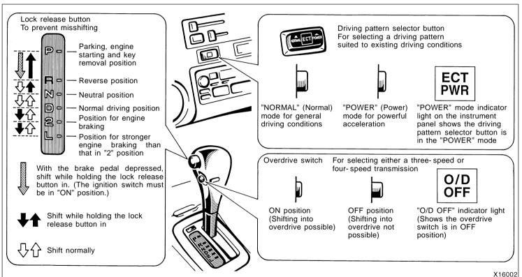
Vehicles with cruise control—When the cruise control is being used, even if you downshift the transmission by turning off the overdrive switch, engine braking will not be applied because the cruise control is not cancelled. For ways to decrease the vehicle speed, see "Cruise control" in this chapter.
