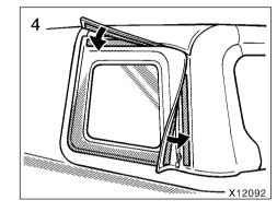
4. Fasten the zipper securely and align the Velcros to secure the quarter windows.
