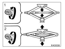
To remove the jack, move the seat to the front-most position and turn the jack joint by hand.
