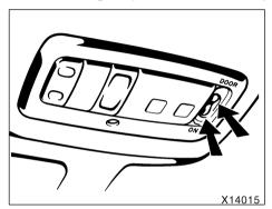
To turn on the personal light, push the switch. To turn the light off, slightly push the switch on the opposite side.
