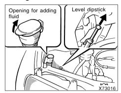
Check the washer fluid level in the reservoir with the dipstick. If the washer fluid level is low, reinsert the dipstick securely and add washer fluid through the opening for adding fluid.
