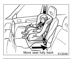
• A forward-facing child restraint system should be allowed to put on the front seat only when it is unavoidable. Always move the seat as far back as possible because the force of a deploying airbag could cause death or serious injury to the child. For instructions concerning the installation of a child restraint system, see "Child restraint" in this chapter.
