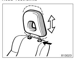
For your safety and comfort, adjust the head restraint before driving.
