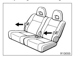
Lean forward and pull the lock release lever. Then lean back to the desired angle and release the lever.
