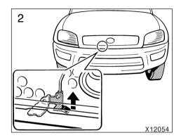
In front of the vehicle, pull up the auxiliary catch lever and lift the hood.
