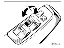
Automatic operation: Push the switch completely down or pull it completely up, and then release it. The window will fully open or close. To stop the window partway, lightly move the switch in the opposite direction and then release it.
