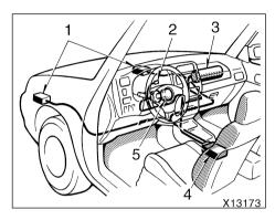
The SRS airbag system mainly consists of the following components and their locations are shown in the illustration.
