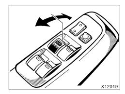
The windows can be operated with the switch on each side door.
