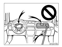
• Do not put objects or your pets on or in front of the dashboard or steering wheel pad that houses the airbag system. They might restrict inflation or cause death or serious injury as they are projected rearward by the force of the deploying airbags. Likewise, the driver and front passenger should not hold things in their arms or on their knees.
