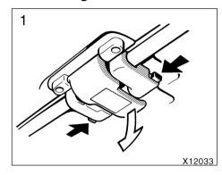
1. Pull the handle down while pushing in one of the lock buttons.
