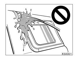
Soft-top models: Spray water on the quarter windows, rear window or top seals from above, at a 45° angle to the ground.
