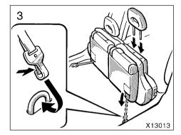
3. Lock the raised bottom cushion in place by clipping the strap to the hook. Then store the head restraint in the head restraint retaining holes in the bottom cushion.
