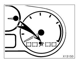
This SRS airbag system has a service reminder indicator to inform the driver of operating problems. If either of the following conditions occurs, this indicates a malfunction of the airbags. Contact your Toyota dealer as soon as possible to service the vehicle.
