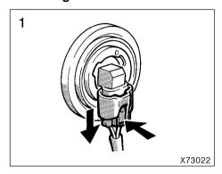
Open the hood. Unplug the connector while depressing the lock release.
