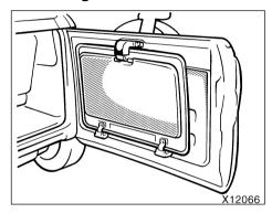
Install the removed sun roof panel on the tailgate as follows.
