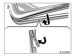
3. Insert the retainer on the bottom of the window into the groove.
