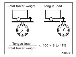
The trailer cargo load should be distributed so that the tongue load is 9 to 11% of the total trailer weight, not exceeding 68 kg (150 lb.).
