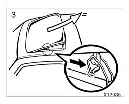
3. Push back the auxiliary catch to release it from the hook. Then lift the sun roof panel and pull it out.
