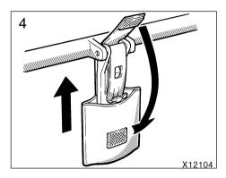
Take the latch handle cover out of the glove box, put it over the latch handle and fasten it securely with Velcros.
