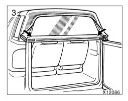
Fasten the zippers securely and align the Velcros to secure the rear window.
