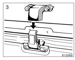
3. Place the removed holder over the sun roof handle.
