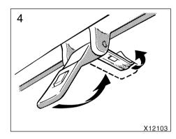
4. Set the hook, push up the latch handle to securely lock it.
