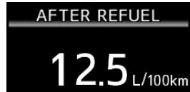
Displays the average fuel consumption since the vehicle was last refueled
