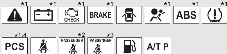
\*<sup>1</sup>: These lights turn on when the “ENGINE START STOP” switch is turned to IGNITION ON mode to indicate that a system check is being performed. They will turn off after the engine is started, or after a few seconds. There may be a malfunction in a system if the lights do not come on, or if the lights do not turn off. Have the vehicle inspected by your Toyota dealer.
