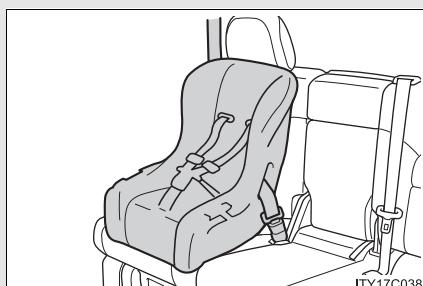
Seat belts equipped with a child restraint locking mechanism (ALR/ELR belts except driver's seat belt) (→P. 70)
