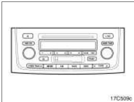
**AM-FM radio/cassette player/compact disc changer controller/compact disc player with changer (with XM satellite radio\* controller)**
