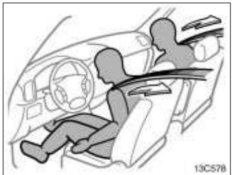
The driver and front passenger seat belt pretensioners are designed to be activated in response to a severe frontal impact or a vehicle rollover.
