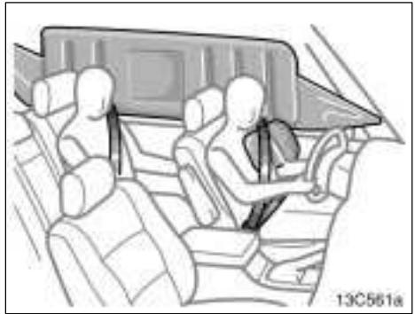
The SRS (Supplemental Restraint System) side airbags and curtain shield airbags are designed to provide further protection for the driver, front passenger and second seat passengers in addition to the primary safety protection provided by the seat belts.
