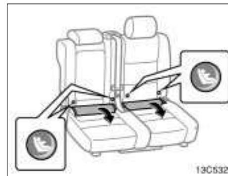
2. Take off the cover between the seat cushion and seatback and confirm the position of the lower anchorages below the symbol in the seat back.
