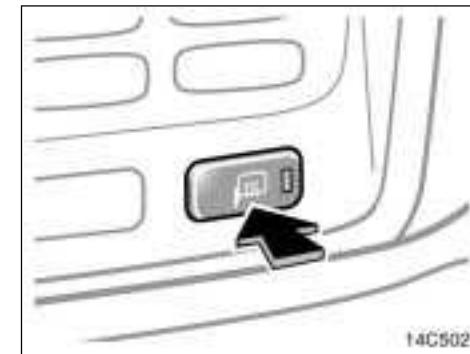
**To defog or defrost the outside rear view mirrors, push the switch.**
