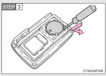
Remove the depleted battery.
