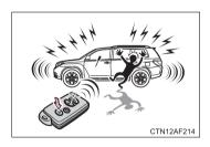
When (i) is pushed for longer than about one second, an alarm will sound for about 60 seconds and the vehicle lights will flash to deter any person from trying to break into or damage your vehicle.
