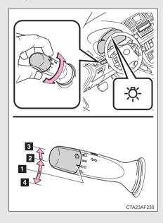
1 AUTO The headlights and parking lights turn on and off automatically. (Vehicles without smart key system: When the engine switch is turned to the "ON" position. Vehicles with smart
