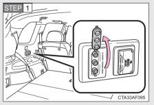
Open the cover, and connect the audio source to the A/V input port.
