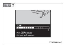
Press the "DISP" button on the steering wheel to adjust the tone.
