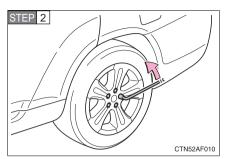
Slightly loosen the wheel nuts (one turn).
