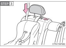
Adjust the head restraint to the downmost position.
