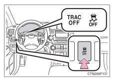
Push and hold the button while the vehicle is stopped to turn off TRAC and VSC.
