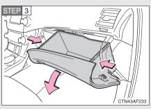
Push each side of the glove box to release the pins. Then pull the glove box down toward you.
