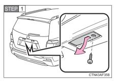
Remove the screw and remove the unit.
