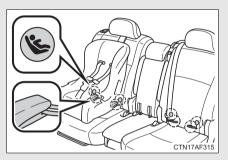
Second seat: Child restraint LATCH anchors
