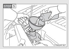
Add engine coolant if necessary.
