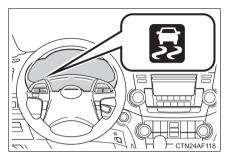
If the vehicle is in danger of slipping, rolling backwards when starting on an incline, or the front wheels (2WD models) or four wheels (4WD models) spin, the indicator flashes to indicate that the VSC/TRAC systems have been engaged.
