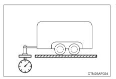
The load placed on the trailer hitch ball. ( $\rightarrow$ P. 257)
