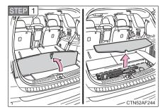
Open the center deck board and remove the cover.
