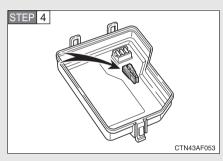
Remove the fuse with the pullout tool.
