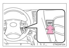
Push the "DISP" button on the steering wheel to display trip information.
