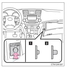
Turn the main switch in the glove box off to disable the power back door system.
