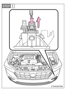
Unplug the connector while depressing the lock release.
