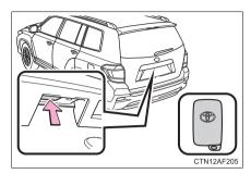
Press the button to unlock the door.
