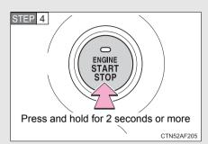
Vehicles with a smart key system: Stop the engine by pressing and holding the "ENGINE START STOP" switch for 2 consecutive seconds or more.
