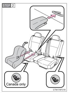
Latch the buckles onto the LATCH anchors.
