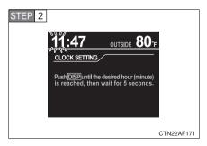
Press the "DISP" button on the steering wheel to adjust the hours.
