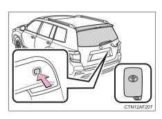
Press and hold the button to open the glass hatch. The glass hatch will pop up.
