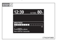
Press the "DISP" button on the steering wheel to adjust the brightness.
