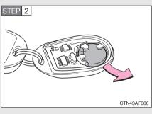
Remove the discharged transmitter battery.
