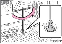
Connect the jack handle and the adapter socket. Turn the jack handle.
