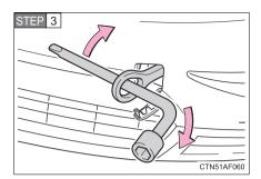
Tighten down the towing eyelet using a wheel securely wrench.
