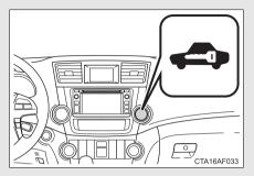
Vehicles without smart key system: The indicator light flashes after the key has been removed from the engine switch to indicate that the system is operating.
