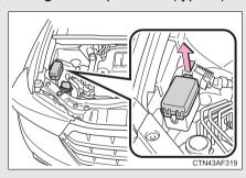
Push the tab in and lift the fuse box cover off. (if equipped)
