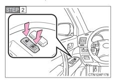
Shift the shift lever to P or N, and press and hold the driver's door lock switch ( or or approximately 5 seconds and then release it.
