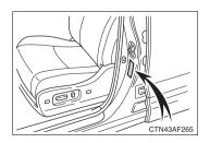
For the GAWR, see the Certification Label. For the maximum load of the tire, see the load limit at maximum cold tire inflation pressure mentioned on the sidewall of the tire. ( $\rightarrow$ P. 636)
