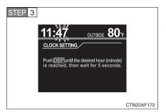
Press the "DISP" button on the steering wheel to adjust the minutes.
