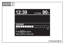
Press the "DISP" button on the steering wheel to adjust the contrast.
