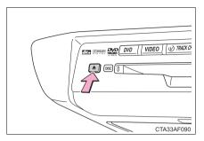
Press (a) and remove the disc.
