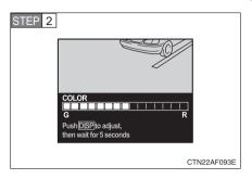
Press the "DISP" button on the steering wheel to adjust the color.
