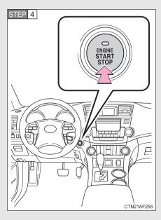
Press the "ENGINE START STOP" switch.
