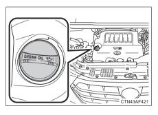
If the oil level is below or near the low level mark, add engine oil of the same type as that already in the engine. Make sure to check the oil type and prepare the items needed before adding oil.
