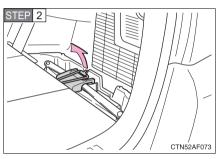
Unhook the tightening strap and remove the pad.
