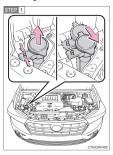
Right side only: Move the washer fluid tank opening.
