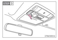
Press and hold down one of the buttons on the HomeLink<sup>®</sup> and the button on the transmitter. When the indicator light on the HomeLink<sup>®</sup> changes from a slow to a rapid flash within 20 seconds, you can release both buttons.
