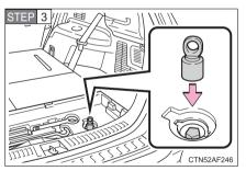
Attach the adapter socket (for removing a spare tire) to the spare tire clamp bolt.
