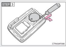
Remove the depleted battery.
