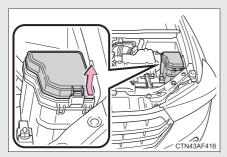
Push the tab in and lift the fuse box cover off.
