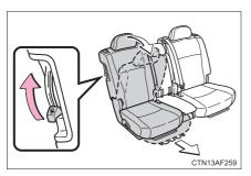
Lift the lever on the side of the seatback and fold down the seatback. The seat will slide forward.
