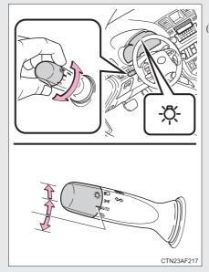
Auto The headlights and (if equipped) parking lights turn on and off automatically. (Vehicles without smart key system:
