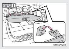
Hang the hooks on the hook brackets on the second seat seatback.
