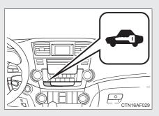
Vehicles without smart key system: The indicator light flashes after the key has been removed from the engine switch to indicate that the system is operating.
