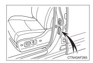
For the GAWR, see the Certification Label. For the maximum load of the tire, see the load limit at maximum cold tire inflation pressure mentioned on the sidewall of the tire. ( $\rightarrow$ P. 590)
