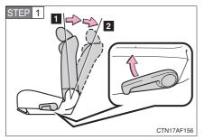
Fold the seatback while pulling the lever. Return the seatback and secure it at the 1st lock position (most upright position). Adjust the seatback to the 3rd lock position.  $(\rightarrow P. 77)$
