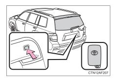
Press and hold the button to open the glass hatch. The glass hatch will pop up.
