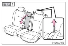
Fold down the second center seatback while pulling the seat-back lock release strap.
