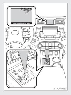
The rear view image is displayed when the shift lever is in the R position.
