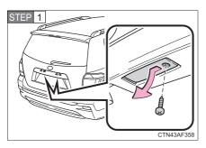
Remove the screw and remove the unit.
