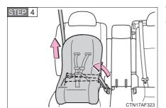
While pushing the child seat into the rear seat, allow the shoulder belt to retract until the child seat is securely in place.
