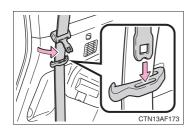
Pass the outer seat belts through the seat belt hangers and secure the seat belt plates to prevent the shoulder belts from being damaged.
