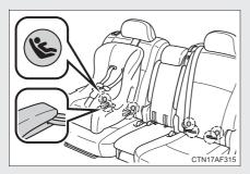
Second seat: Child restraint LATCH anchors
