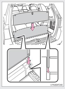
The center deck board can be used to separate the luggage compartment.
