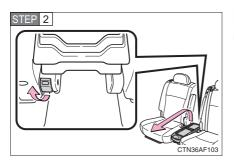
Pull the lock release lever to remove the side table.
