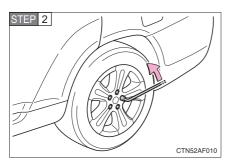
Slightly loosen the wheel nuts (one turn).
