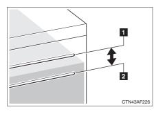
Check that the level is between "UPPER"/"MAX" and "LOWER"/
