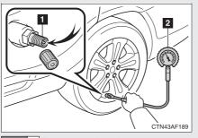
STEP 1 Remove the tire valve cap.
