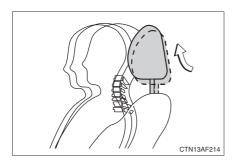
When the occupant's lower back presses against the seatback during a rear-end collision, the head restraint moves slightly forward and upward to help reduce the risk of whiplash to the seat occupant.
