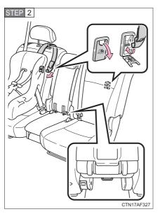
Outer seat: Open the anchor bracket cover, latch the hook onto the anchor bracket and tighten the top tether strap.
