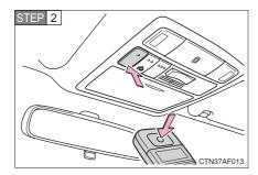
Press and hold down one of the buttons on the HomeLink<sup>®</sup> and the button on the transmitter. When the indicator light on the HomeLink<sup>®</sup> changes from a slow to a rapid flash within 20 seconds, you can release both buttons.
