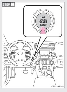
Press the "ENGINE START STOP" switch.
