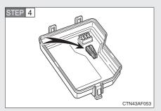
Remove the fuse with the pullout tool.
