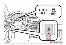
Push and hold the button while the vehicle is stopped to turn off TRAC and Enhanced VSC.
