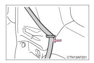
Pass the outer seat belts through the seat belt hangers to help prevent the shoulder belts from being damaged.
