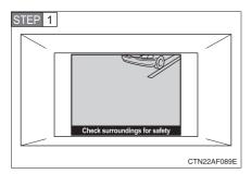
Display the set up screen on the multi-information display when the vehicle is stopped and the rear view monitor is turned on.
