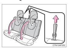
While pulling the straps, fold down the seatbacks.
