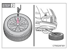
Put the flat tire on the ground with the outer side facing up and install the holding bracket.
