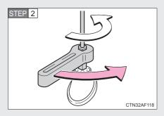
Loosen the antenna with the wrench and remove it.
