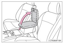
Pull up the knob to release the lock. Lift the lid.
