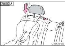
Adjust the head restraint to the downmost position.
