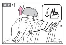
Secure the child restraint using the seat belt or lower anchors, and adjust the head restraint to the upmost position.
