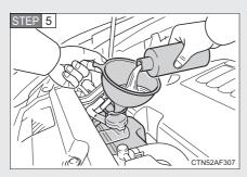
Add engine coolant if necessary.
