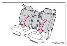
Pull the lever to unlock the seatback and then fold the seatback down.
