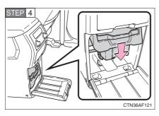
Push down on the end to engage the pins in the holes and close the console box door.
