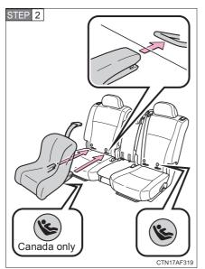
Latch the buckles onto the LATCH anchors.
