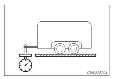
The load placed on the trailer hitch ball.  $(\rightarrow P. 252)$
