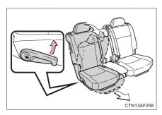
Pull up the lever and fold down the seatback. The seat will slide forward.
