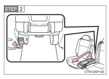
Pull the lock release lever to remove the second center seat.
