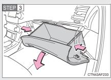
Push each side of the glove box to release the pins. Then pull the glove box down toward you.
