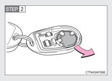
Remove the discharged transmitter battery.
