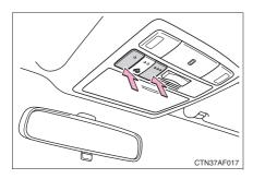
Press and hold down the 2 outside buttons for 10 seconds (or 20 seconds depending on the model) until the indicator light flashes.
