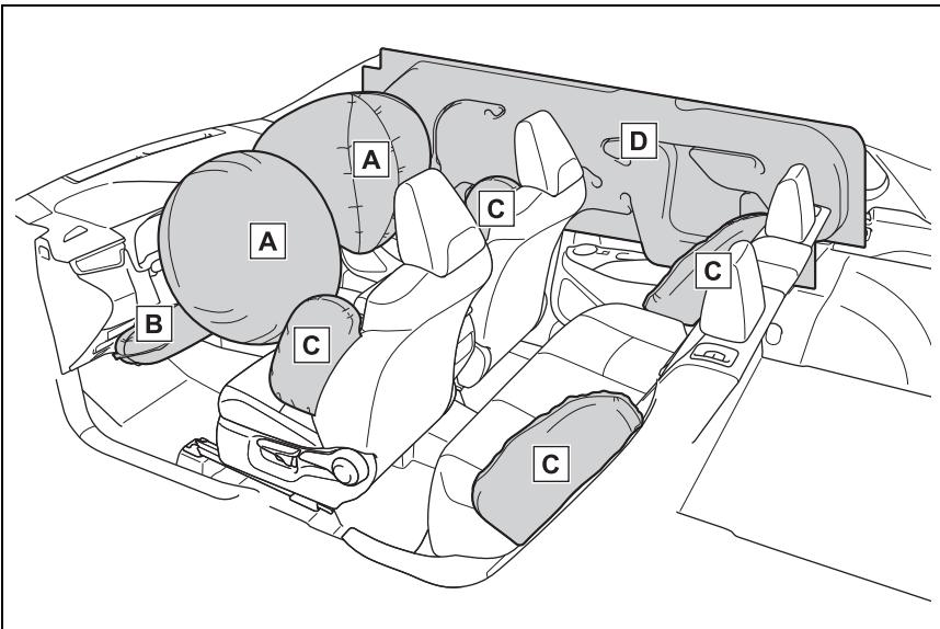
**A** SRS front airbags (SRS driver airbag/SRS front passenger airbag)
