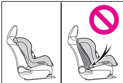
\*<sup>3</sup>: If the head restraint interferes with your child restraint system, and the head restraint can be removed, remove the head restraint.
