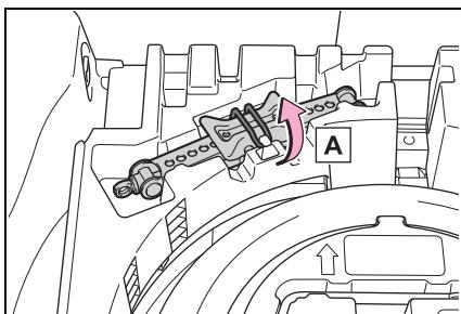
**A** Disengage the tightening strap.
