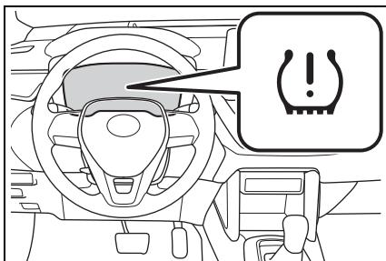
9 If the specified tire inflation pressure of the wheel set installed differs from that of the previous set, it will be necessary to perform the tire inflation pressure setting procedure of the tire pressure warning system. (→P.367)
