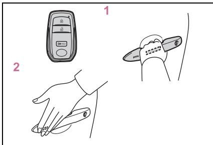
1 Grip the driver's door handle to unlock the door. Holding the driver's door handle for approximately 2 seconds unlocks all the doors. Grip the front passenger's door handle to unlock all the doors.\*
