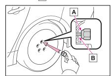
When replacing an aluminum wheel with a steel wheel (including a compact spare tire), tighten the wheel nuts until the tapered portion A comes into loose contact with the
