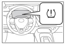
9 If the specified tire inflation pressure of the wheel set installed differs from that of the previous set, it will be necessary to perform the tire inflation pressure setting procedure of the tire pressure warning system. (→P.318)
