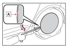
Slightly loosen the wheel nuts (one turn).
