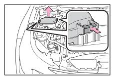
Engine compartment: type B fuse box
