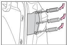
Pull the cover toward the rear of the vehicle and remove the cover.
