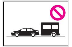
Your vehicle is not designed to be dinghy towed (with 4 wheels on the ground) behind a motor home.
