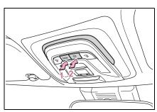
1 Turns the door position on/off When a door is opened while the door position is on, the lights turn
