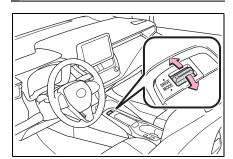
Operate the driving mode select switch forward or backward to select the desired driving mode on the multi-information display.
