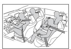
The pretensioners help the seat belts to quickly restrain the occupants by retracting the seat belts when the vehicle is subjected to certain types of severe frontal or side collision or a vehicle rollover.
