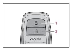
1 Locks all the doors Check that the door is securely locked.
