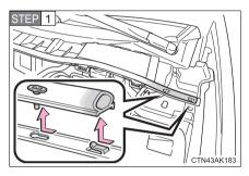
Slide and lift up the rubber strip to partly remove it as shown.
