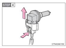
Unplug the bulb while depressing the lock release.
