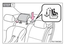
Secure the child restraint using a seat belt or the lower anchors, and lock the head restraint in place at the lowest position.
