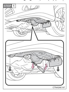
Remove the fender liner bolts and clip.
