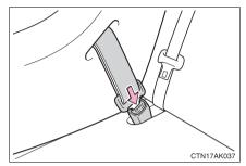
Push the release button and fully retract the seat belt.
