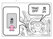
Push and hold the switch while the vehicle is stopped to turn off TRAC and VSC.
