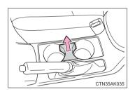
The cup holder insert may be removed for cleaning.
