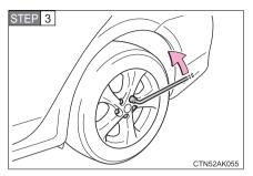
Slightly loosen the wheel nuts (one turn).
