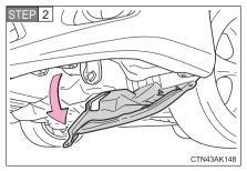
Partly remove the fender liner.
