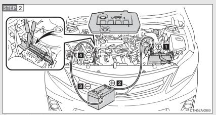
Connecting the jumper cables
