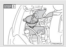
Add engine coolant if necessary.
