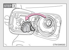
Hang the fuel tank cap on the back of the fuel filler door.
