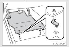
Fix the floor mat in place using the retaining hooks (clips) provided.
