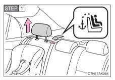
Secure the child restraint using a seat belt or the lower anchors, and remove the head restraint.
