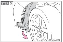
Partly remove the fender liner.
