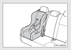
Seat belts equipped with a child restraint locking mechanism (ALR/ELR belts except driver's seat belt) (→P. 58)
