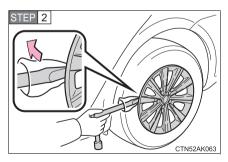
Vehicles with a steel wheel, remove the wheel ornament using the wrench.
