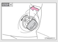
Vehicles without a smart key system: Stop the engine by turning the engine switch to the "ACC" position.
