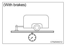
The maximum allowable gross trailer weight. The gross trailer weight is the sum of the trailer weight and the weight of the cargo in the trailer.
