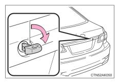
Turn the mechanical key ( $\rightarrow$ P. 23) clockwise to open.
