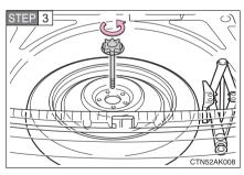
Loosen the center fastener that secures the spare tire.
