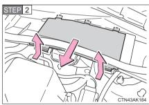
Disconnect the claws and remove the service cover.
