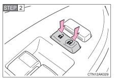
Shift the shift lever to P or N, and press and hold the driver's door lock switch ( or or ) for approximately 5 seconds and then release.
