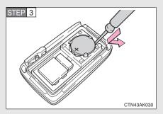
Remove the depleted battery.
