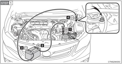
Connecting the jumper cables
