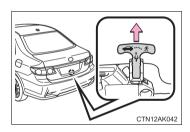
The trunk lid can be opened by pulling down on the glow-in-the-dark lever located on the inside of the trunk lid.
