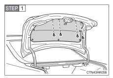
Open the trunk lid and remove the trunk panel cover clips.
