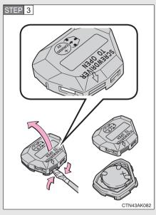
Open the case cover using a flathead screwdriver protected with tape etc. and remove the depleted battery.
