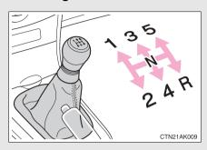
Fully depress the clutch pedal before operating the shift lever, and then release the clutch pedal slowly.
