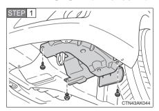
Remove the fender liner bolts and clip.
