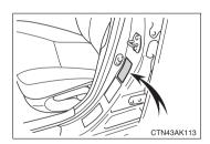
For the GAWR, see the Certification Label. For the maximum load of the tire, see the load limit at maximum cold tire inflation pressure mentioned on the sidewall of the tire. ( $\rightarrow$ P. 440)
