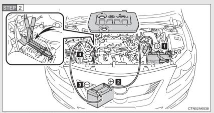
Connecting the jumper cables
