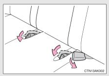
Stow the rear outside seat belt buckles and move the rear center seat belt buckle as shown.
