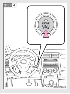
Press the "ENGINE START STOP" switch.
