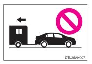
Do not tow the vehicle backwards. Doing so may cause serious damage.
