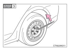
Slightly loosen the wheel nuts (one turn).
