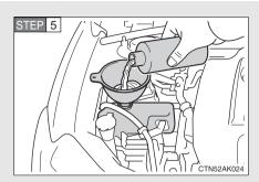
Add engine coolant if necessary.
