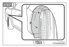
Remove the fender liner clips.
