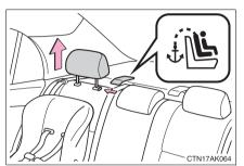
Remove the head restraint.
