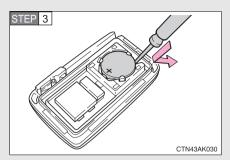
Remove the depleted battery.
