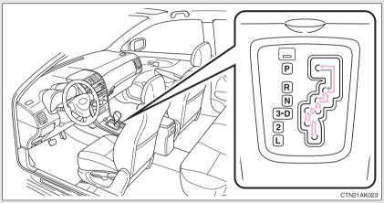
Vehicles with smart key system: While the "ENGINE START STOP" switch is in IGNITION ON mode, depress the brake pedal and move the shift lever.
