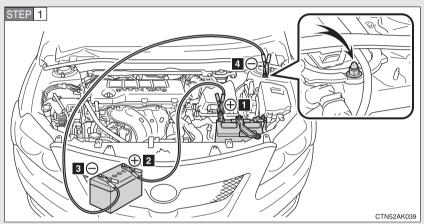
Connecting the jumper cables
