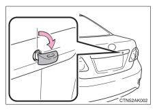
Turn the mechanical key ( $\rightarrow$ P. 21) clockwise to open.
