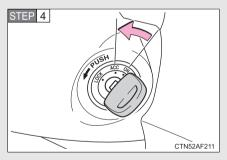
Vehicles without a smart key system: Stop the engine by turning the engine switch to "ACC".
