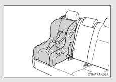
Seat belts equipped with a child restraint locking mechanism (ALR/ELR belts except driver's seat belt) (→P. 55)
