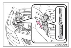
Check the washer fluid level on the level gauge. If the washer fluid level is at "LOW". add washer fluid.
