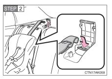
Open the anchor bracket cover, latch the hook onto the anchor bracket and tighten the top tether strap.
