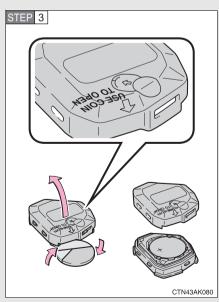
Open the case cover using a coin protected with tape etc. and remove the depleted battery.
