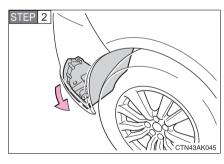
Partly remove the fender liner.
