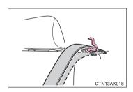
Use the seat belt after passing it through the guide if the seat belt comes free from the guide.
