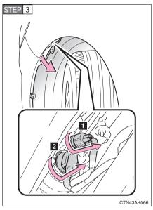
Partly remove the fender liner and turn the bulb base counterclockwise.
