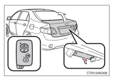
Press the button to unlock the trunk.
