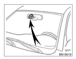
The compass sensor is on the inside rear view mirror.
