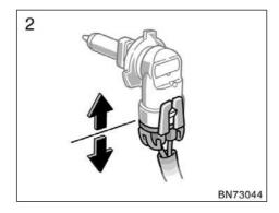
2. Pull the bulb out of the base. Install a new bulb.
