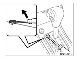
If you cannot shift the selector lever out of "P" position to other positions even though the brake pedal is depressed, use the shift lock override button as follows:
