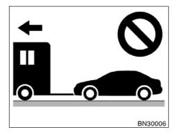
Your vehicle is not designed to be dinghy towed (with four wheels on the ground) behind a motorhome.
