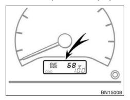
The displayed temperature ranges from -30°C (-22°F) up to 50°C (122°F).
