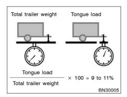
• The trailer cargo load should be distributed so that the tongue load is 9 to 11% of the total trailer weight, not exceeding the maximum of 68 kg (150 lb.). Never load the trailer with more weight in the back than in the front. About 60% of the trailer load should be in the front half of the trailer and the remaining 40% in the rear.
