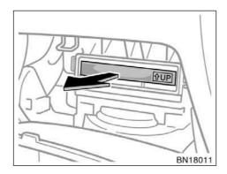
4. Pull the filter out of the filter outlet. Inspect the filter on the surface.
