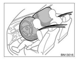
The SRS (Supplemental Restraint System) front airbags are designed to provide further protection for the driver and front passenger in addition to the primary safety protection provided by the seat belts.
