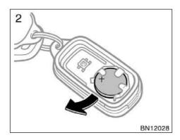
2. Remove the discharged transmitter battery.
