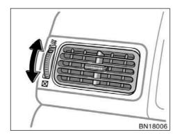
If air flow control is not satisfactory, check the side vents. The side vents may be opened or closed as shown.
