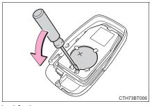
Insert a new battery with the "+" terminal facing up.
