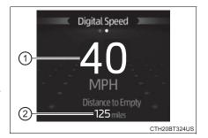
This distance is computed based on your average fuel consumption. As a result, the actual distance that can be driven may differ from that displayed.
