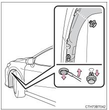
To protect the front bumper from being damaged, apply protective tape around the clip as shown in the illustration.
