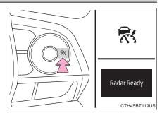
If the cruise control main switch is pressed and held for 1.5 seconds or more, the system turns on in constant speed control mode. (→P. 317)
