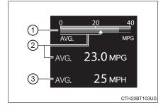
Displays the average vehicle speed since reset or elapsed time since reset, as selected in . (→P. 103)
