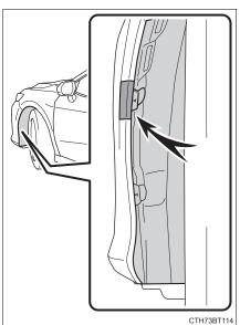
Insert a small flathead screwdriver between the front bumper and fender liner at the position marked with a "V" and then separate the front bumper from the fender liner.
