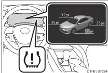
When replacing the tires or wheels, the tire pressure warning valve and transmitters must be installed to the wheels which will be installed to the vehicle.
