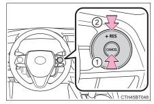
2 Pressing the "+ RES" switch resumes the cruise control and returns vehicle speed to the set speed. When your vehicle is too close to a vehicle ahead, and sufficient automatic deceleration via the cruise control is not possible, the display will flash and the buzzer will sound to alert the driver. An example of this would be if another driver cuts in front of you while you are following a vehicle. Depress the brake pedal to ensure an appropriate vehicle-to-vehicle distance.
