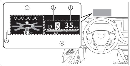
Driving assist system status/navigation system-linked display area (if equipped) (→P. 130)
