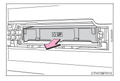
The "↑UP" marks shown on the filter and the filter case should be pointing up.
