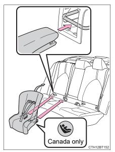
4 If the child restraint has a top tether strap, follow the child restraint manufacturer's operation manual regarding the installation, using the top tether strap to latch onto the top tether strap anchor. (→P. 72)
