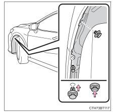
9 To Install the fender liner to the front bumper, engage the clip to the front bumper.
