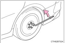
To prevent damage to the vehicle when using the jack, position the jack in the correct location.  $(\rightarrow P. 545)$
