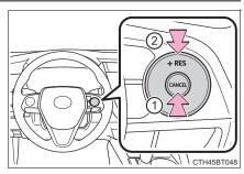
However, cruise control does not resume when the vehicle speed is approximately 16 mph (25 km/h) or less.
