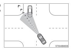
When you turn right/left, pedestrian is detected in the forward direction and estimated to enter your vehicle's path (bicyclists are detected.)
