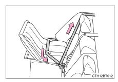
5 After installing the child restraint system, rock it back and forth to ensure that it is installed securely. (→P. 68)
