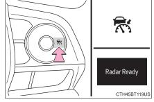
If the cruise control main switch is pressed and held for 1.5 seconds or more, the system turns on in constant speed control mode. (→P. 301)
