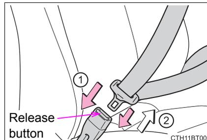
**Adjusting the seat belt shoulder anchor height (front seats)**
