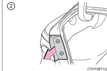
To prevent scratching the vehicle, wrap the tip of the flathead screwdriver with a cloth, etc.
