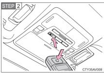
Press and hold one of the HomeLink® buttons and the transmitter button. When the HomeLink® indicator light changes from a slow to a rapid flash, you can release both buttons.
