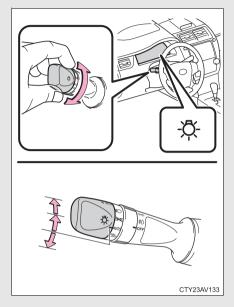
AUTO Vehicles without a smart key system: The headlights and parking lights, daytime running lights turn on and off automatically (when the engine switch is in the "ON" position).
