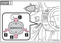
To adjust the mirror, press the switch.
