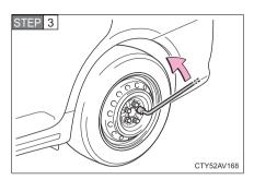
Slightly loosen the wheel nuts (one turn).
