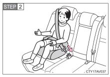
Sit the child in the child restraint system. Fit the seat belt to the child restraint system according to the manufacturer's instructions and insert the plate into the buckle. Make sure that the belt is not twisted.
