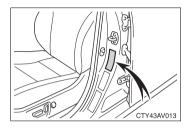
For the GAWR, see the Certification Label. For the maximum load of the tire, see the load limit at maximum cold tire inflation pressure mentioned on the sidewall of the tire.  $(\rightarrow P. 489)$
