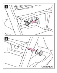
The auxiliary box of the front console is provided with a hole that allows cables to be passed into the cabin from the power outlet and AUX port or AUX port/USB port inside.
