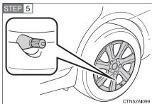
For vehicles with a steel wheel, reinstall the wheel ornament.
