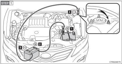
Connecting the jumper cables
