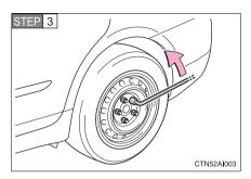
Slightly loosen the wheel nuts (one turn).
