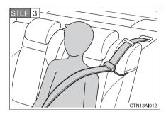
Buckle, position and release the seat belt.
