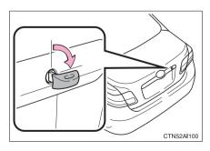
Turn the mechanical key clockwise to open.
