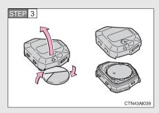
Open the case cover using a coin protected with tape etc. and remove the depleted batterv.
