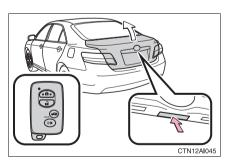
Press the button to unlock the trunk.
