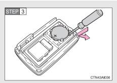
Remove the depleted battery.
