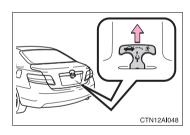
The trunk lid can be opened by pulling up the glow-in-the-dark lever located on the inside of trunk lid.
