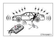
When ((1) is pressed for longer than about one second, an alarm will sound intermittently and the vehicle lights will flash to deter any person from trying to break into or damage your vehicle.
