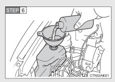
Add engine coolant if necessary.
