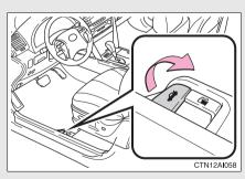
Pull the lever to release the trunk lid.
