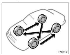
To equalize the wear and help extend tire life, Toyota recommends that you rotate your tires approximately every 12000 km (7500 miles). However, the most appropriate timing for tire rotation may vary according to your driving habits and road surface conditions.
