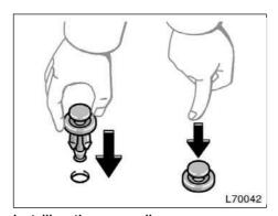
Installing the cover clips
