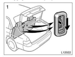
This system deactivates the lock release lever so that things locked in the trunk can be protected.
