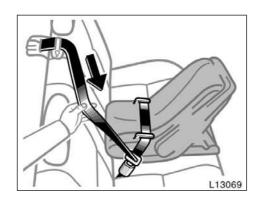
Fully extend the shoulder belt to put it in the lock mode. When the belt is then retracted even slightly, it cannot be extended.
