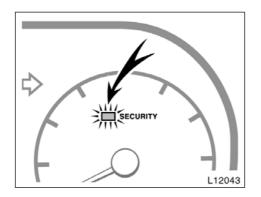
The system is automatically set when the key is removed from the ignition switch. The indicator light will start flashing every 1 second to show the system is set.
