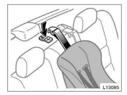
If your child restraint system requires the use of a top strap, latch the hook onto the anchor bracket and tighten the top strap.
