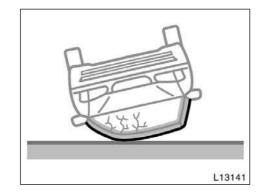
The SRS side airbags are not designed to inflate if the vehicle is rolled over.
