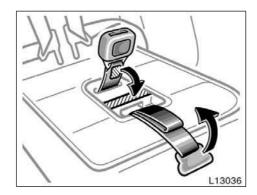
11. To store the built-in child restraint, fasten the shoulder belt clip and return the seat belt buckle using the fastener tapes. Fold up the seat belt adjustment strap (gray tab) in the seat so that the edge of the strap does not come out the raised seat cushion. Raise the seat cushion and reinstall the head restraint and upper pad by inserting the posts into the holes.
