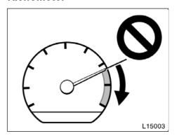
The tachometer indicates engine speed in thousands of rpm (revolutions per minute). Use it while driving to select correct shift points and to prevent engine lugging and overrevving.
