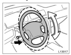
To change the steering wheel angle, hold the steering wheel, pull the lock release lever, tilt the steering wheel to the desired angle and release the lever.
