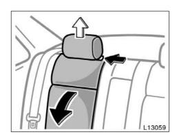
Remove the head restraint and upper pad by pressing the head restraint lock release button and pulling up the head restraint and upper pad. Lower the child seat cushion.
