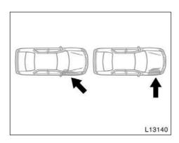
The SRS side airbag system may not inflate if the vehicle is subjected to a collision from the side at an angle, or a collision to the side of the vehicle body other than the passenger compartment shown in the illustration, which impact is not severe enough for the passenger compartment.
