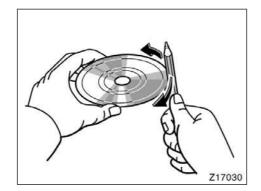
A new disc may have rough edges on its inner and outer perimeter. Remove the rough edges by pressing the side of a ball-point pen or pencil against the inner and outer perimeter of the disc as shown.
