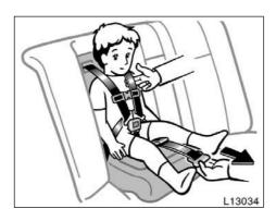
Pull the seat belt adjustment strap (gray tab) firmly until the shoulder belts are snugly adjusted around the child's shoulders.
