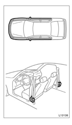
This front seat belt pretensioner system has a service reminder indicator to inform the driver of operating problems. If either of the following conditions occurs, this indicates a malfunction of the airbags or pretensioners. Contact your Toyota dealer as soon as possible to service the vehicle.
