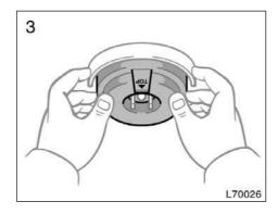
3. Install the rubber cover with the "TOP" mark upward, and snuggle on the boss. Insert the connector. Then install the plastic cover.
