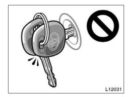
♦When starting the engine, do not use the key in contact with another transponder key (including keys of other vehicles) and do not press another key plate against the key grip. Otherwise the engine may not start, or may stop soon after it starts.
