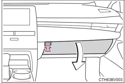
The glove box light turns on when the engine switch is in ACCESSORY or IGNITION ON mode.
