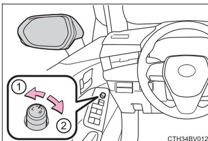
2 To adjust the mirror, operate the switch.
