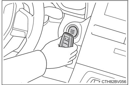
3 Firmly depress the brake pedal and check that
