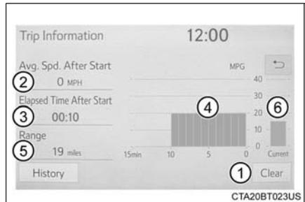
Average fuel consumption for the past 15 minutes is divided by color into past averages and averages attained since the engine switch was last turned to IGNITION ON mode. Use the displayed average fuel consumption as a reference.
