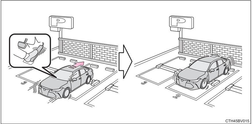
**◆ When the vehicle moves in the unintended direction due to the wrong shift position being selected**
