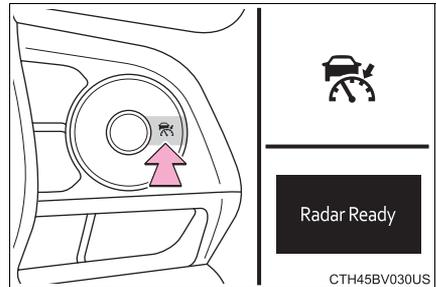
If the cruise control main switch is pressed and held for 1.5 seconds or more, the system turns on in constant speed control mode. (→P. 274)
