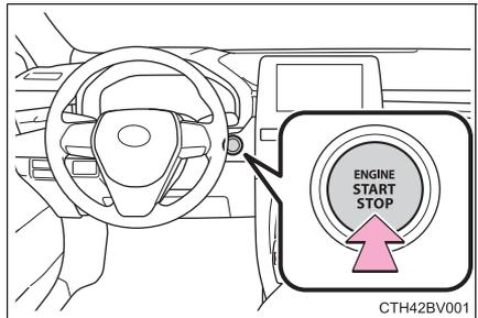
Continue depressing the brake pedal until the engine is completely started. The engine can be started from any engine switch mode.
