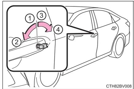
Turning the key rearward unlocks the driver's door. Turning the key once again unlocks the other doors.
