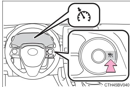
2 Accelerate or decelerate, with accelerator pedal operation, to the desired vehicle speed (at or above approximately 25 mph [40 km/h]) and press the “- SET” switch to set the speed.
