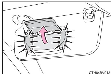
If the vanity lights remain on for 20 minutes while the engine is off, the lights will turn off automatically.
