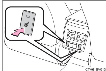
The seat heaters can be used when the engine switch is in IGNITION ON mode.
