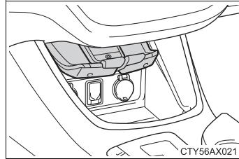
An electronic device on the tray can be recharged by running a charging cable through the clearance of the tray and connecting it to the AUX/USB port or power outlet underneath the tray.
