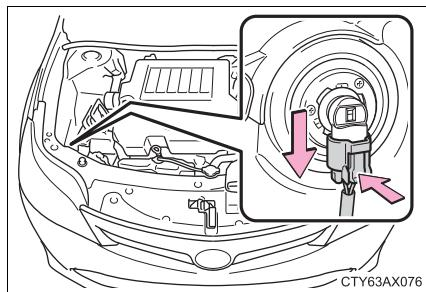
2 Turn the bulb base counter-clockwise.
