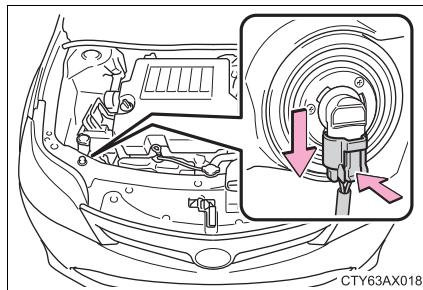
2 Turn the bulb base counter-clockwise.
