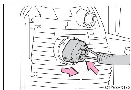
4 Turn the bulb base counter-clockwise.
