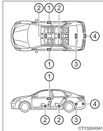
**■ Effective range (areas within which the electronic key is detected)****● When locking or unlocking the doors**
