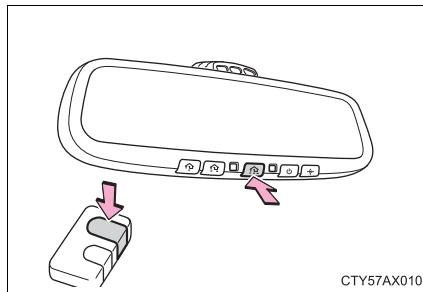
3 Test the operation of the HomeLink® by pressing the newly programmed button.
