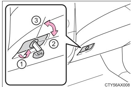
The trunk opener main switch is located in the glove box. (→P. 104)
