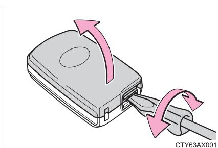
**3** Remove the depleted battery.
