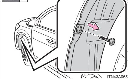
Remove the fender liner clip.
