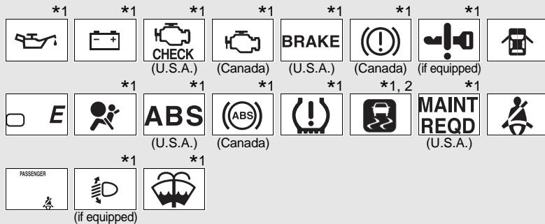
\*<sup>1</sup>: These lights turn on when the "ENGINE START STOP" switch is turned to IGNITION ON mode (vehicles with smart key system) or the engine switch is turned to the "ON" position (vehicles without smart key system) to indicate that a system check is being performed. They will turn off after the engine is started, or after a few seconds. There may be a malfunction in a system if the lights do not come on, or turn off. Have the vehicle inspected by your Toyota dealer.
