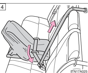
While pushing the child restraint system down into the rear seat, allow the shoulder belt to retract until the child seat is securely in place.
