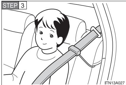
Buckle, position and release the seat belt.
