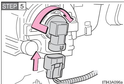
Turn and secure the socket and plug the connector.
