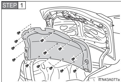
Open the trunk and remove the trunk panel cover.
