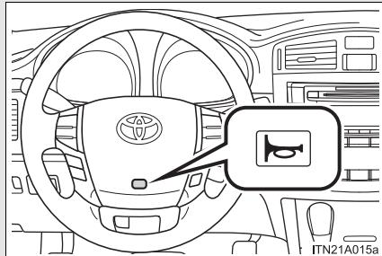
To sound the horn, press on or close to the
