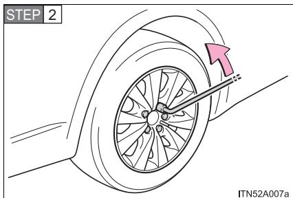
Slightly loosen the wheel nuts (one turn).
