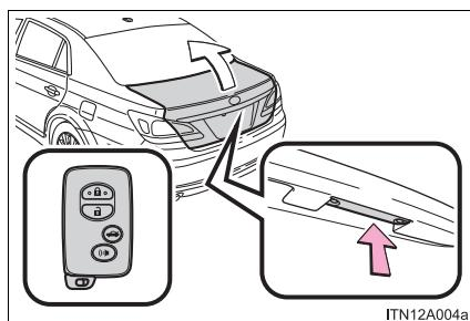
Press the button to unlock the trunk.
