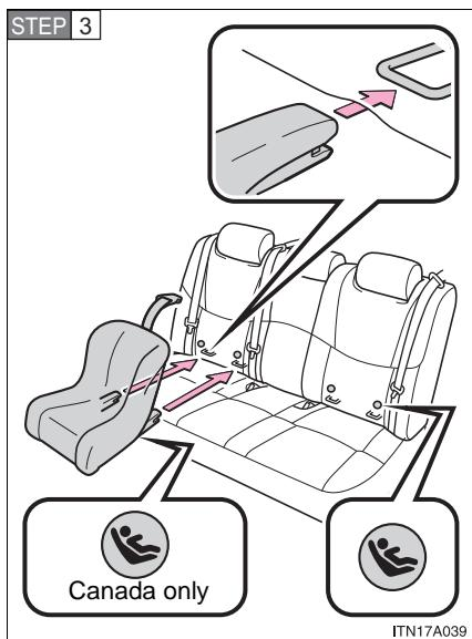
Latch the buckles onto the LATCH anchors.
