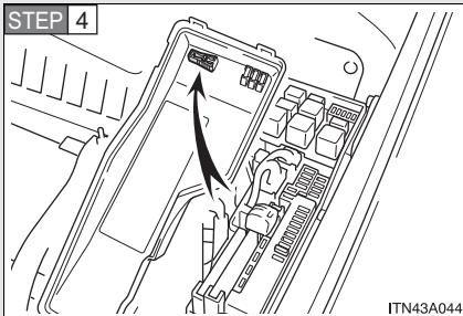
Remove the fuse with the pull-out tool.
