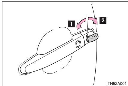
Using the mechanical key (→P. 28) in order to perform the following operations:
