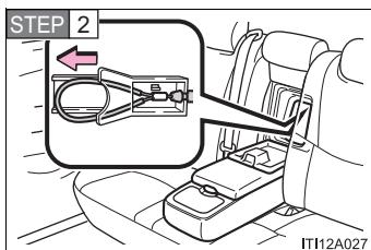
Pull the loop of wire to unlock the trunk lid.
