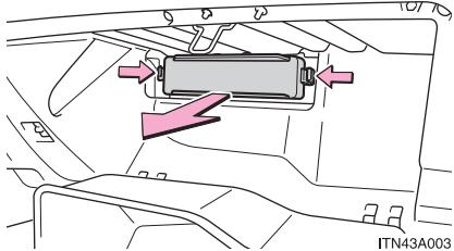
Remove the filter cover while pushing in both ends of the cover.
