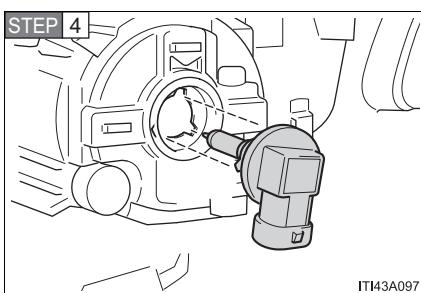
Exchange the light bulb, and install the socket.
