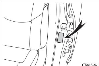
For the GAWR, see the Certification Label. For the maximum load of the tire, see the load limit at maximum cold tire inflation pressure mentioned on the sidewall of the tire. (→P. 532)
