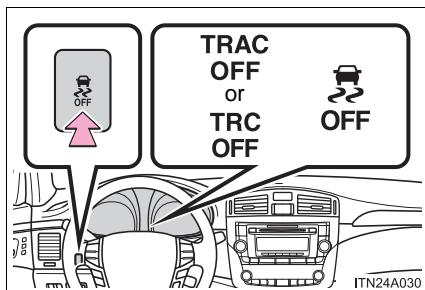
Push and hold the button for more than 3 seconds while the vehicle is stopped to turn off TRAC/TRC and VSC.
