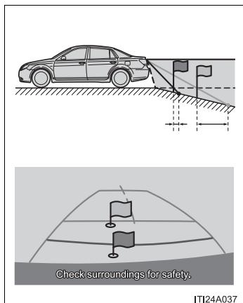
When the grade behind the vehicle slopes down sharply, objects appear to be closer than they actually are.
