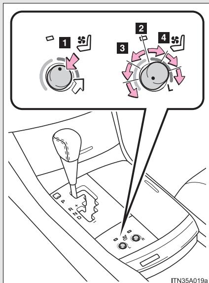
**1** Press the knob to release it, and turn the knob to the desired temperature setting.
