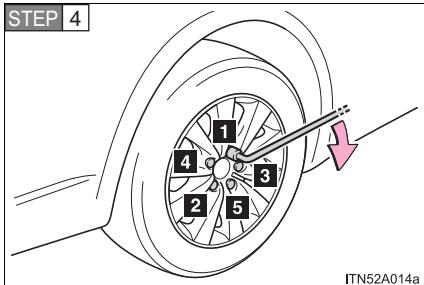
Firmly tighten each nut two or three times in the order shown in the illustration.
