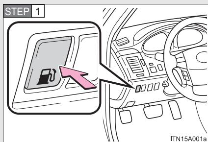
Press the fuel filler door opener switch.
