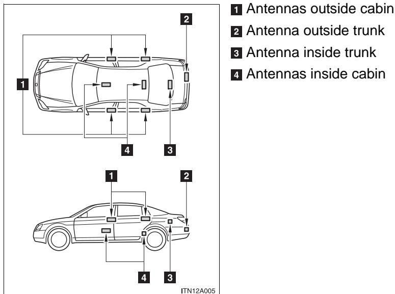
**■ Effective range (areas within which the electronic key is detected)**
