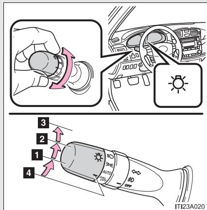
**■ AUTO** The headlights, parking lights, daytime running lights and so on turn on and off automatically. (When the “ENGINE START STOP” switch is in IGNITION ON mode [vehicles with smart key system] or the engine switch is in the “ON” position [vehicles without smart key system].)
