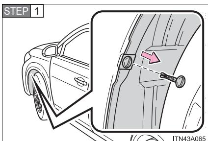
Remove the fender liner clip.
