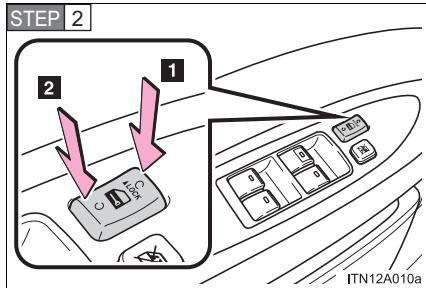
Shift the shift lever to “P” or “N”, press and hold the driver’s door lock switch (1 or 2) for about 5 seconds then release.
