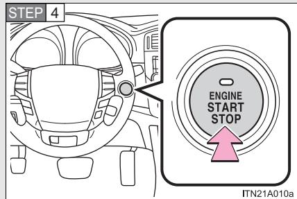
Press the “ENGINE START STOP” switch.
