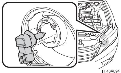
Exchange the light bulb, and install the socket.
