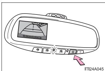
● To temporarily turn off the monitor when it is on.
