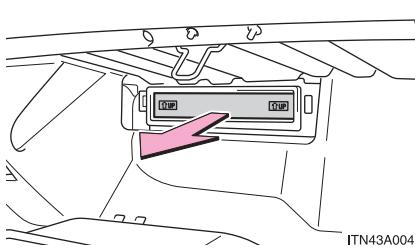
Pull the filter out of the filter outlet.
