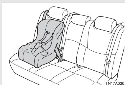
Seat belts equipped with a child restraint locking mechanism (ALR/ELR belts except driver's seat belt) (→P. 73)
