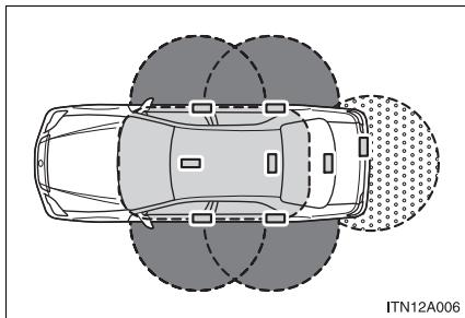
**● When locking or unlocking the doors**
