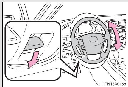
Hold the steering wheel, press the tilt lock release lever, and adjust to the ideal position by moving the steering wheel vertically.
