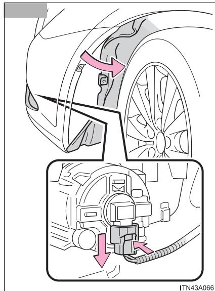
Partly remove the fender liner and unplug the connector while depressing the lock release.
