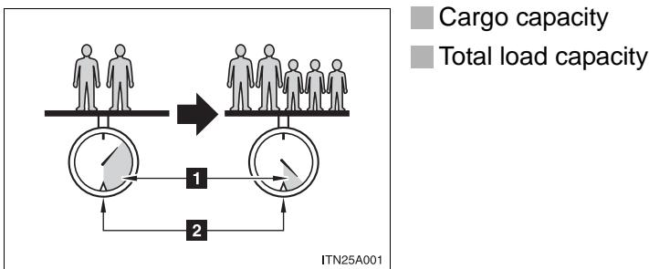
When 2 people with the combined weight of 366 lb. (166 kg) are riding in your vehicle, which has a total load capacity of 870 lb. (395 kg), the available amount of cargo and luggage load capacity will be as follows:
