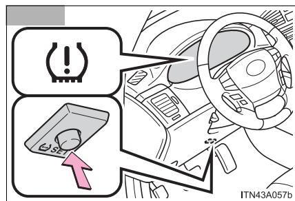
Push and hold the tire pressure warning reset switch until the tire pressure warning light blinks slowly 3 times.
