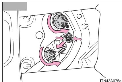
Turn the bulb bases counter-clockwise and remove (upper and lower), or squeeze bulb base and remove (center).
