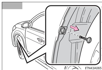
Remove the fender liner clip.
