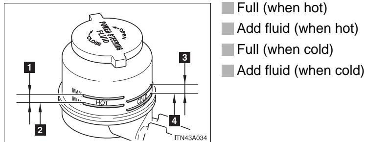
**Hot:** The vehicle has been driven around 50 mph (80 km/h) for 20 minutes, or slightly longer in frigid temperatures. (Fluid temperature, 140 °F - 175 °F [60 °C - 80 °C]).
