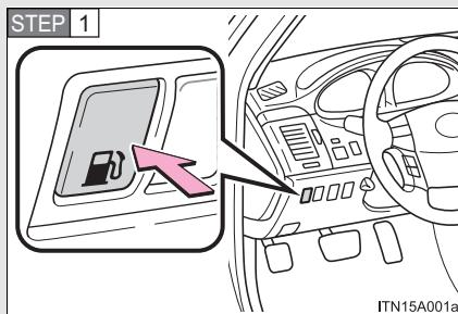
Press the fuel filler door opener switch.
