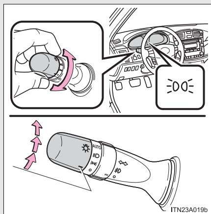
The headlights, parking lights, daytime running lights and so on turn on and off automatically. (When the "ENGINE START STOP" switch is in IGNITION ON mode [vehicles with smart key system] or the engine switch is in the "ON" position [vehicles without smart key system].)
