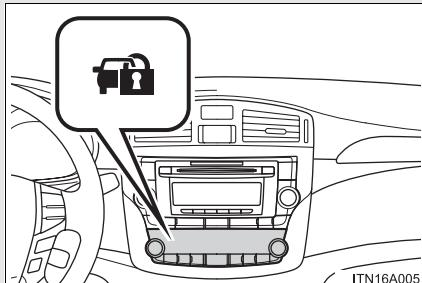
Close the doors, trunk and hood, and lock all doors. The system will be set automatically after 30 seconds.
