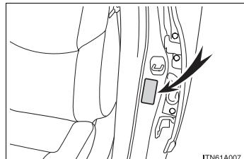
For the GAWR, see the Certification Label. For the maximum load of the tire, see the load limit at maximum cold tire inflation pressure mentioned on the sidewall of the tire. (→P. 519)
