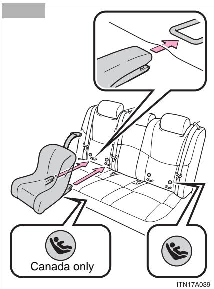
Latch the buckles onto the LATCH anchors.
