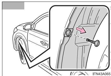
Remove the fender liner clip.
