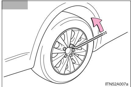
Slightly loosen the wheel nuts (one turn).
