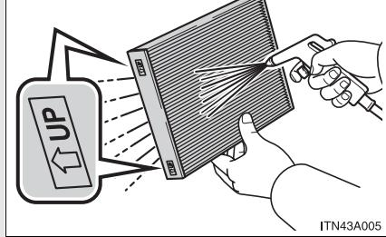
If the filter is dirty, clean by blowing compressed air through the filter from the downward side.
