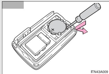
Remove the depleted battery.
