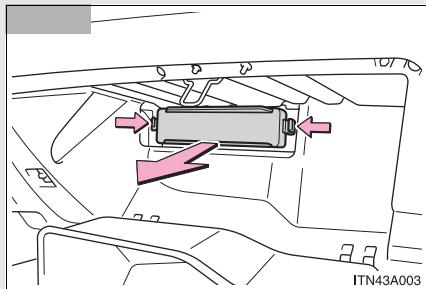
Remove the filter cover while pushing in both ends of the cover.
