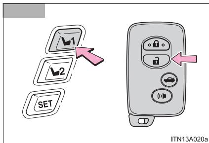
Push the "1" or "2" button on the driver's side and the
