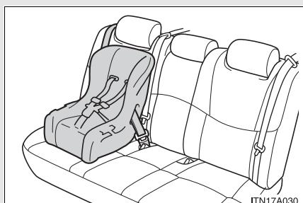
Seat belts equipped with a child restraint locking mechanism (ALR/ELR belts except driver's seat belt) (→P. 68)
