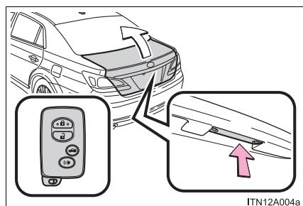
Press the button to unlock the trunk.
