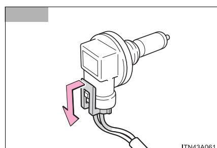
Unplug the connector while pulling the lock release.
