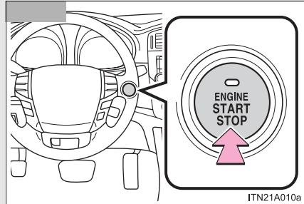
Press the “ENGINE START STOP” switch.
