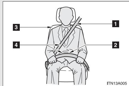
Extend the shoulder belt so that it comes fully over the shoulder, but does not come into contact with the neck or slide off the shoulder.
