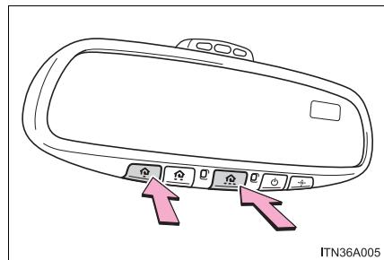
Press and hold down the 2 outside buttons for 10 seconds until the indicator light flashes.
