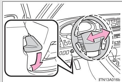
Hold the steering wheel and press the telescopic lock release lever, and adjust to the ideal position by moving the steering wheel horizontally.
