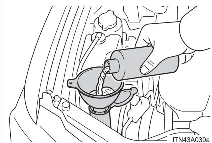
If any washer does not work or the low washer fluid warning light comes on, the washer tank may be empty. Add washer fluid.
