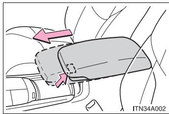
If necessary, the console box lid can slide forward. Pull the lid forward by grasping the front of the lid.
