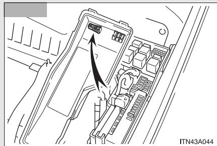
Remove the fuse with the pull-out tool.
