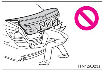
The trunk lid may fall if it is not opened fully. It is more difficult to open or close the trunk lid on an incline than on a level surface, so beware of the trunk lid unexpectedly opening or closing by itself. Make sure that the trunk lid is fully open and secure before using the trunk.
