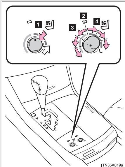
Press the knob to release it, and turn the knob to the desired temperature setting.
