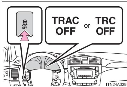
Quickly push and release the button to turn off TRAC/TRC.
