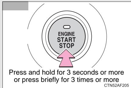
Vehicles with a smart key system: To stop the engine, press and hold the "ENGINE START STOP" switch for 3 consecutive seconds or more, or press it briefly for 3 times or more in succession.
