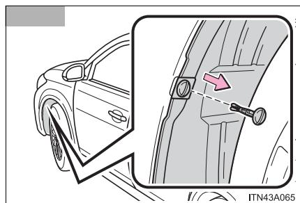
Partly remove the fender liner and turn the bulb base counter-clockwise.
