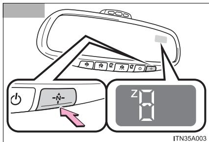
Press the switch until a number (1 to 15) appears on the compass display.
