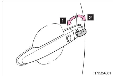
Using the mechanical key (→P. 24) in order to perform the following operations:
