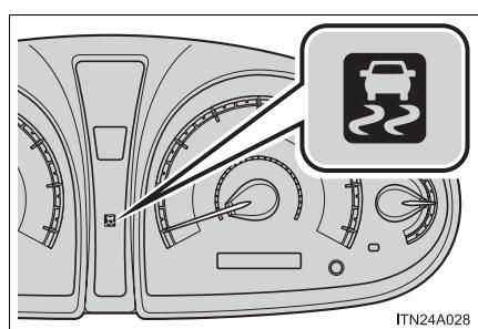
If the vehicle is in danger of slipping, or if the front wheels spin, the slip indicator light flashes to indicate that the VSC/TRAC/TRC have been engaged.
