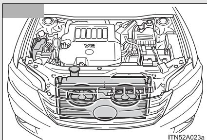
After the engine has cooled down sufficiently, check the coolant level and inspect the radiator core (radiator) for any leaks.
