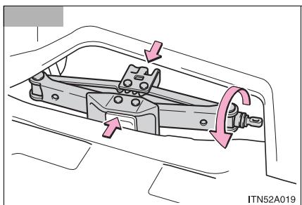
To remove the jack, turn the jack joint by hand until the jack becomes free.
