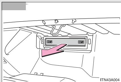
Pull the filter out of the filter outlet.
