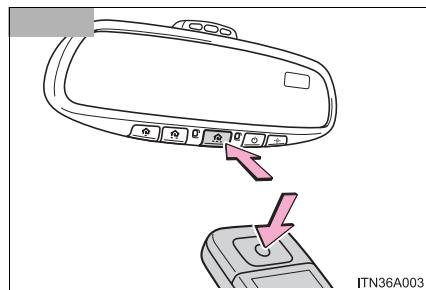
Press and hold one of the HomeLink® buttons and the transmitter button. When the HomeLink® indicator light changes from a slow to a rapid flash, you can release both buttons.
