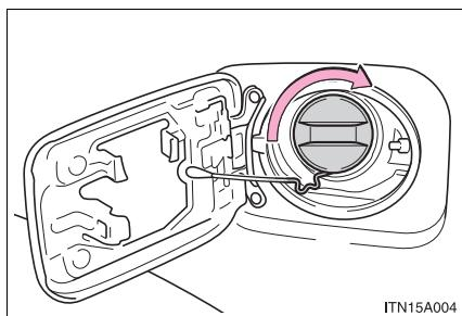
After refueling, turn the fuel tank cap clockwise until you hear a click. The cap will revolve slightly in the opposite direction once released.
