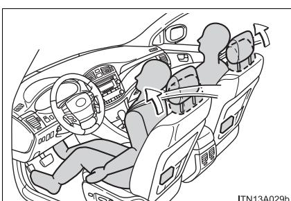
When a front seatback receives a strong impact during a rear-end collision, the head restraint moves slightly forward and upward to provide support for the occupant's head.
