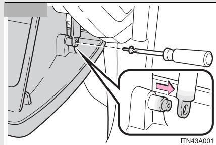
Open the glove box. Remove the screw with a Phillips-head screwdriver and slide off the damper.
