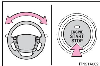
The green indicator light on the "ENGINE START STOP" switch will flash. Press the "ENGINE START STOP" switch again while turning the steering wheel slightly in either direction.
