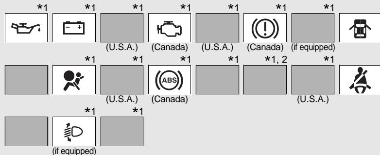
\*1: These lights turn on when the "ENGINE START STOP" switch is turned to IGNITION ON mode (vehicles with smart key system) or the engine switch is turned to the "ON" position (vehicles without smart key system) to indicate that a system check is being performed. They will turn off after the engine is started, or after a few seconds. There may be a malfunction in a system if the lights do not come on, or turn off. Have the vehicle inspected by your Toyota dealer.
