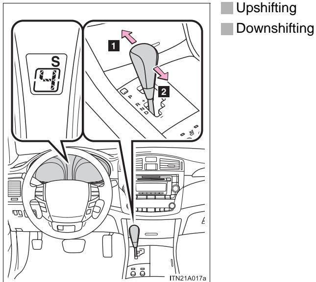
The initial shift range in S mode is set automatically to 5 or 4 according to vehicle speed. However, the initial shift range may be set to 3 if AI-SHIFT has operated while the shift lever was in the D position. (→P. 159)
