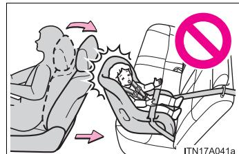
**1** If the driver's seat interferes with the child restraint system and prevents it from being attached correctly, attach the child restraint system to the right-hand rear seat.
