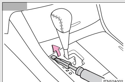
Pry the cover up with a flat-head screwdriver or equivalent.
