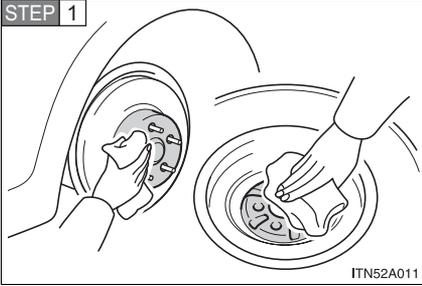
Remove any dirt or foreign matter from the wheel contact surface.
