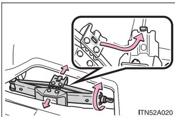
To store the jack, align the hole of the jack head with the vehicle hook. Turn the jack joint until the jack base fits securely with the vehicle body. This prevents the jack from flying forward during a collision or sudden stop.
