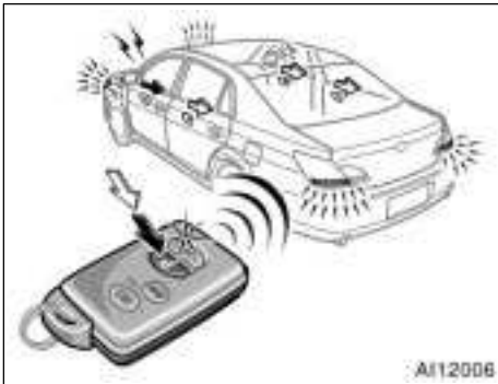
Unlocking operation (vehicles with smart key system)
