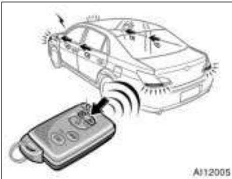
Locking operation (vehicles with smart key system)
