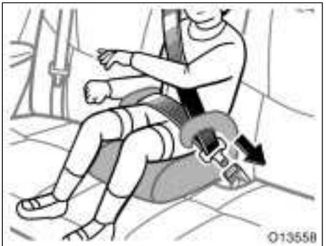
1. Sit the child on a booster seat. Run the lap and shoulder belt through or around the booster seat and across the child following the instructions provided by its manufacturer and insert the tab into the buckle taking care not to twist the belt.
