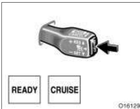
When the ignition is turned off, all the preset data is cleared. When you use the dynamic laser cruise control again, you need to reset the data.
