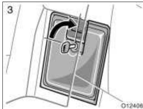
2. After closing the glove box lid, insert the master key (vehicles with key cylinder-type ignition switch) or mechanical key (vehicles with smart key system) and turn it clockwise to safeguard the lock release switch.
