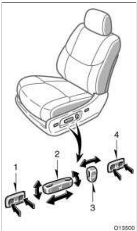
**1. SEAT LEG SUPPORT ADJUSTING SWITCH (some models on driver's side)**
