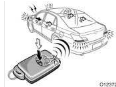
Unlocking operation (vehicles with smart key system)
