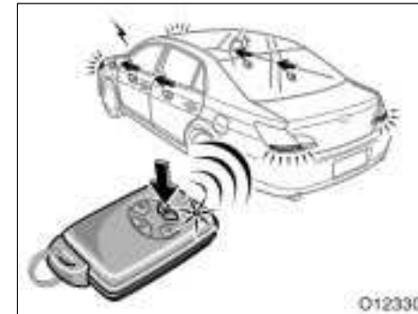
Locking operation (vehicles with smart key system)
