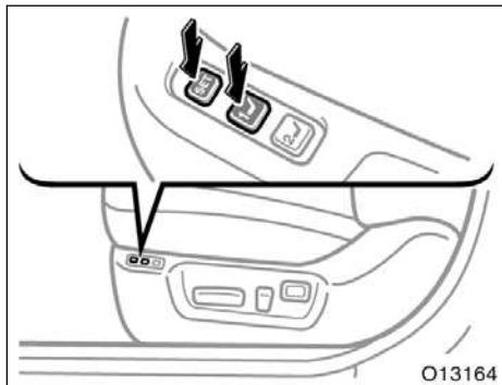
To make only slight changes to an already memorized position, the easiest way is to first activate the memorized position, then make the desired changes and perform step 2 above.
