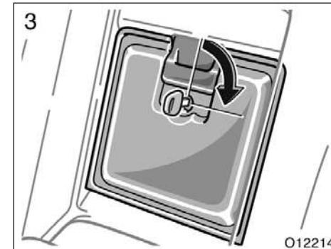
This system helps protect things locked in the trunk by safeguarding the trunk opener main switch from unwanted access.
