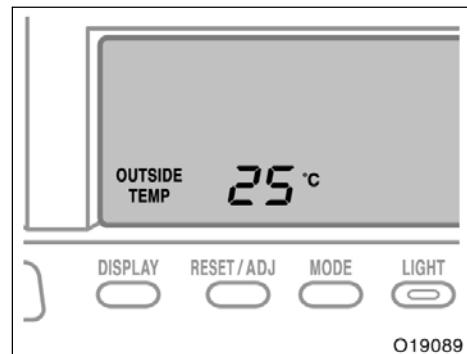
The outside temperature display indicates outside air temperatures.
