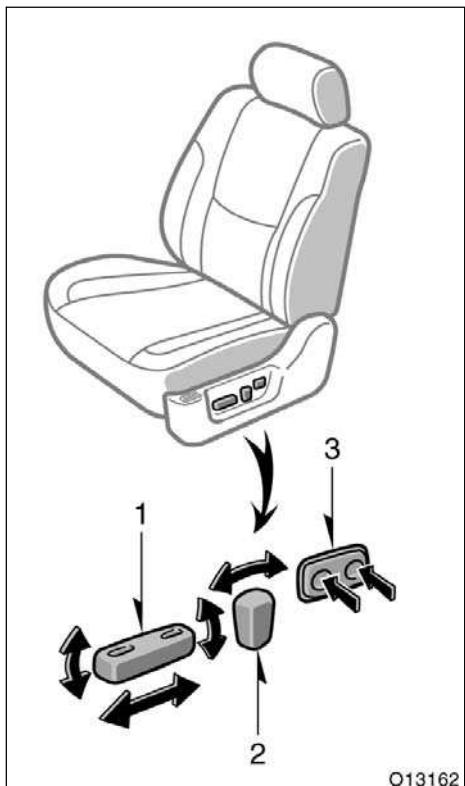
**1. SEAT POSITION AND SEAT CUSHION ANGLE ADJUSTING SWITCH**
