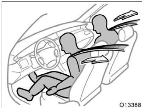
Collisions occurring at certain speeds and angles may cause the seat belt pretensioners and SRS airbags not to operate all together.
