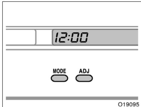
To reset the hour: Push the "MODE" button until the hour display blinks. Then push the "ADJ" button.
