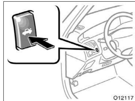
To open the trunk lid from the driver's seat, push the lock release switch.
