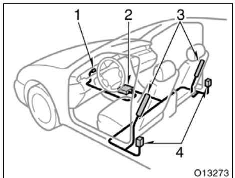
The SRS side airbag system mainly consists of the following components, and their locations are shown in the illustration.
