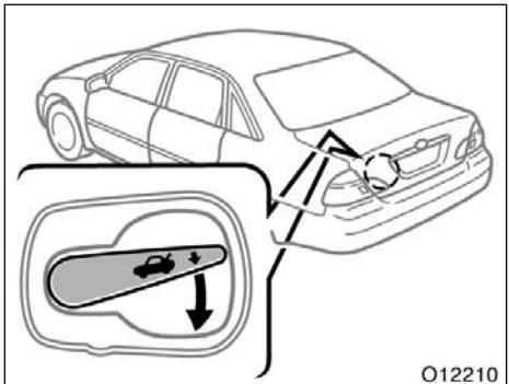
If a person is locked in the trunk, he/she can pull down the phosphorescent handle on the inside of trunk lid to open the trunk lid.
