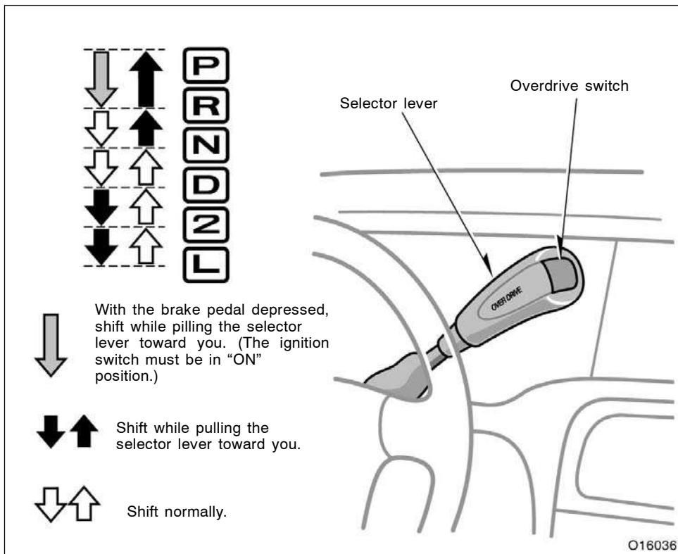
Your automatic transmission has a shift lock system to minimize the possibility of incorrect operation. This means you can only shift out of "P" position when the brake pedal is depressed (with the ignition switch in "ON" position and the selector lever pulled toward you).
