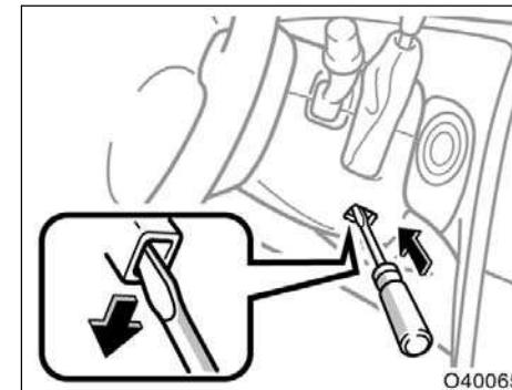
3. Insert the screwdriver or equivalent into the hole to pull down the shift lock override button. You can shift out of "P" position only while pushing the button.
