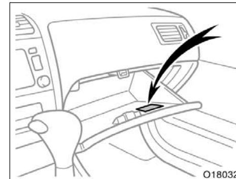
The air conditioning filter information label is placed on the inside of the glove box as shown and indicates that a filter has been installed.
