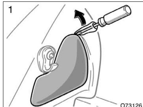
Use a flat-bladed screwdriver which is wrapped with a cloth.
