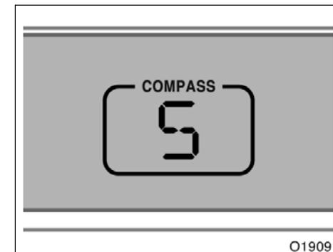
**The compass indicates the direction that the vehicle is heading. In the above case, it shows that the vehicle is heading south.**
