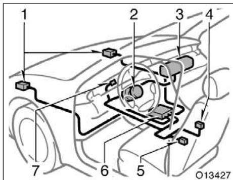
The SRS front airbag system mainly consists of the following components, and their locations are shown in the illustration.
