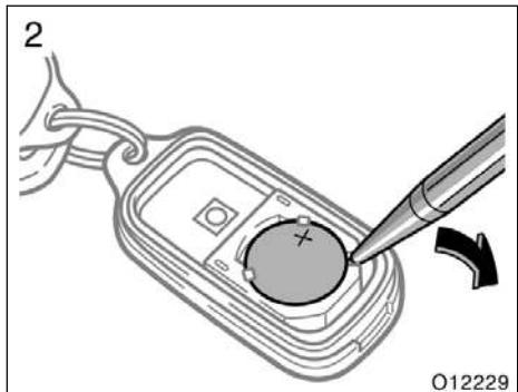
2. Remove the discharged transmitter battery by ballpoint pen. Insert the tip of ballpoint pen at the guide groove and lift as shown in the above illustration.
