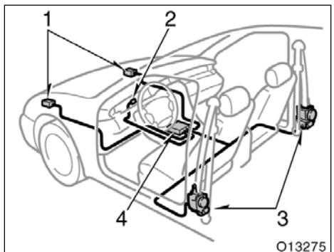
The front outside seat belt pretensioner system consists mainly of the following components and their locations are shown in the illustration.
