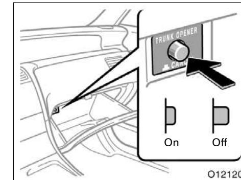
If you do not want to activate the trunk lid opener system, turn off the trunk opener main switch in the glove box. To turn it on, push in the trunk opener main switch.
