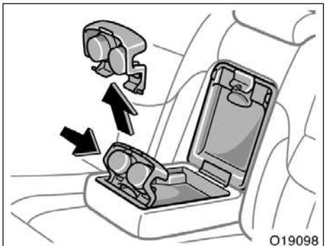
To maximize the storage room, remove the cup holder by pushing the side facing at its upright position.
