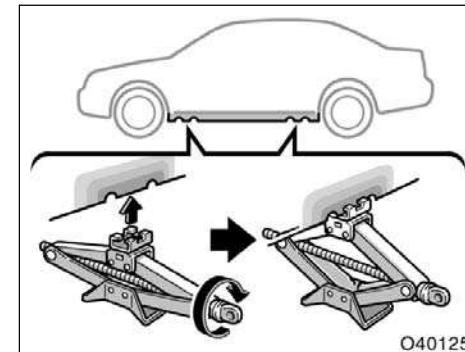
**5. Position the jack at the correct jack point as shown. Rotate the load rest 90° from storage position to lifting position.**
