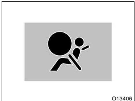
This front outside seat belt pretensioner system has a service reminder indicator to inform the driver of operating problems. If any of the following conditions occurs, this indicates a malfunction of the airbags or pretensioners. Contact your Toyota dealer as soon as possible to service the vehicle.
