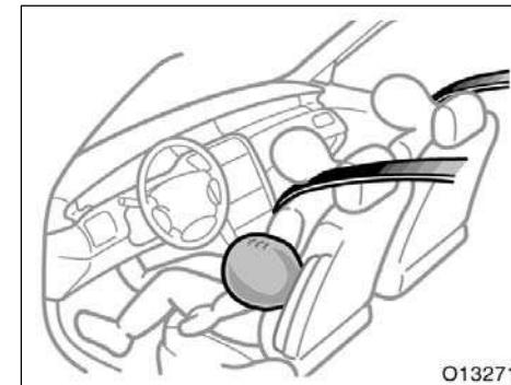
The SRS (Supplemental Restraint System) side airbags are designed to provide further protection for occupants in the following seats in addition to the primary safety protection provided by the seat belts.
