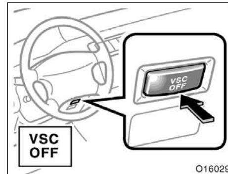
If your wheels get stuck in a ditch when you are driving on a severe off road and sand, turn off the vehicle skid control system. This system that controls engine performance interferes with the process of freeing your wheels.
