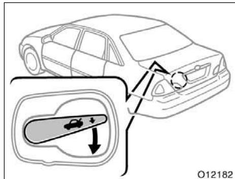
2. After closing the trunk lid, insert the master key and turn it counterclockwise to deactivate the lock release lever.
