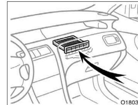
**Automatic air conditioning system only—This air conditioning system has a high efficient air refiner filter which helps eliminate dust and pollen, thereby increasing your driving comfort.**
