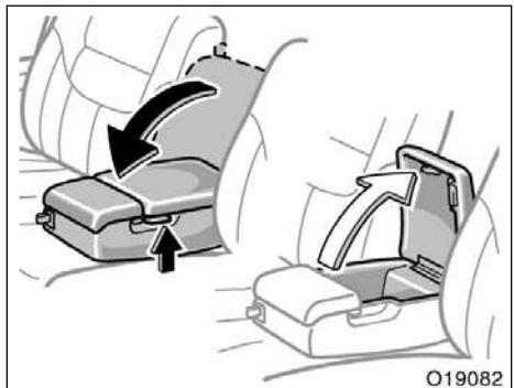
To use the box, pull down the armrest, pull up the lock release lever and open the lid.
