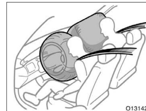
The SRS (Supplemental Restraint System) front airbags are designed to provide further protection for occupants in the following seats in addition to the primary safety protection provided by the seat belts.
