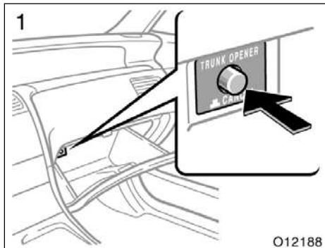
This system helps protect things locked in the trunk by safeguarding the trunk opener cancel switch from unwanted access.
