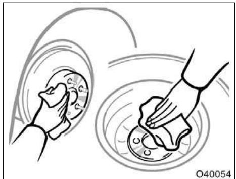
**—Reinstalling wheel nuts**
