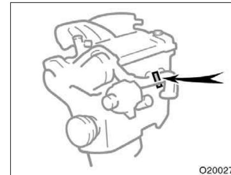
**The engine number is stamped on the engine block as shown.**
