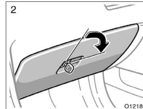
2. After closing the glove box lid, insert the master key into the glove box lock and turn it clockwise to safeguard the lock release switch.
