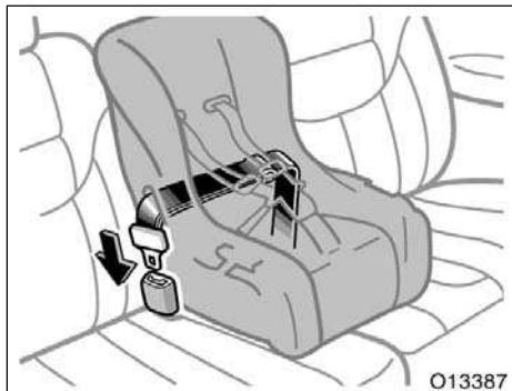
1. Run the center lap belt through or around the convertible seat following the instructions provided by its manufacturer and insert the tab into the buckle taking care not to twist the belt. Keep the lap portion of the belt tight.
