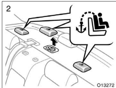
2. Remove the anchor bracket cover with the symbol mark shown in the illustration.
