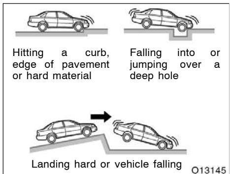
**The SRS front airbags may deploy if a serious impact occurs to the underside of your vehicle. Some examples are shown in the illustration.**
