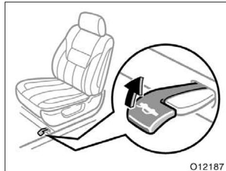
To open the trunk lid from the driver's seat, pull up on the lock release lever.
