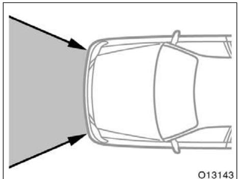
**The SRS front airbag system is designed to activate in response to a severe frontal impact within the shaded area between the arrows in the illustration.**
