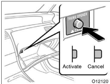
If you do not want to activate the trunk lid opener system, turn off the trunk opener cancel switch in the glove box. To turn it on, push in the trunk opener main switch.
