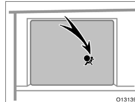
This indicator comes on when the ignition key is turned to the "ACC" or "ON" position. It goes off after about 6 seconds. This means the SRS front airbags are operating properly.
