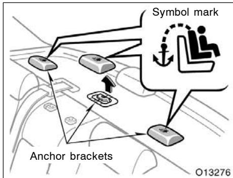
Use the anchor bracket on the package tray to attach the top strap.
