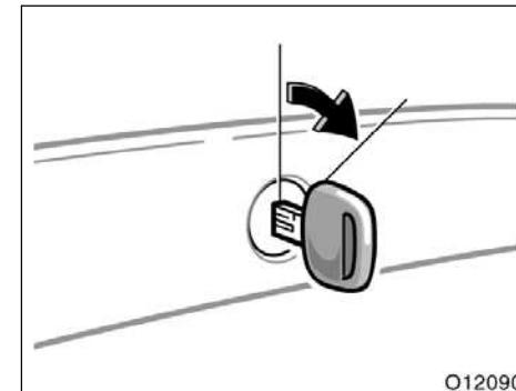
To open the trunk lid from the outside, insert the master key and turn it clockwise.
