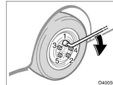
Before putting on wheels, remove any corrosion on the mounting surfaces with a wire brush or such. Installation of wheels without good metal-to-metal contact at the mounting surface can cause wheel nuts to loosen and eventually cause a wheel to come off while driving. Therefore after the first 1600 km (1000 miles), check to see that the wheel nuts are tight.
