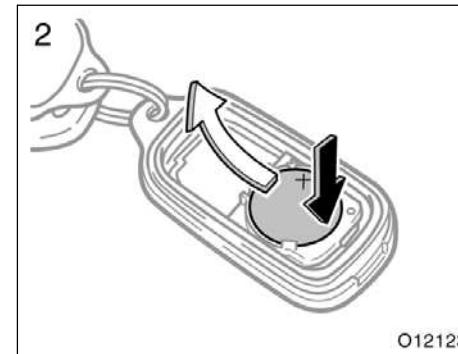
2. Push the edge of the discharged transmitter battery and lift it out as shown in the above illustration.
