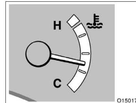
**The gauge indicates the engine coolant temperature when the ignition switch is on. The engine operating temperature will vary with changes in weather and engine load.**
