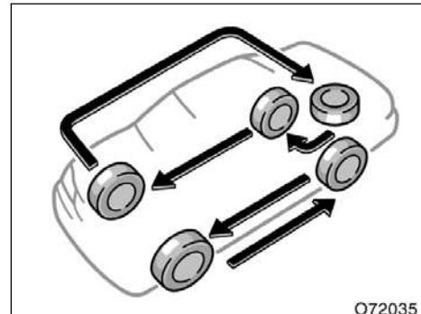
With a spare tire of the same wheel type as the installed tires
