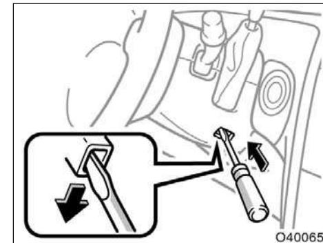
3. Insert the screwdriver or equivalent into the hole to pull down the shift lock override button. You can shift out of "P" position only while pushing the button.
