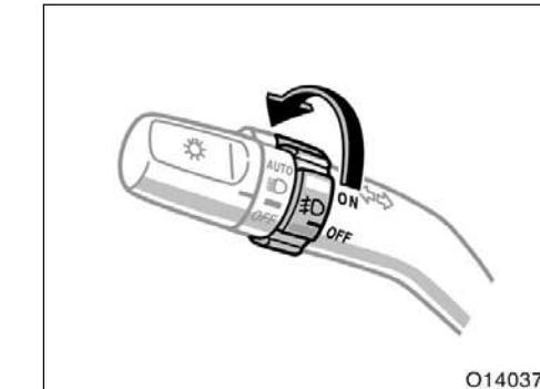
To turn on the front fog lights, twist the band of the headlight and turn signal switch lever. They will come on only when the headlights are on low beam.
