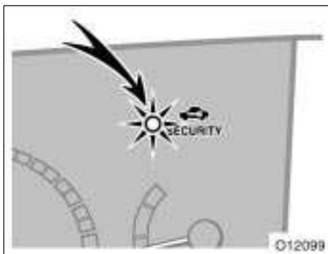
The engine immobiliser system is a theft prevention system. When you insert the key in the ignition switch, the transponder chip in the key's head transmits an electronic code to the vehicle. The engine will start, only when the electronic code in the chip corresponds to the registered ID code for the vehicle.
