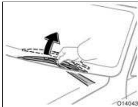
To pull up the windshield wipers to the rest position, hold the connection of the wiper arm and wiper blade and pull it upward along the windshield glass.
