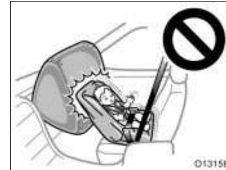
● Never put a rear-facing child restraint system on the front seat because the force of the rapid inflation of the front passenger airbag can cause death or serious injury to the child.
