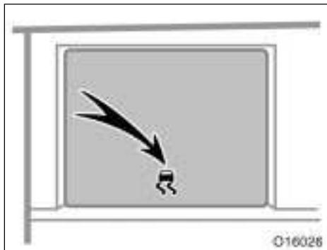
The traction control system automatically helps control the spinning of the front wheels which may occur when accelerating on slippery road surfaces, thus assisting driver to control the driving power of the front wheels.
