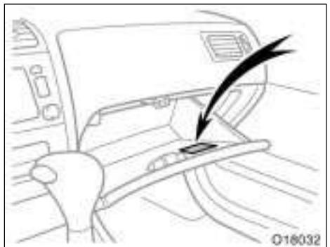
The filter information label is placed on the inside of the glove box as shown.
