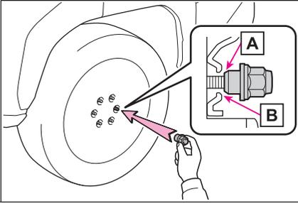
When replacing an aluminum wheel with a spare aluminum wheel, tighten the nuts until the washer of the nut **A** comes into loose contact with the disc wheel **B**.
