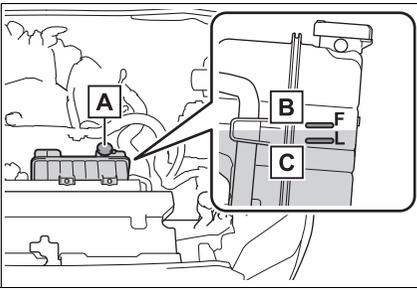
**A** Engine coolant reservoir cap
