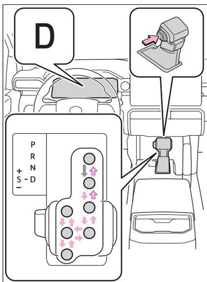
← While the engine switch is in ON and the brake pedal depressed\*, shift the shift lever while pushing the shift release button on the shift knob.
