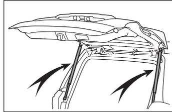
? Do not attach any foreign objects, such as stickers, plastic sheets, or adhesives to the damper stay rod.
