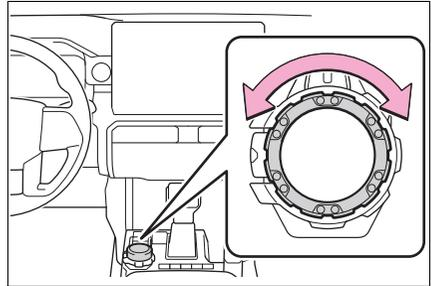
▶ Front-wheel drive control switch is in “4L”
