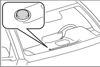
The sensor may not function properly if an object is placed on the sensor, or anything that blocks the sensor is affixed to the windshield. Doing so interferes with the sensor detecting the level of ambient light and may cause the automatic headlight system to malfunction.
