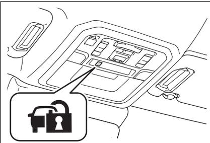
The indicator light flashes after the engine switch has been turned off to indicate that the system is operating.
