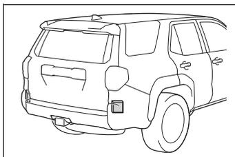
? Do not attach accessories, stickers (including transparent stickers), aluminum tape, etc., to a sensor or its surrounding area on the rear bumper.
