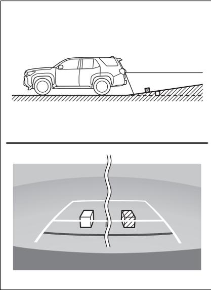
? **When the ground behind the vehicle slopes down sharply**
