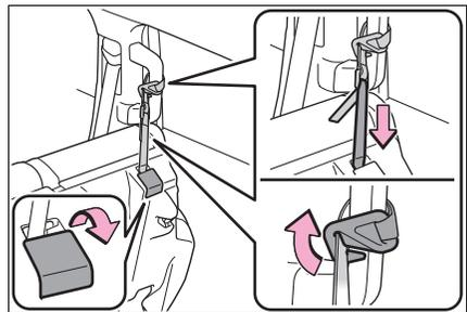
If removing from the assist grip is difficult, loosen the band.
