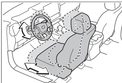
When any of the following has been performed, the driver's seat and steering wheel (power adjustment type) automatically return to their original positions.
