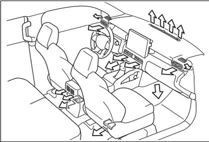
? **Adjusting the air flow direction**
