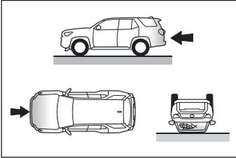
? The following SRS airbags will not normally deploy in rear collisions, end over end vehicle rollovers, or low speed front or side collisions:
