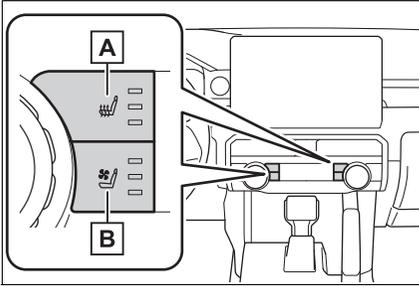
**A** Adjust the front seat heater temperature level
