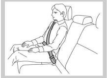
Seatbelts provide maximum restraint when the occupant sits well back and upright in the seat. Do not put cushions or any other materials between occupants and seatbacks or seat cushions. If you do so, the risk of sliding under the lap belt and of the lap
