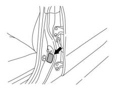
The maximum load you can carry in your vehicle is shown on the tire inflation pressure label attached to the driver's side door pillar. It includes the total weight of the driver and all passengers and their belongings, any optional equipment such as a trailer hitch, roof rack or bike carrier, etc., and the tongue load of a trailer.
