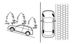
When parking on a hill, always turn the steering wheel as described here. When the vehicle is headed up the hill, the front wheels should be turned away from the curb.
