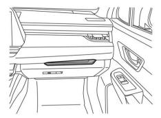
The front passenger's tray is located on the upper side of the glove box.
