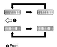
Models with a spare tire of the same wheel type as the installed tires:
