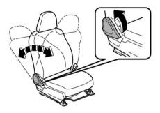
2. Make sure the seatback is securely locked into place.
