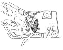
Remove the bulb holder from the rear combination light assembly by turning it counterclockwise.
