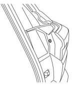
Slide the side cover upward and remove it
