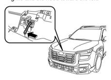
Lift up the hood, release the hood prop from its retainer and put the end of the hood prop into the slot in the hood. Hold the grip for handling the hood prop.
