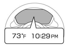
This screen displays the clock and outside temperature.
