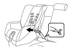
Attach the tether onto the tether anchor and tighten the tether firmly. For additional instructions, refer to "Tether anchors" P82. 8. Before having a child sit in the child restraint system, try to move it back and forth and right and left to check if it is firmly secured. Sometimes a child restraint system can be more firmly secured by pushing it down into the seat cushion. It should not be possible to move the child restraint system more than 1 in (2.5 cm).
