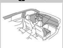
If you notice any damage or cracks where an SRS airbag is stored, have it replaced by an authorized SUBARU dealer.  Do not strike the area around SRS airbag system component parts or subject the area to impact.
