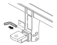
Insert the safety pin through the provided hole on the hitch pin securely.
