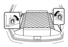
The cargo area is equipped with four tiedown hooks so that cargo can be secured with a cargo net or ropes.
