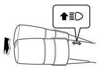
While the light control switch is in the "O" or "AUTO" position in a dark place, the headlights will turn on.
