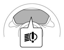
The LED headlight warning light illuminates if the LED headlights malfunction.
