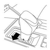
With the vehicle either moving or stationary, move the select lever from the "D" position to the "M" position to select the manual mode.
