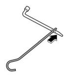
11. Insert the jack handle into the jackscrew, and turn the handle until the tire clears the ground. Do not raise the vehicle higher than necessary.
