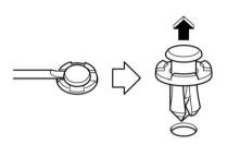
2. Pull the protruded center portion to remove the entire body of the clip.
