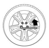
Place the jack under the side sill at the front or rear jack-up point closest to the flat tire.
