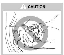
If the floor mat slips forward and interferes with the movement of the pedals during driving, it could cause an accident. Observe the following precautions to prevent the floor mat from slipping forward.
