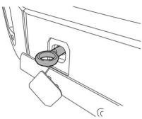
Tighten the towing hook securely using the jack handle and wheel nut wrench
