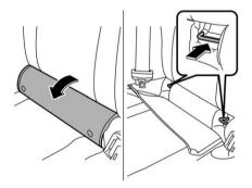
3. If the child restraint system makes contact with the head restraint of the rear seating position where the child restraint system is to be installed, raise the head restraint to the extended position. If the child restraint system still makes contact, remove the head restraint. For details, refer to "Head Restraint Adjustment" #P50.
