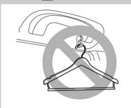
Do not hang coat hangers or other hard or pointed objects on the coat hooks. If such items were hanging on the coat hooks during deployment of the SRS curtain airbags, they could cause serious injuries by coming off the coat hooks and being thrown through the cabin or by preventing deployment of the curtain airbags.
