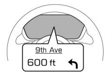
When the route guidance is set in the navigation system, this item shows the navigation route information. For details about the navigation system, refer to the separate navigation/audio Owner's Manual
