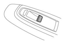
Each passenger's window can be controlled by the power window switch located on the door.
