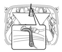
If it is difficult to hang the cargo floor lid from the hook, use a dry cloth to wipe off any material adhering to the opening of the rear gate where you would like to attach the hook.
