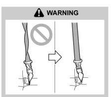
Fastening the seatbelt with the webbing twisted can increase the risk or severity of injury in an accident. When fastening the belt after it is pulled out from the retractor, especially when inserting the anchor tongue plate into the mating buckle (on right-hand side), always check that the webbing is not twisted.
