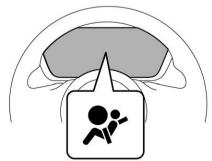
The SRS airbag system warning light will show normal system operation by illuminating for approximately 6 seconds when the ignition switch is turned to the "ON" position.
