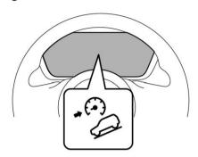
This indicator appears while the hill descent control function is in the standby mode. It flashes while the function is operating. It will disappear when the function is in the disabled mode. When this function is changed from operational to non-operational, it will disappear when the vehicle speed reaches more than approximately 18 mph (30 km/h).
