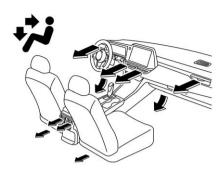
Instrument panel outlets and the foot outlets
