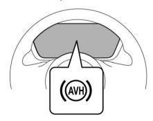
While the vehicle is kept stopped by the Auto Vehicle Hold function, the Auto Vehicle Hold indicator light will flash.
