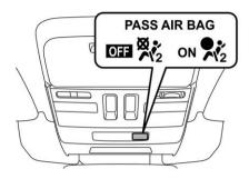
on ∰: Front passenger's frontal airbag ON indicator light
