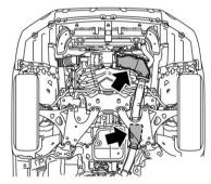
The catalytic converter is installed in the exhaust system. It serves as catalyst to reduce HC, CO and NOx in exhaust gases, thus providing cleaner exhaust.
