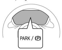
When the parking brake is applied, the following indicator lights illuminate.
