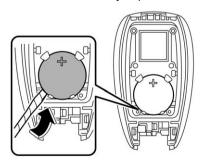
Insert a new battery with its positive (+) side facing upward as shown in the figure.
