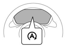
If the engine is temporarily stopped by the system, the Auto Start Stop indicator light on the instrument cluster will illuminate in green. This indicator light will turn off when the system restarts the engine.
