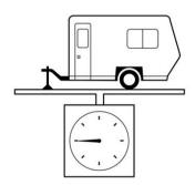
The total trailer weight (trailer weight plus its cargo load) must never exceed the maximum total trailer weight in the following table.
