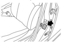
Check the tire pressures when the tires are cold. Use a pressure gauge to adjust the tire pressures to the values shown on the tire inflation pressure label. The tire inflation pressure label is located on the door pillar on the driver's side.
