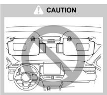
Do not pull out the extension plate with the sun visor positioned over the windshield. The extension plate would obstruct your view of the inside mirror.
