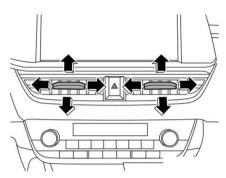
To adjust the airflow direction, move the tab. To close the ventilator, move the tab towards the center of the vehicle.
