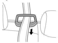
Make sure that the "▼" mark on the anchor tongue plate and the "▲" mark on the anchor buckle face outwards.
