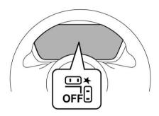
When the Front Cross Traffic Information function is turned OFF, the Front Cross Traffic Braking OFF indicator on the instrument cluster display will illuminate.
