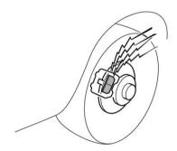
The disc brake pad wear warning indicators on the disc brakes give a warning noise when the brake pads are worn.
