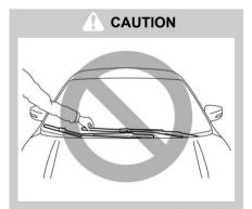
Hold the wiper arm when replacing the wiper blade. Holding the wiper blade, may result in blade deformation.
