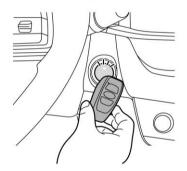
When the communication between the access key fob and the vehicle is completed, a chime (ding) will sound. At the same time, the status of the push-button ignition switch changes to either of the following.
