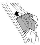
3. Remove the upper and lower screws.
