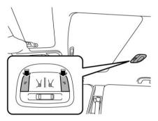
To turn on the dome light, press the switch.
