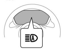
When the high beam assist function is activated, the high beam assist indicator on the instrument cluster will illuminate.
