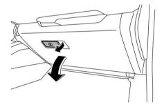
To open the glove box, pull the handle. To close it, push the lid firmly upward.
