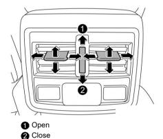
To adjust the flow direction, move the tab.
