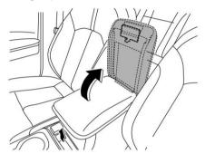
To open the lid, pull up the lock release lever.
