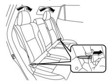
Release the strap and move the seatback back and forth to confirm that it is securely fixed in place.
