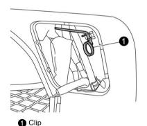
3. Pull the clip to unlock the fuel filler lid.
