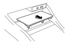
4. While depressing the brake pedal, press the shift lock release portion, and then move the select lever
