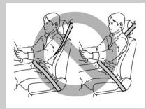
Never place the shoulder belt under the arm or behind the back. If an accident occurs, this can increase the risk or severity of injury.
