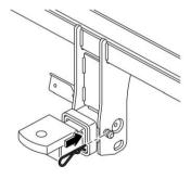
Check the ball mount assembly by pulling on it to make sure it does not come off the hitch receiver.  Use only a hitch ball that is appropriate for the ball mount and your trailer. The hitch ball must be securely installed on the ball mount
