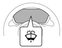
The windshield washer fluid warning light appears when the washer fluid level in the tank has dropped to the lower limit. If the warning light appears, refill the tank with fluid. For the tank refilling method, refer to "Windshield Washer Fluid" # P495.
