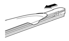
4. Be sure to position the claws at the end of the support between the stoppers on the rubber as shown. If the rubber is not retained properly, the wiper blade may scratch the windshield
