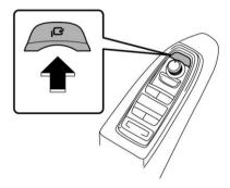
The power folding mirror switch operates when the ignition switch is in the "ON" or "ACC" position.
