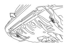
The front tie-down hooks are located between each of the front tires and the front bumper.
