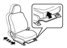
Try to move the seat back and forth to make sure that it is securely locked into place.
