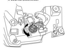
Pull the bulb out of the bulb holder and replace it with a new one.
