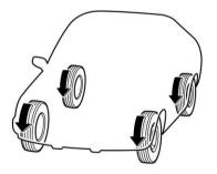
All-Wheel Drive distributes the engine power to all four wheels. AWD vehicles provide better traction when driving on slippery, wet or snow-covered roads and when moving out of mud, dirt and sand. By shifting power between the front and rear wheels, SUBARU AWD can also provide added traction during acceleration, and added engine braking force during deceleration.
