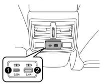
USB Type-C: DC 5 V/3.0 AUSB Type-A: DC 5 V/2.4 A
