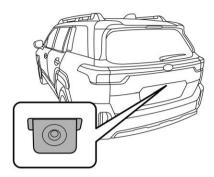
A rear view camera is attached to the rear gate. When the ignition switch is in the "ON" position and the select lever is set to "R", the rear view camera automatically displays the rear view image behind the vehicle on the center information display.
