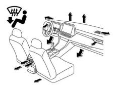
Windshield defroster outlets, foot outlets and both side outlets of the instrument panel
