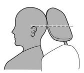
Each head restraint should be adjusted so that the center of the head restraint is closest to the top of the occupant's ears.
