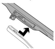
4. When installing the wiper blade assembly, align it with the wiper arm connection part and then slide it in the opposite direction of removal to install. After installing the wiper blade assembly, close the lock cover and check that the connection part is locked completely.
