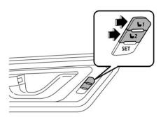
A chirp will sound and the seat and outside mirror move to the registered position.
