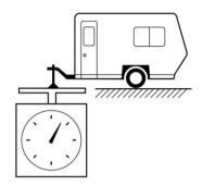
Ensure that the trailer tongue load is from 8% to 11% of the total trailer weight and does not exceed the maximum value. For details about the trailer tongue load, refer to "Trailer hitch" "Trailer Hitch (Dealer Option)" \$\times P424\$.
