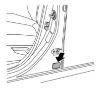
The certification label attached to the driver's side door pillar shows GVWR (Gross Vehicle Weight Rating) and GAWR (Gross Axle Weight Rating).
