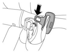
3. With the belt held by hand, allow the retractor to roll up the belt slowly. You should hold the webbing end and guide it back into the retractor while it is rolling up. Neatly store the tongue plate in the recess on the ceiling and then insert the anchor tongue plate into the slot located at the front of the recess.
