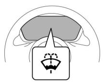
When there is only a small amount of washer fluid remaining, the windshield washer fluid warning light will appear. When this occurs, refill the washer fluid as follows.
