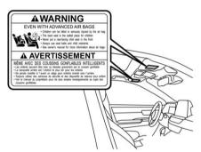
This vehicle has warning labels on the driver's and front passenger's sun visors beginning with the phrase "EVEN WITH ADVANCED AIR BAGS" and a tag attached to the glove box lid beginning with the phrase "Even with Advanced Air Bags". Make sure that you carefully read the instructions on the warning labels and tag.
