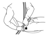
5. To tighten the lap part, pull up on the shoulder belt.
