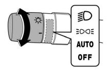
To turn on the headlights, turn the knob on the end of the light control switch.
