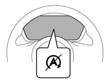
If the operational conditions are not met when the vehicle is stopped, the engine will not stop and the Auto Start Stop No Activity Detected indicator light will illuminate. It will turn off when the vehicle begins to drive.
