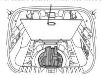
The under-floor storage compartment is located under the floor of the cargo area and can be used to store small items. To open the lid, pull the handle up.
