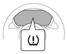
The tire pressure monitoring system provides the driver with the warning message indicated by sending a signal from a sensor that is installed in each wheel when tire pressure is severely low.
