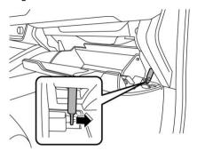
Push both sides of the glove box inward to unlock the stoppers and then pull down the glove box as far as it will go.
