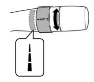
Turn the dial to adjust the sensitivity of the rain sensor for wiper control. Turn the dial downward to increase the sensitivity. Turn the dial upward to decrease the sensitivity.
