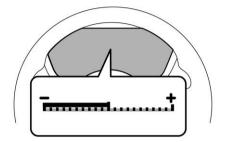
The ECO gauge shows the difference between the average rate of fuel consumption since the trip meter was last reset and the current rate of fuel consumption.
