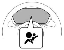
If the seatbelt buckle switch and/or front passenger's occupant detection system have failed, the SRS airbag system warning light will illuminate. If the SRS airbag system warning light illuminates, immediately stop the vehicle in a safe place, and consult a SUBARU dealer.
