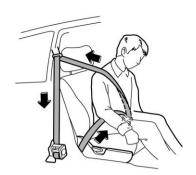
If the sensor detects a certain predetermined amount of force during frontal or side collisions or rollover accidents, any seatbelt that has a seatbelt pretensioner is quickly drawn back in by the retractor to take up the slack so that the belt more effectively restrains the seat occupant.
