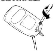
Carefully pry the remote engine start transmitter halves apart using a small flat-head screwdriver.
