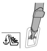
12. To remove the child restraint system, press the release button on the seatbelt buckle and allow the belt to retract completely. The belt will return to the ELR mode.
