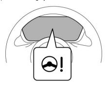
When the ignition switch is turned to the "ON" position, the power steering warning light on the instrument cluster illuminates to inform the driver that the warning system is functioning properly. Then, if the engine started, the warning light turns off to inform the driver that the steering power assist is operational.
