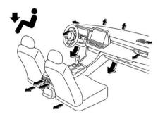
Foot outlets, both side outlets of the instrument panel and some through windshield defroster outlets (A small amount of air flows to the windshield and both side windows to prevent fogging.)
