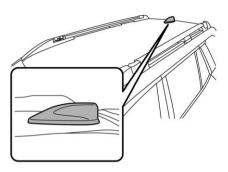
The satellite radio antenna is installed in the center of the roof at the rear.
