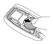
Attach the cover to the access key fob by fitting the projections and recesses together.
