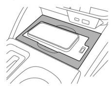
The mobile device holder is an accessory designed to securely hold smartphones and other devices placed on the wireless charger.
