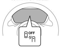
When the BSW/RCTW system is turned OFF, the BSW/RCTW OFF indicator on the instrument cluster display will illuminate.
