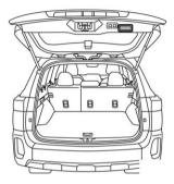
Pull down the rear gate when the rear gate is opened. The rear gate will close automatically.
