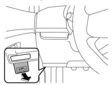
Release the secondary hood release by moving the lever between the front grille and the hood toward the left.
