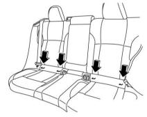
Two lower anchors are provided for installing a child restraint system in the rear seat window-side seating positions. Lower anchors for window-side seating positions may be used for a seat in the center seating position if a child restraint system manufacturer's instructions permit this installation method and specify using anchors as far apart as those in this vehicle. Each lower anchor is located where the seat cushion meets the seat-back
