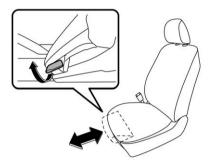
The seat front length can be adjusted. Pull up the lever to adjust the length and release the lever to lock it.
