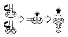
2. Remove the clips with a flat-head screwdriver using leverage.
