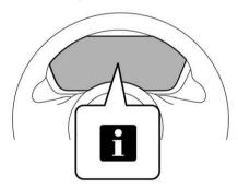
The warning screen will return to the original screen after a few seconds. While the [i] information reminder is shown on the display, it may be possible to display the warning screen again. To recall the message marked with [i] on the display, press and hold the steering wheel.
