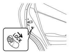
Each rear door has a child safety lock. When the child safety lock lever is in the "LOCK" position, the door cannot be opened from inside. The door can only be opened from the outside.
