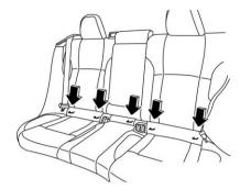
There are a total of 5 lower anchors at the rear seat. The second lower anchor from the right side is used for both the right seat and center seat. Each lower anchor is located where the seat cushion meets the seatback.
