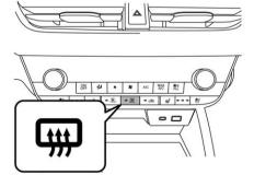
To activate the defogger and deicer system, press the defogger button. The rear window defogger, outside mirror defogger and windshield wiper deicer are activated simultaneously. The indicator light on the defogger button illuminates while the defogger and deicer system is activated
