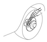
The disc brakes have audible wear indicators on the brake pads. If the brake pads wear close to their service limit, the wear indicator makes a very audible scraping noise when the brake pedal is applied.
