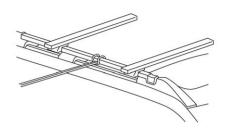
When placing a load laterally on the vehicle, such as by tying a rope directly to the roof rails, ensure you follow these guidelines. Incorrect usage of the roof rails can warp or damage both the vehicle body and the roof rails.
