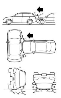
The driver's and front passenger's SRS frontal airbags are not designed to deploy in most of the following cases.
