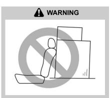
Never stack luggage or other cargo higher than the top of the seatback because it could tumble forward and injure passengers in the event of a sudden stop or accident.
