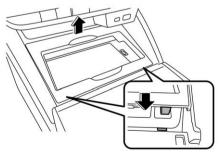
3. Place the mobile device holder onto the wireless charger.
