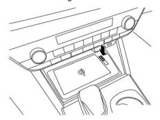
Place the mobile device so that the screen or keypad is facing up (the charging surface is facing downward).
