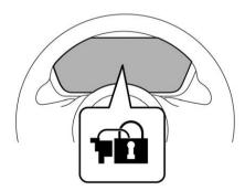
All doors, the rear gate and fuel filler lid will lock, an electronic chirp will sound once, the hazard warning flashers will flash once, and the security indicator light will start flashing rapidly.
