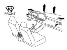
After defrosting the windshield by pressing the defroster button "\(\vec{w}\)", pressing the button again returns the system to the setting that had been selected before the defroster was activated.
