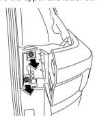
Slide the rear combination light assembly rearward to remove it from the vehicle.
