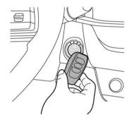
When the communication between the access key fob and the vehicle is completed, a chime (ding) will sound. At the same time, the push-button ignition switch turns to the "ACC" or "ON" position.
