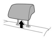
Raise the head restraint to the extended position. If the booster seat still makes contact, remove the head restraint. For details, refer to "Head Restraint Adjustment" \$\textit{P} P50.
