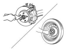
14.Put on the spare tire. Replace the wheel nuts. Tighten them by hand.
