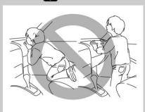
Never allow a child to stand up or kneel on the front passenger's seat. The SRS airbag deploys with considerable force and can injure or even kill the child.
