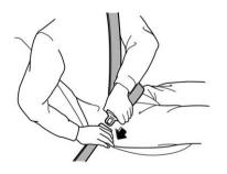
To tighten the lap part, pull up on the shoulder belt
