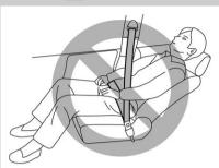
To prevent the passenger from sliding under the seatbelt in the event of a collision, always put the seatback in the upright position while the vehicle is in motion. Also, do not place objects such as cushions between the passenger and the seatback. If you do so, the risk of sliding under the lap belt and of the lap belt sliding up over the abdomen will increase, and both can result in serious injury or death.
