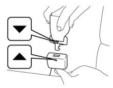
After confirming that the webbing is not twisted, insert the anchor tongue plate attached at the webbing end into the buckle on the right-hand side until a click sounds
