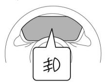
The front fog light indicator light located on the instrument cluster will illuminate when the front fog lights are on.
