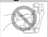
Do not press your feet onto the instrument panel. Doing so may prevent the occupant detection function of the SRS airbag system and SRS airbag from functioning correctly. This may result in serious injury or death in the event of an accident.
