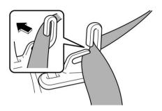
Pull the strap and adjust the seatback to the desired position.
