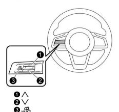
By operating  $\bigwedge$  or  $\bigvee$  of the control switches, the screens can be changed.
