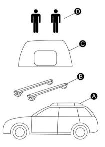
within the roof rail load limit of 220 lbs (100 kg). Refer to the user manual that accompanied the roof tent for important safety information and instructions on the proper installation and use of the tent.
