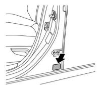
GVWR of your vehicle that is given by SUBARU is shown on the certification label located at the bottom of driver's side door pillar of your vehicle.
