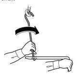
After towing, remove the towing hook from the vehicle and stow it in the underfloor storage compartment.
