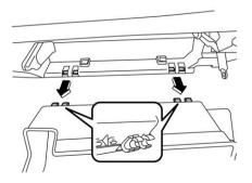
Pinch both tabs and remove the filter cover.
