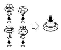
Insert the clip without the center portion first and then push the center portion of the clip into the hole.
