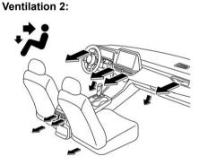
Instrument panel outlets and foot outlets
