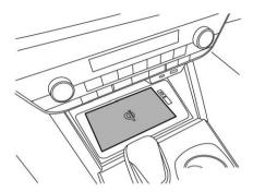
To charge a cell phone, smartphone or a similar mobile device compatible with the Qi wireless charging standard, place the device in the charging area located below the center information display.
