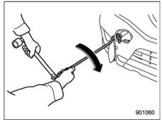
Tighten the towing hook securely using the jack handle and wheel nut wrench. After towing, remove the towing hook from the vehicle and stow it in the under-floor storage compartment.
