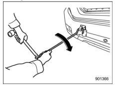
4. Tighten the towing hook securely using the jack handle and wheel nut wrench.
