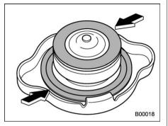
After refilling the reserve tank and the radiator, reinstall the cap and check that the rubber gaskets inside the radiator cap are in the proper position.
