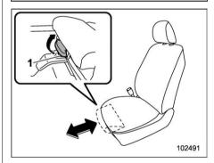
The seat front length can be adjusted. Pull up the lever "1" to adjust the length and release the lever to lock it.
