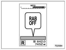
After the brake pedal is depressed, the RAB OFF indicator will illuminate and the system will temporarily stop operating. The RAB OFF indicator will turn off when the select lever is shifted to a position other than the "R" position.
