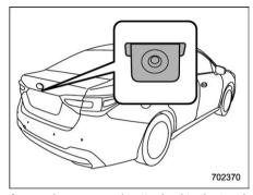
A rear view camera is attached to the trunk lid (Legacy) or rear gate (Outback/Subaru Outback Wilderness). When the ignition switch is in the "ON" position and the select lever is set to "R", the rear view camera automatically displays the rear view image behind the vehicle on the center information display.
