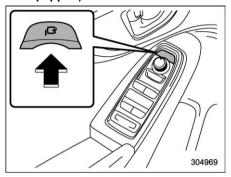
The power folding mirror switch operates when the ignition switch is in the "ON" or "ACC" position.
