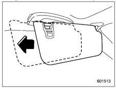
With the sun visor positioned over the side window, you can slide the sun visor toward the rear to prevent glare through the gap between the sun visor and center pillar. To slide the sun visor, pull it toward the rear of the vehicle. When you have finished sliding it, push it toward the front of the vehicle.
