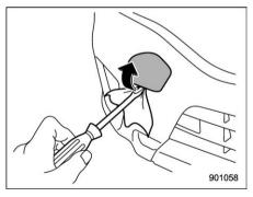
Cover the tip of a flat-head screwdriver with vinyl tape or cloth so that it will not scratch the bumper. Insert the flathead screwdriver into the cutout of
