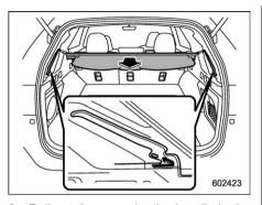
2. Pull out the cover by the handle in the center to extend it. Then insert the stoppers into the catches as shown.
