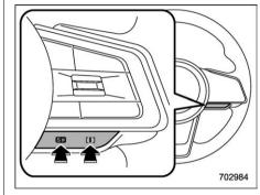
To select the intelligent (I) mode, press the "I" side of the switch. To select the Sport Sharp (S#) mode, press the "S#" side of the switch
