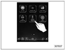
To turn the Vehicle Dynamics Control on and off, touch the "Vehicle Dynamics Control" icon.
