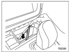
4. While depressing the brake pedal, insert the screwdriver into the hole. press the shift lock release portion using the screwdriver, and then move the select lever
