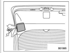
Apply a flat-head screwdriver to the light cover or rear gate light (if equipped) as shown in the illustration, and pry the light cover off from the rear gate trim.
