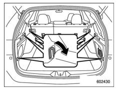
The cargo area is equipped with several tie-down hooks so that cargo can be secured with a luggage net or ropes.
