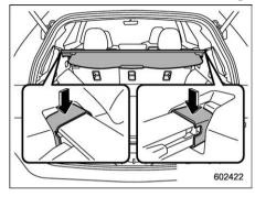
1. Insert the left side cover housing end into the retainer, then insert the right cover housing end into the right retainer.
