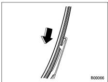
Align the claws of the plastic support with the grooves in the blade rubber assembly, then slide the blade rubber assembly into place.
