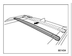
Check that the rear crossbar is stowed in the front side holder. If the rear crossbar is stowed in the rear side holder, move it back to the front side holder (original position).
