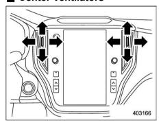
Move the tabs to adjust the flow direction. To close the ventilator, move the tab all the way down.
