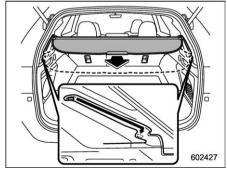
To lower the lifted cover, hold the cover by the handle and pull it back into to the catches.
