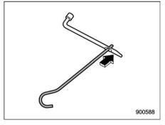
10. Insert the jack handle into the hole of the wheel nut wrench.
