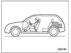
Vehicle capacity weight of the vehicle is 800 lbs (363 kg), which is indicated on the vehicle placard with the statement "The combined weight of occupants and cargo should never exceed 363 kg or 800 lbs".
