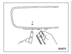
While the HomeLink® indicator light is flashing orange, press and hold the hand-held remote button. Continue pressing the hand-held remote button until the HomeLink® indicator light changes from orange to green. You may now release the hand-held remote button.
