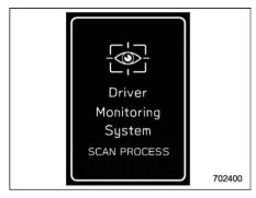
When the door is opened and the push-button ignition switch is OFF, the user recognition screen appears and the Driver Monitoring system starts user recognition.
