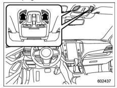
To turn on the map light, press the lens. To turn it off, press the lens again.
