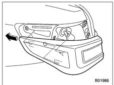
Reinstall the rear combination light assembly by sliding the two-pronged part of the combination light assembly securely to each holder of the vehicle side.
