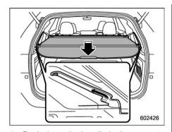
Push down the handle in the center to lift the cover up.
