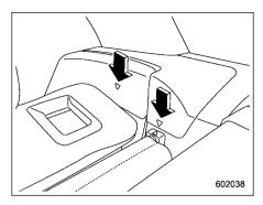
Align the right side of the front cover rod end with a triangle mark on the cargo area trim.
