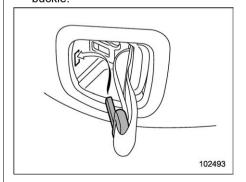
Allow the retractor to roll up the belt. You should hold the webbing end and guide it back into the retractor while it is rolling up. Neatly store the tongue plate in the recess and then insert the anchor tongue plate into the slot.
