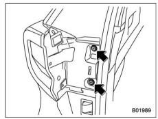
3. Remove the upper and lower screws.
