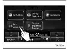
To turn the Auto Vehicle Hold function on and off, touch the "Auto Vehicle Hold" icon. When the Auto Vehicle Hold function is turned off, the Auto Vehicle Hold indicator liaht will turn off.
