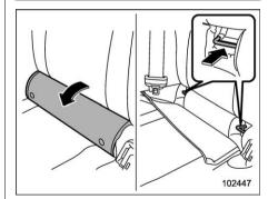
Peel off the anchorage cover completely from the selected side of the rear seatback to expose the anchorages (bars) to be used for installation of the child restraint system.
