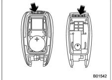
5. Attach the cover to the access key fob by fitting the projections and recesses together.
