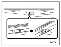
2. Turn the wiper blade assembly counterclockwise.
