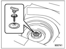
Take out the under-floor storage compartment and turn the attaching bolt counterclockwise, then take the spare tire out.
