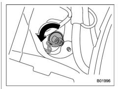
Turn the bulb socket counterclockwise and remove it.
