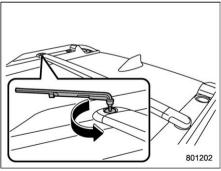
3. Remove the bolt of the crossbar by using the torque wrench and pull this side out.
