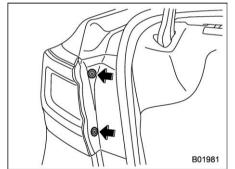
Undo the clips. For the method to undo the clips, refer to "Type C clips" P522.
