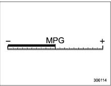
The ECO gauge shows the difference between the average rate of fuel consumption since the trip meter was last reset and the current rate of fuel consumption.
