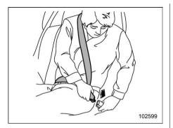
5. Insert the center seatbelt tongue plate into the center seatbelt buckle until it clicks.
