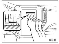
Touch the screen and move the screen to the desired position.
