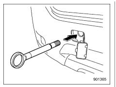
Screw the towing hook into the threaded hole until its thread can no longer be seen.
