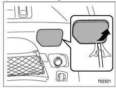
Remove the access cover at the rightside of the cargo area trim using a flathead screwdriver.
