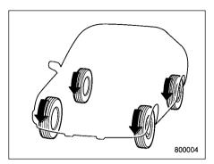
All-Wheel Drive distributes the engine power to all four wheels. AWD vehicles provide better traction when driving on slipperv, wet or snow-covered roads and when moving out of mud. dirt and sand. By shifting power between the front and rear wheels, SUBARU AWD can also provide added traction during acceleration, and added engine braking force during deceleration.
