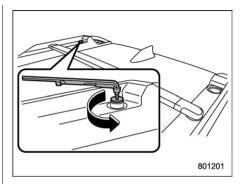
2. Remove the plastic plug of the roof rail holder by using the torque wrench.
