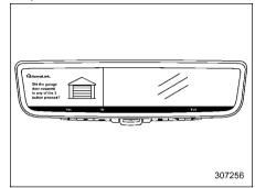
"Program Success": If the programmed HomeLink button works, select "Yes" and programming is completed. If the programmed HomeLink button does not work, select "No" and pro-
