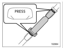
To connect the extender to the seatbelt, insert the tongue plate into the seatbelt buckle so that the "PRESS" marks on the buckle-release buttons of the extender and the seatbelt are both facing the same direction, as shown in the illustration. You will hear a click when the tongue plate locks into the buckle.
