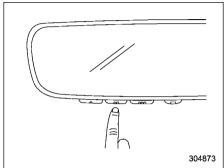
Return to the vehicle and firmly press, hold for 2 seconds and release the HomeLink® button up to three times. At this point programming is complete and your device should operate when the HomeLink® button is pressed and released.
