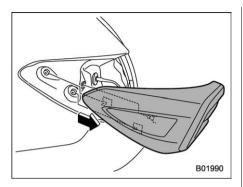
4. Slide the rear combination light assembly straight rearward and remove it from the vehicle.
