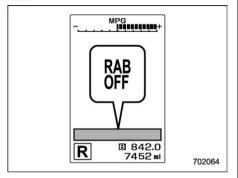
The RAB OFF indicator will turn off when the corresponding function is turned ON.
