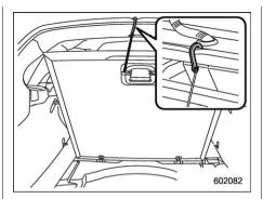
Use the hook provided on the back to hang the cargo floor lid open. The hook can be hanged onto the opening of the rear gate.
