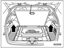
3. Remove the left and right corners of the cargo floor lid.
