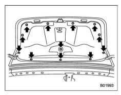
Remove the trunk trim lining by removing the clips indicated in the illustration.
