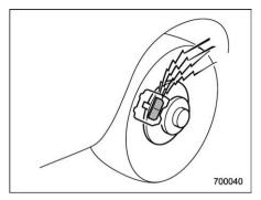
The disc brakes have audible wear indicators on the brake pads. If the brake pads wear close to their service limit, the wear indicator makes a very audible scraping noise when the brake pedal is applied. The disc brakes have audible wear inapplied.
