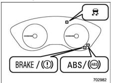
If a malfunction occurs in the EBD system. the system stops working and the following warning lights illuminate simultaneously.
