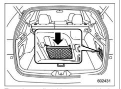
There is an adjustable storage net in the cargo area. Push the net downward to expand the cargo area.
