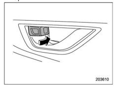
Rotate the lock lever forward
