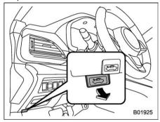
Pull the hood release knob under the instrument panel.
