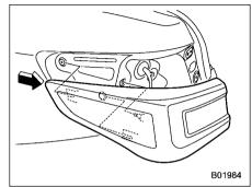
4. Slide the rear combination light assembly straight rearward and remove it from the vehicle.
