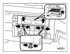
3. Replace the cabin air filter with a new one and then reinstall the cover.
