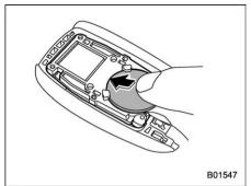
Insert a new battery with its positive (+) side facing upward as shown in the figure.
