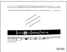
Press any of the left, center or right buttons to display the main menu. Select HomeLink menu using the left button. Select "STATUS" using the center button.
