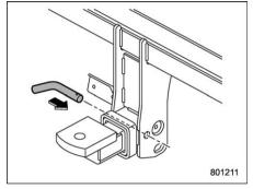
2. Insert the hitch pin into the hole located on the hitch receiver tube so that the pin passes through the ball mount.
