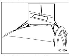
Each of the two roof moldings has two mounting points for crossbars. Each mounting point is fitted with a cover. Use a screwdriver to open the covers. When installing the crossbars on the roof molding, follow the manufacturer's instructions.
