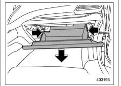
(3) Push both sides of the glove box inward to unlock the stoppers and then pull down the glove box as far as it will go.
