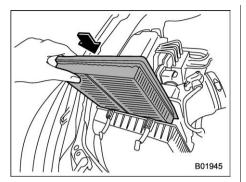
Install a new air cleaner element in the way the longitudinal side and the transverse side face as shown in the illustration.
