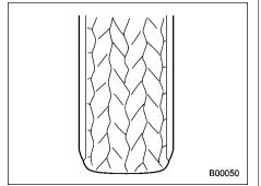
Roadholding is good, and steering is responsive. Rolling resistance is low, so fuel consumption is also lower.
