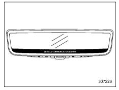
When there is a vehicle communication error, the warning indicators will appear as shown in the illustration.
