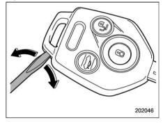
Open the key head using a flat-head screwdriver.
