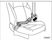
The extender adds approximately 8 inches (200 mm) of length and it can be used for either the driver or front passenger seating position.
