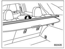
3. Remove the front cover and place it on the cover housing.
