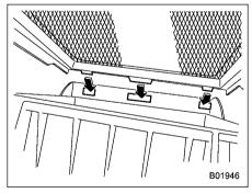
6. To install the air cleaner case (rear), insert the three projections on the air
