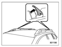
1. Pull out the integrated crossbars from the roof rail holders by pulling up the covers.
