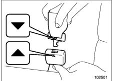
Make sure that the "▼" mark on the anchor tongue plate and the "▲" mark on the buckle face outwards.
