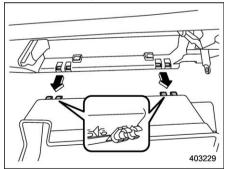
(4) Pull out the glove box horizontally and remove the hinge portion.
