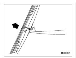
Pull the wiper blade assembly toward you to remove it from the wiper arm.
