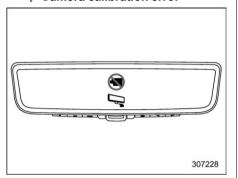
When there is a camera calibration error, the warning indicators will appear as shown in the illustration.
