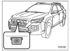
The image from the camera mounted inside the front grille is displayed in the center information display.
