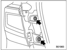
3. Remove the upper and lower screws.
