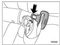
Insert a tongue plate or other hard pointed object into the slot in the connector (buckle) on the right-hand side and push it in. The anchor tongue plate will then disconnect from the buckle.
