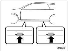
Place the jack under the side sill at the front or rear jack-up point closest to the flat tire.
