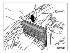
Install a new air cleaner element in the way the longitudinal side and the transverse side face as shown in the illustration.
