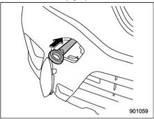
Screw the towing hook into the threaded hole until the threads can no longer be seen.
