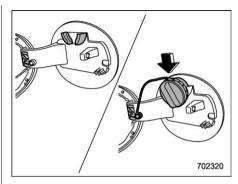
Set the fuel filler cap on the cap holder inside the fuel filler lid.
