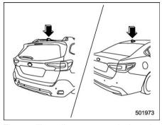
The satellite radio antenna and telematics antenna (if equipped) are installed in the center of the roof at the rear.
