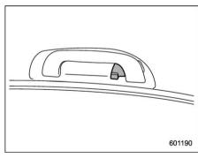
The coat hook is attached to each rear passenger's assist grip.
