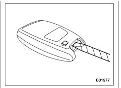
Wrap a flat-head screwdriver with vinyl tape or a cloth, and insert it in the gap to remove the cover.
