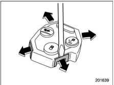
Open the transmitter case by releasing the hooks
