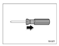
3. Remove the grip portion of the screwdriver.
