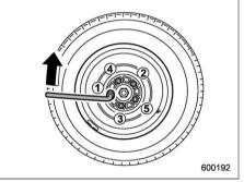
16. Use the wheel nut wrench to securely tighten the wheel nuts to the specified torque, following the tightening order in the illustration.
