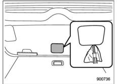
Remove the access cover at the bottom-center of the rear gate trim using flat-head screwdriver.
