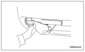
3. Turn the towing hook cover clockwise, pivoting it about the side that is next to the fog lamp. Pull out the towing hook cover to remove it.
