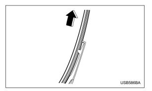
$\ensuremath{\mathsf{2}}.$  Pull the blade rubber assembly out of the plastic support.
