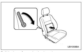
Pull the lever forward or backward. Pulling the lever forward will increase the amount of support for your lower back.
