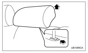
**Center seating position:** Pull the headrest up while pressing the release button located on the top of the seatback.
