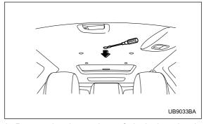
2. Remove the plug on the roof trim by inserting the end of the regular screwdriver between the roof and plug and prying it off.
