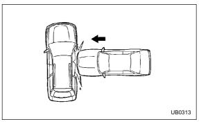
A severe side impact near the front seat activates the SRS side airbag.
