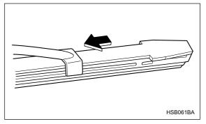
3. Align the claws of the metal support with the grooves in the rubber and slide the blade rubber assembly into the metal support until it locks.
