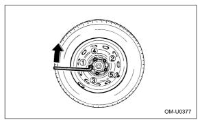
14.Use the wheel nut wrench to securely tighten the wheel nuts to the specified torque, following the tightening order in the illustration.
