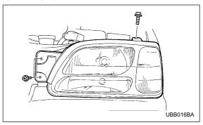
1. Remove the headlight assembly mounting screws located at the top of and the front of the headlight assembly using a phillips screwdriver or an open-end wrench.
