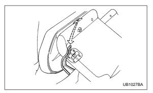
6. Unlock the seatback by pulling the release knob and fold the seatback down. Confirm that the pin located at the bottom of the seat cushion is inserted into the slot at the top of the seatback.
