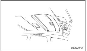
The front moonroof has a tilting function and the rear moonroof has a sliding function.
