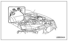
Check the level of the washer fluid at each fuel stop. If the level is low, fill the fluid up to the neck of the reservoir.
