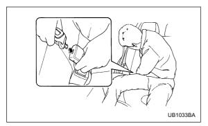
3. After confirming that the webbing is not twisted, insert the connector (tongue) attached at the webbing end into the buckle on the right-hand side until a click is heard. If the belt stops before reaching the buckle, return the belt slightly and pull it out more slowly. If the belt still cannot be unlocked, let the belt retract slightly after giving it a strong pull, then pull it out slowly again.
