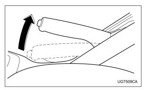
Check the parking brake stroke according to the maintenance schedule in the "Warranty and Maintenance Booklet". When the parking brake is properly adjusted, braking power is fully applied by pulling the lever up seven to eight notches gently but firmly (about 44 lbs, 196 N, 20 kg). If the parking brake lever stroke is not within the specified range, have the brake system checked and adjusted at your SUBARU dealer.
