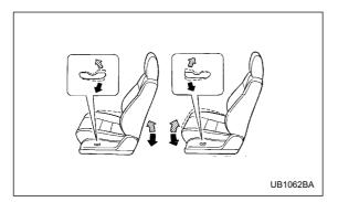
To adjust the angle and height of the seat cushion, move the control switch in the corresponding direction.
