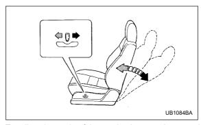
To adjust the angle of the seatback, move the control switch.
