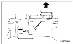
**Window-side seating positions:** Pull the headrest up while pressing the release button located on the backside of the seatback
