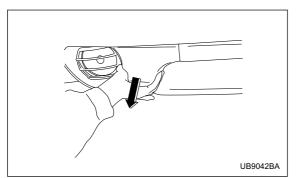
1. Squeeze the sides of portion  $\boldsymbol{\mathsf{A}}$  and pull the towing hook cover toward you.
