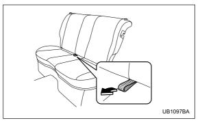
5. Raise the seat cushion by pulling up the tab. Make certain that the rear passenger's cup holder is fully retracted before raising the seat cushion.
