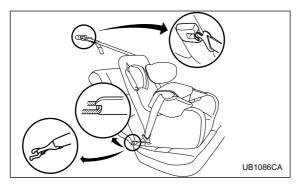
Your vehicle is equipped with four lower anchorages (bars) and three upper anchorages (tether anchorages) for accommodating such child restraint systems.
