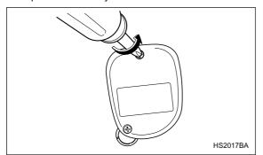
1. Remove the two screws on the back of the trans-
