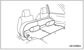
7. Install the headrests (if so equipped) onto the backside of the seatback (window-side positions only). To return the rear seat to its original position, raise the seatback and seat cushion until they lock into place and make sure that they are securely locked. Make sure that the rear seatbelts are not under the seat cushion or seatback.
