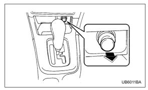
The electrical power socket located on the lower part of the instrument panel can be used as cigarette lighter socket. A cigarette lighter plug is an optional accessory. It is available from your SUBARU dealer. The cigarette lighter socket may also be used as a power source for an in-car use electrical appliance.
