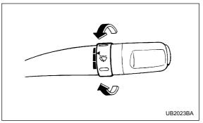
When the wiper switch is in the " $\nabla$ " position, turn the dial to adjust the operating interval of the wiper. The operating interval can be adjusted continuously from the shortest interval to the longest.
