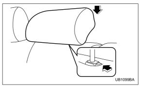
To raise the headrest, pull it up. To lower it, push the headrest down while pressing the release button on the top of the seatback.
