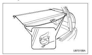
To extend the cover, pull the end of the cover out of the housing, then insert its hooks into the catches as shown. To rewind it, unhook it from the catches and it will rewind automatically. You should hold on to the cover and guide it back into the cover housing while it is rewinding.
