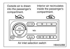
Select the air inlet by pushing the air inlet selection switch.
