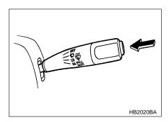
To wash the windshield, push the washer button at the end of the wip-
