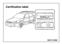
The certification label attached to the driver's side door shows GVWR (Gross Vehicle Weight Rating) and GAWR (Gross Axle Weight Rating).
