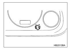
To set the time, turn the setting knob clockwise to advance and counterclockwise to retard the time. 3
