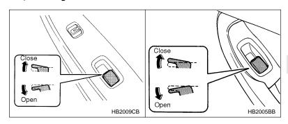
To open the window, push the switch down and hold it until the window reaches the desired position. To close the window, pull the switch up and hold it until the window reaches the desired position.
