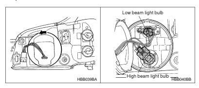
Remove the headlight bulb cover, by turning it counterclockwise.
