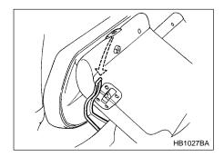
7. Install the headrests (if so equipped) onto the backside of the seat-back (window-side positions only).
