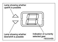
Lamps showing whether upshifting and downshifting are possible: The  $\triangle$  and  $\nabla$  lamps show whether upshifting and downshifting are possible. When both lamps are off, SPORTSHIFT operation is not possible. When both lamps are on, upshifting and downshifting are both possible. When only the  $\triangle$  lamp is on, only upshifting is possible. When only the  $\nabla$  lamp is on, only downshifting is possible.
