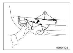
1. Ilnsert the projection  ${\bf C}$  into the hole  ${\bf D}$ .
