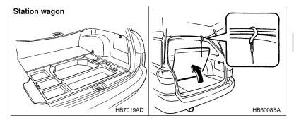
The subfloor storage is located under the floor of the trunk or cargo area and can be used to store small items. To open the lid, pull the tab or handle up.
