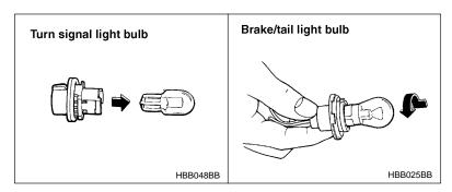
5. Remove the bulb from the socket.
