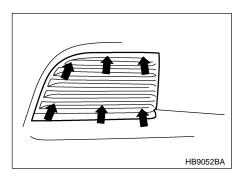
Align the towing hook cover with its original installation position and press all parts of it into place.
