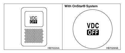
Note: Even when the lighting switch is turned to the "5065" or "\$\int 0"" position, the "OFF" portion of the symbol stamped on the switch will not illuminate in the dark. Only "VDC" portion will illuminate.
