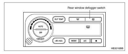
To turn on the defogger, push the switch. To turn it off, push the switch again.
