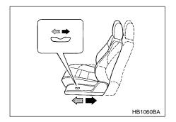
To adjust the seat forward or backward, move the control switch forward or backward.
