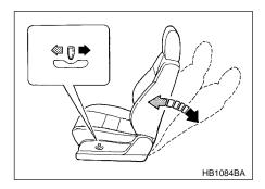
To adjust the angle of the seatback, move the control switch.
