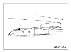
3. Insert the safety pin into the hitch pin securely.
