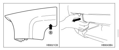
2. Press portion  $\boldsymbol{\mathsf{B}}$  and simultaneously pull the towing hook cover toward you.
