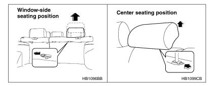
1. Remove the headrest (if so equipped) at the seating position where the child restraint system has been installed with the seatbelt or lower anchorages; lift up the headrest while pressing the release but-
