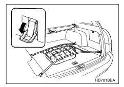
The cargo area is equipped with four tie-down hooks so that cargo can be secured with a luggage net or ropes.
