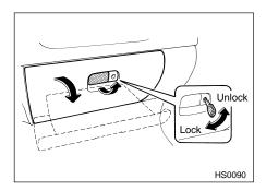
To open the glove box, pull the handle. To close it, push the lid firmly upward.
