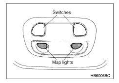
To turn on the map light, push the switch. To turn it off, push the switch again.
