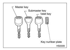
Three types of keys are provided for your vehicle. Master key, submaster key and valet key.
