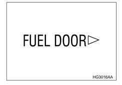
ullet You will see the "FUEL DOOR  $\triangleright$ " sign in the combination meter. This indicates that the fuel filler door (lid) is located on the right side of the vehicle.
