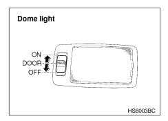
The dome light switch has three positions:
