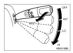
To turn the wipers on, push the wiper control lever down.
