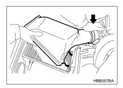
To install the air cleaner case cover, insert the two projections on the air cleaner case cover into the slits on the air cleaner case and then snap the two clamps on the air cleaner case cover.
