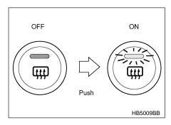
To turn on the defogger, push the switch. To turn it off, push the switch again.
