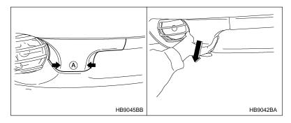
1. Squeeze the sides of portion  $\boldsymbol{\mathsf{A}}$  and pull the towing hook cover toward you.
