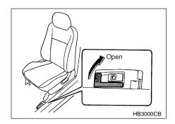
Pull the trunk lid release lever upward.
