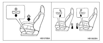
To adjust the angle and height of the seat cushion, move the control switch in the corresponding direction.
