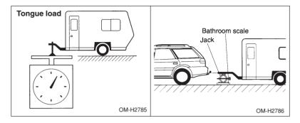
The tongue load can be adjusted by proper distribution of the load in the trailer. Never load the trailer with more weight in the back than in the front; approximately 60 percent of the trailer load should be in the front and approximately 40 percent in the rear. Also, distribute the load as evenly as possible on both the left and right sides.
