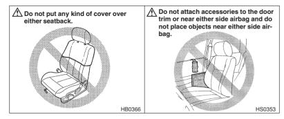
The SRS side airbag is stored in the door side of each front seatback. which bears an "SRS AIRBAG" label.
