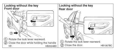
To lock the **front door** from the outside without the key, rotate the lock lever rearward and hold the outside door handle up while closing the door.
