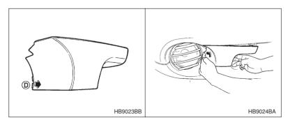
3. Push the portion **D**. Pull out the towing hook cover to remove it.
