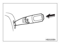
To wash the windshield, push the washer button at the end of the wip-
