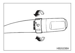
When the wiper switch is in the "\(\overline{\sigma}\)" position, turn the dial to adjust the operating interval of the wiper.
