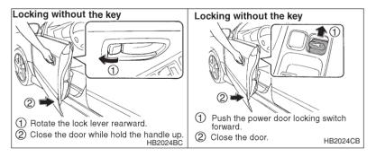
To lock the door from the outside without the key, rotate the lock lever rearward and then close the door.
