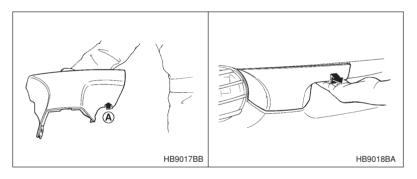
1. Pull the towing hook cover toward you while pushing up the portion  ${\bf A}$ . The portion  ${\bf B}$  will be raised.
