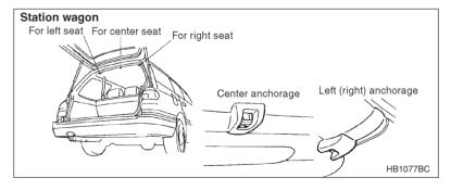
Three anchorages, i.e., ones for the right, center and left positions, are already installed on the rear shelf (on Sedan) or on the rear edge of the roof (on Staion wagon).
