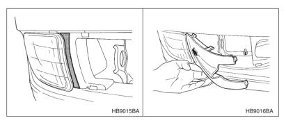
1. Insert the towing hook cover into the clearance between the fog light (or bumper trim cover) and the bumper body.
