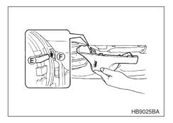
1. Insert the guide **E** into the hole **F**.
