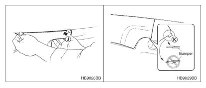
3. Push at the portion  ${\bf J}$ . Check that the tab of the portion  ${\bf K}$  is fitted in the bumper as shown in the illustration.
