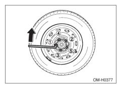
The torque for tightening the nuts is 58 to 72 ft-lb (78 to 98 N-m, 8 to 10 kg-m). This torque is equivalent to applying about 88 to 110 lbs (40 to 50 kg) at the top of the wheel nut wrench. Never use your foot on the wheel nut wrench or a pipe extension on the wrench because you may exceed the specified torque. Have the wheel nut torque checked at the nearest automotive service facility.
