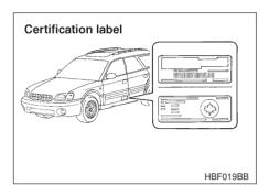
The certification label attached to the driver's side door shows GVWR (Gross Vehicle Weight Rating) and GAWR (Gross Axle Weight Rating).
