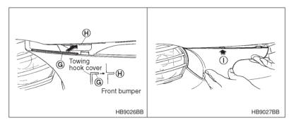
2. Fit the flange  ${\bf G}$  in the slit  ${\bf H}$  from the left end. While holding the towing hook cover at the portion  ${\bf G}$ , push at the portion  ${\bf I}$ .
