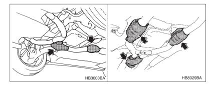
The catalytic converter is installed in the exhaust system. It serves as catalyst to reduce HC, CO and NOx in exhaust gases, thus providing cleaner exhaust.
