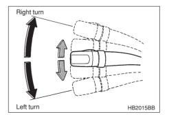
To activate the right turn signal, push the turn signal lever up. To activate the left turn signal, push the turn signal lever down. When the turn is fin-
