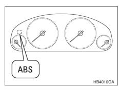
The ABS warning light comes on when the ignition switch is turned to the "ON" position and goes out after about two seconds.
