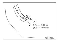
Stop the engine and firmly depress the brake pedal several times. Lightly press the brake pedal down with one finger to check the free play with a force of less than 2 lb (10 N, 1 kg).
