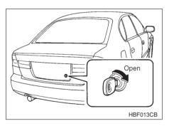
To open the trunk lid from outside, insert the key and turn it clockwise. To close the trunk lid, lightly press the trunk lid down until the latch engages.
