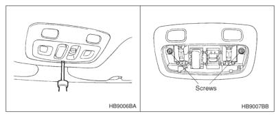
2. Remove the spot light lens by prying the edge of the lens with a regular screwdriver, then remove the switch body retaining screws and take off the moonroof switch.
