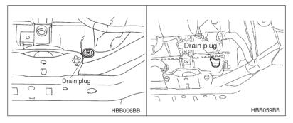
3. Loosen the radiator cap to drain the coolant from the radiator. Then drain the coolant from the reserve tank. Tighten the drain plug securely.
