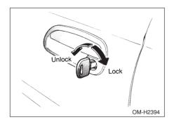
To lock the door from the outside with the key, turn the key toward the rear. To unlock the door, turn the key toward the front.
