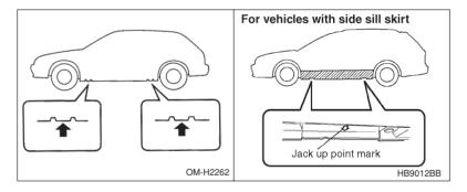
Turn the jackscrew by hand until the jack head engages firmly into the jack-up point.
