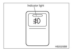
The indicator light located on the switch will illuminate when the fog lights are on.
