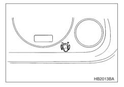
To set the time, turn the setting knob clockwise to advance and counterclockwise to retard the time.
