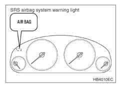
A diagnostic system continually monitors the readiness of the SRS airbag system (including front seatbelt pretensioners) while the vehicle is being driven. The SRS airbag system warning light "AIRBAG" will show normal system operation by lighting for about 6 seconds when the ignition key is turned to the "ON" position.
