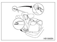
Your vehicle is equipped with four lower anchorages (bars) and three upper anchorages (tether anchorages) for accommodating such child restraint systems.
