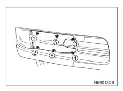
2. Push the towing hook cover in accordance with the pushing order given in the illustration.
