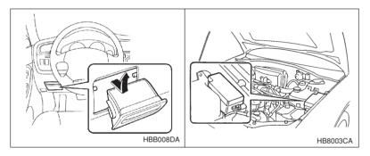
The fuses are designed to melt during an overload to prevent damage to the wiring harness and electrical equipment. The fuses are located in two fuse boxes. One is located under the instrument panel behind the coin tray on the driver's seat side. The other one is housed in the engine compartment. The fuse puller and spare fuses are stored in the main fuse box cover in the engine compartment.
