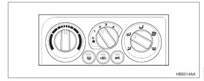
This setting allows you to direct air of different temperatures from the instrument panel and foot outlets. The air from the foot outlets is slightly warmer than from the instrument panel outlets.
