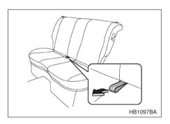
6. Unlock the seatback by pulling the release knob and fold the seatback down. Confirm that the pin located at the bottom of the seat cushion is inserted into the slot at the top of the seatback.
