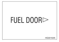
ullet You will see the "FUEL DOOR  $\triangleright$ " sign in the combination meter. This indicates that the fuel filler door (lid) is located on the right side of the vehicle.
