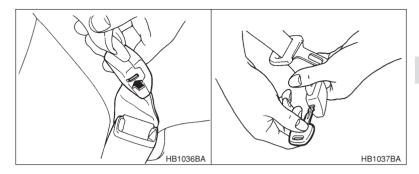
1. Insert a key or other hard pointed object into the slot in the connector (buckle) on the right-hand side and push it in, and the connector (tongue) plate will disconnect from the buckle.
