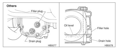
Remove the plug from the filler hole and check the oil level. The oil level should be kept even with the bottom of the filler hole. If the oil level is below the bottom edge of the hole, add oil through the filler hole to raise the level.
