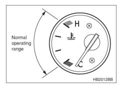
The temperature gauge shows engine coolant temperature when the ignition switch is in the "ON" position.
