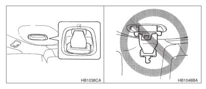
2. Allow the retractor to roll up the belt. You should hold the webbing end and guide it back into the retractor while it is rolling up. Neatly store the tongue plates in the recess in the retractor and then insert the connector (tongue) plate into the slot located at the front of the recess.
