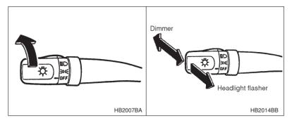
The light switch operates only when the ignition switch is in the "ON" position.
