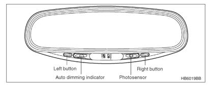
The inside electronic compass mirror has an anti-glare feature which automatically reduces glare coming from headlights of vehicles behind you. It also contains a built-in compass.
