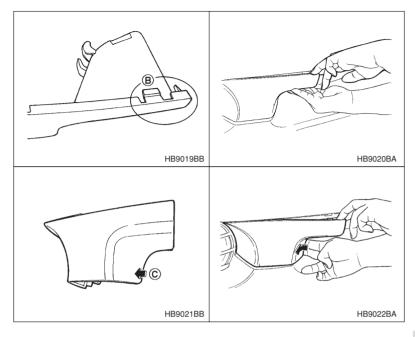
2. Pull the portion  ${\bf B}$  toward you with your left hand. Simultaneously pull the portion  ${\bf C}$  toward you while pushing the portion  ${\bf C}$  with your right hand.
