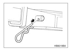
4. Pull the ball mount to make sure it does not come off the hitch receiver
