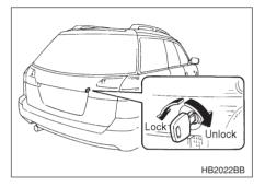
To unlock the rear gate, insert the key in the keyhole and turn it clockwise. To lock the rear gate, insert the key in the keyhole and turn it counterclockwise. If your vehicle is equipped with power door locking switches, the rear gate can also be locked and unlocked through use of the power door locking switches. Refer to "Power door locking switches" section in this chapter.
