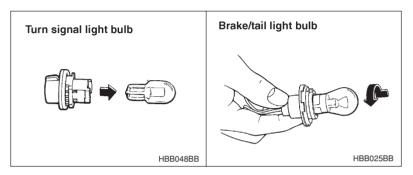
5. Remove the bulb from the socket.
