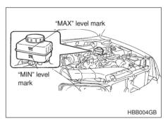
Check the fluid level on the outside of the reservoir. If the level is below "MIN", add the recommended brake fluid to "MAX". Use only brake fluid from a sealed container.
