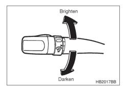
When the lighting switch is in the " $\stackrel{>}{>}$ 0 $\stackrel{<}{<}$ " or " $\stackrel{\blacksquare}{\equiv}$ D" position, you can adjust brightness of the instrument panel illumination for better visibility.
