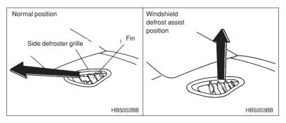
The driver's side defroster grille is adjustable. The normal position as shown in the diagram directs warm air to the side glass. When more rapid defrosting of the windshield is desired, the air flow can be directed temporarily toward the windshield to assist the windshield defroster. If this is done, the driver's side grille should always be returned to its normal position so that the warm air flow can then be used to defrost the driver's side window.
