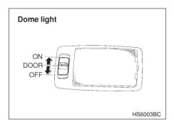
The dome light switch has three positions:
