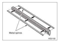
5. Align the claws of the metal support with the grooves in the rubber and slide the blade rubber assembly into the metal support until it locks. Be sure to position the claws at the end of the metal support between the stoppers on the rubber as shown. If the rubber is not retained properly, the wiper blade may scratch the windshield.
