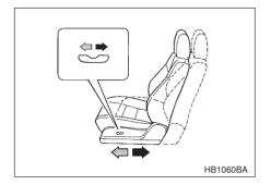
To adjust the seat forward or backward, move the control switch forward or backward.
