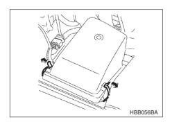
1. Unsnap the two clamps holding the air cleaner case cover.
