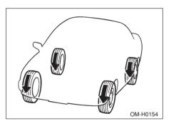
All wheel drive distributes the engine power to all four wheels. AWD vehicles provide better traction when driving on slippery, wet or snowcovered roads and when moving out of mud, dirt and sand. By shifting power between the front and rear wheels, SUBARU AWD can also provide added traction during acceleration, and added engine braking force during deceleration.
