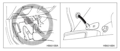
A retaining pin is located on the driver's side of the vehicle next to the fuel filler door release. The floor mat is secured using the built-in grommet, by placing the grommet over the pin and pushing downward.
