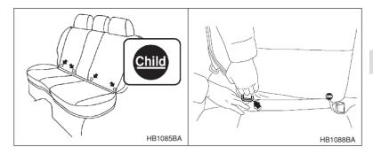
You will find marks "Child" at the bottom of the rear seat seatbacks. These marks indicate the positions of the lower anchorages (bars). Each lower anchorage is located where the seat cushion meets the seatback.
