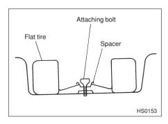
When storing a conventional tire, put the spacer upside down and tighten the attaching bolt firmly.
