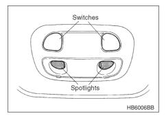
To turn on the spotlight, push the switch. To turn it off, push the switch again.
