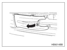
2. Insert your fingers under the raised portion **B**. Then, pull it toward you so that the towing hook cover may swing open. Remove the cover.
