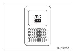
Note: Even when the lighting switch is turned to the "⋽໙ང" or "≣Ɗ" position, the "OFF" portion of the symbol stamped on the switch will not illuminate in the dark. Only "VDC" portion will illuminate.
