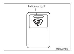
The windshield wiper deicer operates only when the ignition switch is in the "ON" position.
