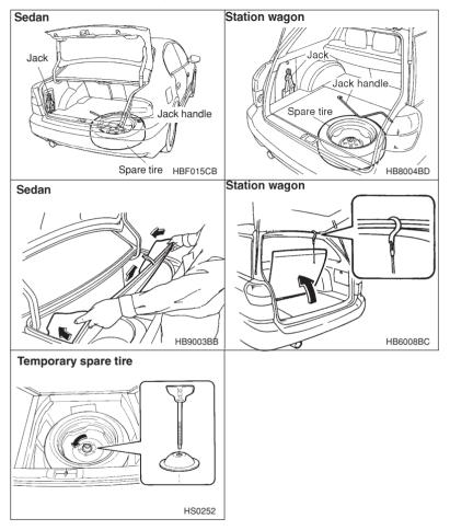
The spare tire is stored under the floor of the trunk or cargo area.
