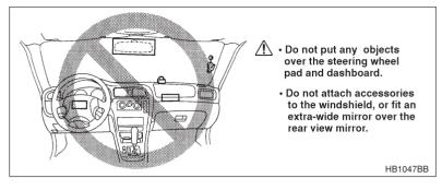
The driver's SRS frontal airbag is stowed in the center portion of the steering wheel. The passenger's SRS frontal airbag is stowed near the top of the dashboard under an "SRS AIRBAG" mark.
