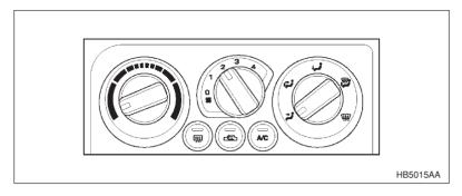
To force outside air through the instrument panel outlets:
