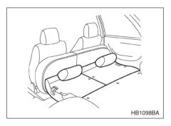
To return the rear seat to its original position, raise the seatback and seat cushion until they lock into place and make sure that they are securely locked.
