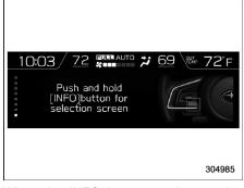
When the INFO button on the steering wheel is pressed and held on this screen, the setting screen can be displayed. For details, refer to "Setting screen" @ 3-
