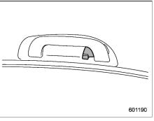
A coat hook is attached to the rear passenger's hand grip.
