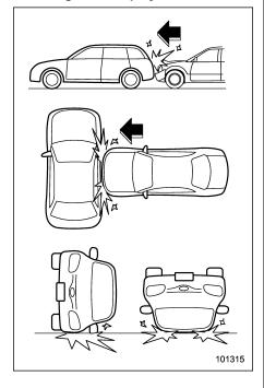
The driver's and front passenger's SRS frontal airbags are not designed to deploy in most of the following cases.
