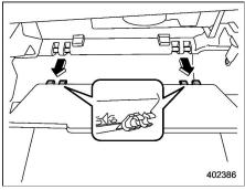
(4) Pull out the glove box horizontally and remove the hinge portion. When doing this, be careful not to damage the hinge.
