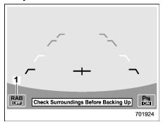
Reverse Automatic Braking system OFF indicator
