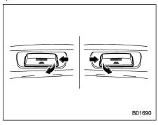
1. The license plate lights must be pushed outwards, and then pulled out to be removed.
