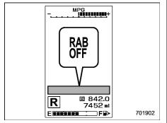
RAB OFF indicator: illuminates when the Reverse Automatic Braking system is turned OFF
