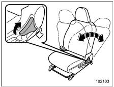
Pull the reclining lever up and adjust the seatback to the desired position. Then release the lever and make sure the seatback is securely locked into place.
