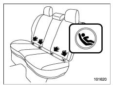
2. You will find marks "©" at the bottom of the rear seat seatbacks. These marks indicate the positions of the lower anchorages (bars).
