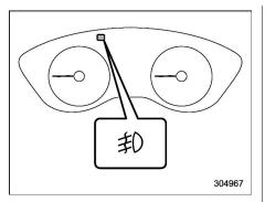
The indicator light on the combination meter will illuminate when the front fog lights are illuminated.
