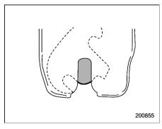
3. Pull the release handle upward and check that the latch is released.
