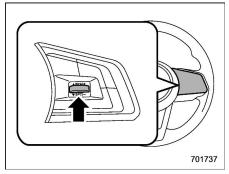
Press the "RES/SET" switch to the "RES" side and hold it until the vehicle reaches the desired speed. Then, release the switch. The vehicle speed at that moment will be memorized and treated as the new set speed.
