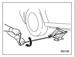
7. Insert the jack handle into the jackscrew, and turn the handle until the tire clears the ground. Do not raise the vehicle higher than necessary.
