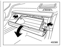
(3) Push in the stoppers located on both sides of the glove box and then pull down the glove box as far as it will qo.
