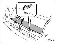
3. Put the cargo floor board back while hanging two retaining straps on the hooks that are located on the rear wall of cargo area.
