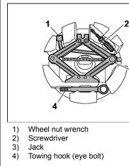
A jack handle is stored under the floor of the trunk (sedan) or the cargo area (5-door models). A jack and a towing hook are stored in the tool bucket that is located in the recess of the spare tire wheel.
