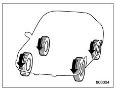
All-Wheel Drive distributes the engine power to all four wheels. AWD models provide better traction when driving on slippery, wet or snow-covered roads and when moving out of mud, dirt and sand. By shifting power between the front and rear wheels, SUBARU AWD can also provide added traction during acceleration and added engine braking force during deceleration.
