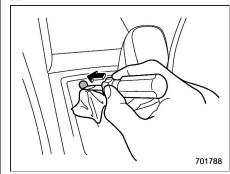
2. Wrap the tip of a flat-head screwdriver with vinyl tape or a cloth and use it to remove the shift lock cover. The shift lock release button is located under the shift lock cover.
