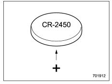
3. Remove the circuit board from the bottom half of the case and remove the battery and replace with new one. Be sure to observe the (+) sign on the old battery before removing it to ensure that the new battery is inserted properly (battery "+"
