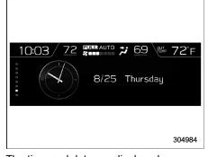
The time and date are displayed. You can adjust the time and date. For details, refer to "Clock" @ 3-63.
