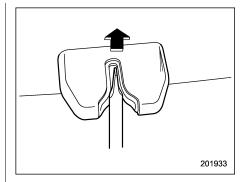
2. Use a flat-head screwdriver with a thin blade. Slide the flat-head screwdriver. blade from the slit aperture of the lock assembly fully to the end until you hear a click.
