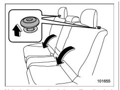
Unlock the seatback by pulling the lock release knob and then fold the seatback down.
