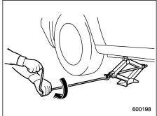
10. Insert the jack handle into the jackscrew, and turn the handle until the tire clears the ground. Do not raise the vehicle higher than necessary. 11. Remove the wheel nuts and the flat tire.
