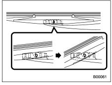
2. Turn the wiper blade assembly counterclockwise
