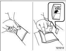
Remove the covers and locate the lower anchorages (bars).
