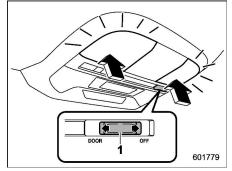
Door interlock switch To turn on the map light, push the switch. To turn it off, push the switch again.
