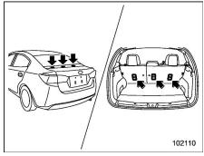
The tether anchorages (upper anchorages) are provided at the locations shown in the above illustration. For details, refer to "Top tether anchorages" \$\tilde{\text{\$\sigma}}\$1-38.
