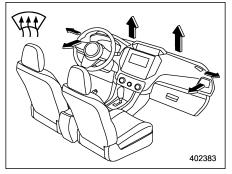
**(Defrost):** Windshield defroster outlets and both side outlets of the instrument panel (Refer to "Defrosting" \$\tilde{\text{\$\text{\$}}} 4-10.)\$
