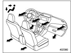
(Bi-level): Instrument panel outlets and foot outlets
