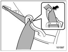
3. After drawing out the seatbelt, pass it through the belt guide as follows: First insert one edge of the belt into the open gap in the belt guide; then slide the rest of the belt in, so that the whole belt fits inside.
