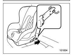
4. While following the instructions supplied by the child restraint system manufacturer, connect the lower hooks onto the lower anchorages located at "Q" marks on the bottom of the rear seatback. When the hooks are connected, make sure the
