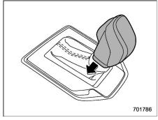
"L" is for using engine braking when going down a hill, etc. To select this mode, move the select lever from the "D" position to the "L" position.
