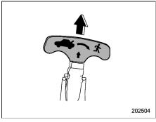
To open the trunk lid from inside the trunk, pull the trunk lid release handle upward as indicated by the arrow on the handle.
