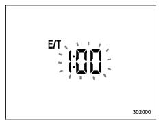
The journey time indication flashes each time a complete hour has elapsed. If the display is giving a reading other than the journey time, the display switches to the journey time, flashes for 5 seconds, and returns to its original reading each time a complete hour has elapsed.
