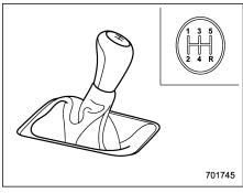
The manual transmission is a fully synchromeshed. 5-forward-speed and 1-reverse-speed transmission.
