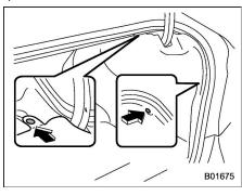
1. Remove the clips from the trunk trim with a flat-head screwdriver.
