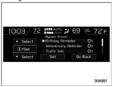
2. Select "On" or "Off" to turn the display of items on or off by using the control switches.
