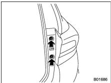
2. Using a Phillips screwdriver, remove the upper and lower screws that secure the rear combination light assembly.
