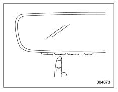
7. Return to the vehicle and firmly press, hold for two seconds and release the HomeLink button up to three times. At this point programming is complete and your device should operate when the HomeLink button is pressed and released.
