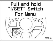
While this screen is selected, pull and hold the "I/SET" switch to enter the menu screen.
