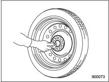
12. Before putting the spare tire on, clean the mounting surface of the wheel and hub with a cloth.
