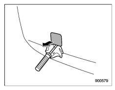
2. Cover the tip of a flat-head screwdriver with vinvl tape or cloth so that it will not scratch the bumper. Pry off the cover on the rear bumper using a screwdriver, and you will find a threaded hole for attaching the towing hook.
