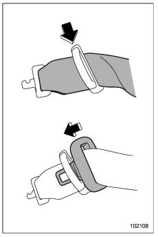
3. Allow the retractor to roll up the belt. You should hold the webbing end and guide it back into the retractor while it is rolling up. Insert the connector (tongue) into the belt holder.
