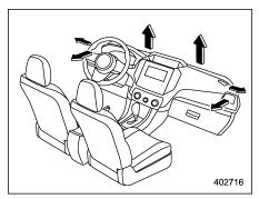
Select the "w" or "" mode to defrost or dehumidify the windshield and front door windows.
