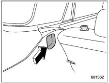
2. Insert both ends of the cover housing into the recesses of the retainers.
