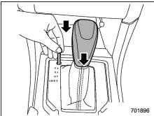
4. While depressing the brake pedal, insert a screwdriver into the hole, move it right and left while pushing the shift lock release button using a screwdriver, and then move the select lever.
