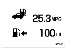
: Current fuel consumption □ ←: Driving range on remaining fuel
