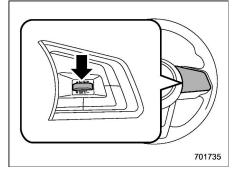
2. Press the "RES/SET" switch to the "SET" side once. Now the desired speed is set and the vehicle will keep running at that speed without depressing the accelerator pedal.
