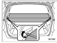
To extend the cover, pull the end of the cover out of the housing, then insert its hooks into the catches as shown. To rewind it, unhook it from the catches and it will rewind automatically. You should hold on to the cover and quide it back into the cover housing while it is rewinding.
