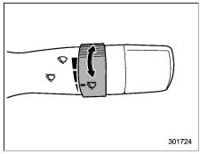
When the wiper switch is in the "\overline{\sigma}" position, turn the dial to adjust the operating interval of the wiper. The operating interval can be adjusted in several steps.
