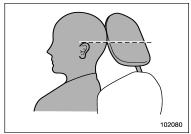
Each head restraint should be adjusted so that the center of the head restraint is closest to the top of the occupant's ears.
