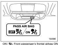
off / №2: Front passenger's frontal airbag OFF indicator
