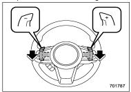
To upshift to the next higher gear position, pull the shift paddle that has "+" indicated on it. To downshift to the next lower gear position, pull the shift paddle that has "-" indicated on it.
