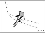
2. Cover the tip of a flat-head screwdriver with vinyl tape or cloth so that it will not scratch the bumper. Pry off the cover on the rear bumper using a screwdriver, and you will find a threaded hole for attaching the towing hook.
