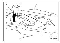
Check the parking brake stroke according to the maintenance schedule in the "Warranty and Maintenance Booklet". When the parking brake is properly adjusted, braking power is fully applied by pulling the lever up 7 to 8 notches gently but firmly (approximately 45 lbf [200 N, 20.4 kgf]). If the parking brake lever stroke is not within the specified range, have the brake system checked and adjusted at your SUBARU dealer.
