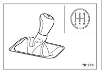
The manual transmission is a fully synchromeshed. 5-forward-speed and 1-reverse-speed transmission.
