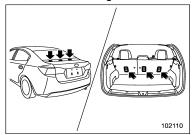
The tether anchorages (upper anchorages) are provided at the locations shown in the above illustration. For details, refer to "Top tether anchorages" #1-36.
