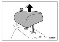
1. Raise the head restraint to the extended position. Do not remove the head restraint.
