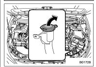
Remove the washer tank filler cap, then add windshield washer fluid
