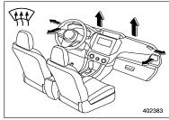
(Defrost): Windshield defroster outlets and both side outlets of the instrument panel (Refer to "Defrosting" #4-10.)
