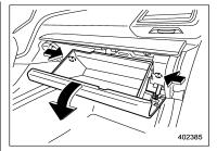
(3) Push in the stoppers located on both sides of the glove box and then pull down the glove box as far as it will go.
