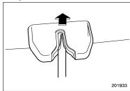
2. Use a flat-head screwdriver with a thin blade. Slide the flat-head screwdriver blade from the slit aperture of the lock
