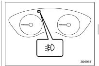
The indicator light on the combination meter will illuminate when the front foa lights are illuminated.
