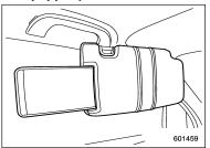
With the sun visor positioned over the side window, you can use the sun visor extension plate to prevent glare through the gap between the sun visor and center pillar. To use the extension plate, pull it toward the rear of the vehicle. When you have finished using it, stow it by pushing it toward the front of the vehicle.
