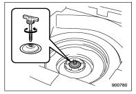
6. Take out the tool bucket and turn the attaching bolt counterclockwise, then take the spare tire out.
