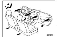
(Ventilation 2 for type B and C): Instrument panel outlets and foot outlets
