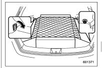
The cargo area is equipped with four tiedown hooks so that cargo can be secured with a cargo net or ropes.
