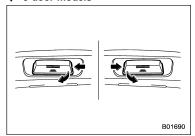
1. The license plate lights must be pushed outwards, and then pulled out to be removed.
