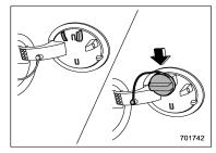
4. Set the fuel filler cap on the cap holder inside the fuel filler lid.
