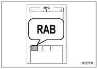
If the Reverse Automatic Braking System malfunctions, the above indicator illuminates on the combination meter. Contact the nearest SUBARU dealer for details.
