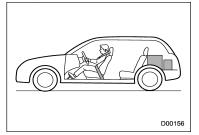
Vehicle capacity weight of the vehicle is 900 lbs (408 kg), which is indicated on the vehicle placard with the statement "The combined weight of occupants and cargo should never exceed 900 lbs or 408 kg".
