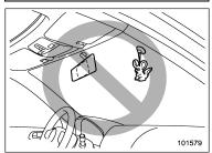
Do not attach accessories to the windshield, or fit an extra-wide mirror over the inside rear view mirror. If the SRS airbag deploys, those objects could become projectiles that could seriously injure vehicle occupants.
