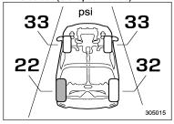
This screen displays each tire pressure. When a tire is deflated, the deflated tire and the tire pressure will be displayed on the screen in yellow.
