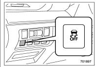
Press the Vehicle Dynamics Control OFF switch to deactivate the Vehicle Dynamics Control system. Creating adequate driving wheel slip by deactivating the Vehicle Dynamics Control system may help to recover from the loss of traction. Use the Vehicle Dynamics Control OFF switch as necessary.
