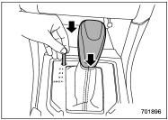
4. While depressing the brake pedal, insert a screwdriver into the hole, move it right and left while pushing the shift lock release button using a screwdriver, and then move the select lever
