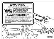
Your vehicle has warning labels on the driver's and front passenger's sun visors
