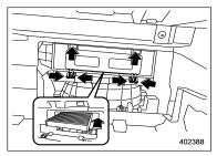
3. Replace the cabin air filter with a new one and then reinstall the cover.
