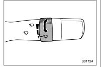
When the wiper switch is in the "position, turn the dial to adjust the operating interval of the wiper. The operating interval can be adjusted in several steps from the shortest interval to the longest.
