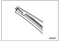
Securely retain both ends of the rubber with the stoppers on the plastic support
