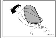
The angle of the head restraint can be adjusted in several steps. While maintaining a suitable driving posture, adjust the head restraint to a position where the back of your head is as close to the head restraint as possible.
