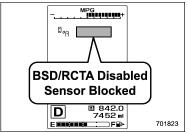
System temporary stop indicator due to reduced radar sensitivity
