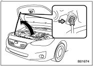
4. Lift up the hood, release the hood prop from its retainer and put the end of the hood prop into the slot in the hood.
