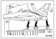
5. To install the air cleaner case (rear), insert the three projections on the air
