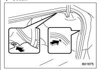
1. Remove the clips from the trunk trim with a flat-head screwdriver.
