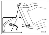
Retaining pins are located on the driver's side floor.
