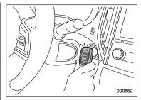
5. Hold the access key fob with the buttons facing you, and touch the pushbutton ignition switch with it.
