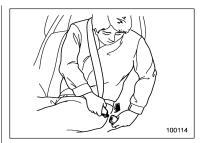
5. Insert the center seatbelt tongue plate into the center seatbelt buckle until it clicks.
