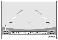
Reverse Automatic Braking system OFF indicator
