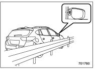
The BSD/RCTA approach indicator light may illuminate when driving close to solid objects on the road or road side (such as guardrails, tunnels and sidewalls).
