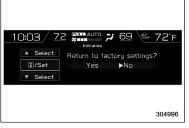
2. Select "Yes" or "No" by using the control switches.
