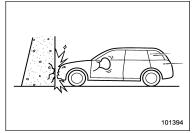
A head-on collision against a thick concrete wall at a vehicle speed of 12 to 19 mph (20 to 30 km/h) or higher activates only the driver's SRS frontal airbag or both driver's and front passenger's SRS frontal
