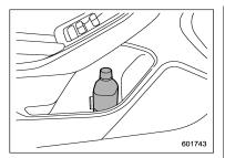
The bottle holder equipped on each door trim can be used to hold beverage bottles and other items.
