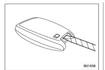
2. Wrap a flat-head screwdriver with vinyl tape or a cloth, and insert it in the gap to remove the cover.
