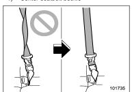
Fastening the seatbelt with the webbing twisted can increase the risk or severity of injury in an accident. When fastening the belt after it is pulled out from the retractor, especially when inserting the connector's tongue plate into the mating buckle (on right-hand side), always check that the webbing is not twisted.
