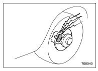
The disc brakes have audible wear indicators on the brake pads. If the brake pads wear close to their service limit, the wear indicator makes a very audible scraping noise when the brake pedal is applied.
