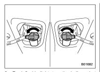
3. For left side light, turn the bulb socket clockwise and remove it.
