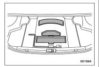
The storage compartments are located under the floor of the trunk. They can be used to store small items.
