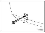
Screw the towing hook into the thread hole until its thread can no longer be seen.
