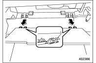
(4) Pull out the glove box horizontally and remove the hinge portion. When
