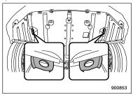
The front tie-down hooks are located between each of the front tires and the front bumper.
