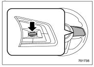
2. Press the "RES/SET" switch to the "SET" side once. Now the desired speed is set and the vehicle will keep running at that speed without depressing the accelerator pedal.
