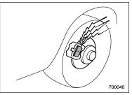
The disc brake pad wear warning indicators on the disc brakes give a warning noise when the brake pads are worn. If a squeaking or scraping noise is heard from the disc brakes while braking, immediately have your vehicle checked by your SUBARU dealer.
