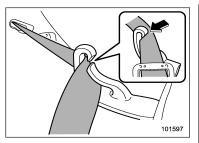
After drawing out the seatbelt, pass it through the belt guide as follows: First insert one edge of the belt into the open gap in the belt guide; then slide the rest of the belt in, so that the whole belt fits inside.
