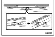
2. Turn the wiper blade assembly counterclockwise.
