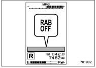
RAB OFF indicator: illuminates when the Reverse Automatic Braking system is turned OFF.
