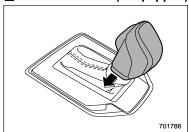
"L" is for using engine braking when going down a hill, etc. To select this mode, move the select lever from the "D" position to the "L" position.
