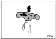
To open the trunk lid from inside the trunk, pull the trunk lid release handle upward as indicated by the arrow on the handle.
