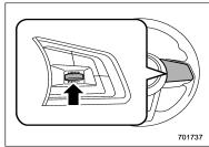
To resume the cruise control after it has been temporarily canceled and with vehicle speed of approximately 20 mph (30 km/h) or more, press the "RES/SET"
