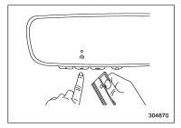
3. While the HomeLink indicator light is flashing orange, press and hold the handheld remote button. Continue pressing the hand-held remote button until the HomeLink indicator light changes from orange to green. You may now release the hand-held remote button.
