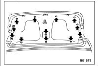
2. Remove the trunk trim lining by removing the clips indicated in the illustration.
