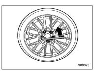
8. Loosen the wheel nuts using the wheel nut wrench but do not remove the nuts.
