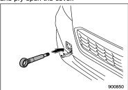
3. Screw the towing hook into the thread
