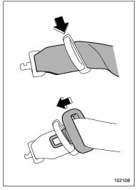
3. Allow the retractor to roll up the belt. You should hold the webbing end and guide it back into the retractor while it is rolling up. Insert the connector (tongue) into the belt holder.
