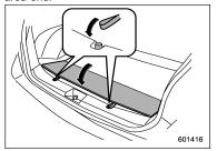
3. Put the cargo floor board back while hanging two retaining straps on the hooks that are located on the rear wall of cargo area.
