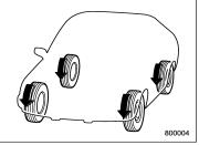
All-Wheel Drive distributes the engine power to all four wheels. AWD models provide better traction when driving on slippery, wet or snow-covered roads and when moving out of mud, dirt and sand. By shifting power between the front and rear wheels, SUBARU AWD can also provide added traction during acceleration and added engine braking force during deceleration.
