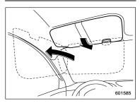
To block out glare, swing down the visors. To use the sun visor at a side window, swing it down and move it sideways.
