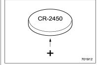
3. Remove the circuit board from the bottom half of the case and remove the battery and replace with new one. Be sure to observe the (+) sign on the old battery before removing it to ensure that the new battery is inserted properly (battery "+"
