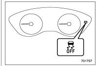
When the switch is pressed during engine operation, the Vehicle Dynamics Control OFF indicator light "#" on the combination meter illuminates. The Vehicle Dynamics Control system will be deactivated and the vehicle will behave like a model not equipped with the Vehicle Dynamics Control system. When the switch is pressed again to reactivate the Vehicle Dynamics Control system, the Vehicle Dynamics Control OFF indicator light turns off.
