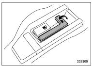
Pull the trunk lid release lever upward. The lever is on the floor at the left of the driver's seat.
