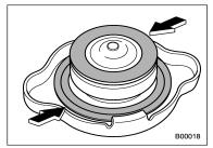
After refilling the reserve tank and the radiator, reinstall the cap and check that the rubber gaskets inside the radiator cap are in the proper position.
