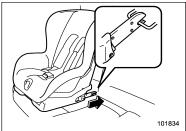
4. While following the instructions supplied by the child restraint system manufacturer, connect the lower hooks onto the lower anchorages located at "@" marks on the bottom of the rear seatback. When the hooks are connected, make sure the adjacent seatbelts are not caught.
