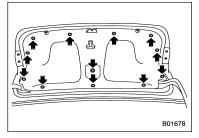
1. Open the trunk and remove the clips from the trunk lid trim with a flat-head screwdriver.
