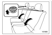
Unlock the seatback by pulling the lock release knob and then fold the seatback down.
