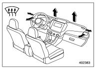
Select the "\(\overline{\pi}\)" or "\(\overline{\pi}\)" mode to defrost or dehumidify the windshield and front door windows.
