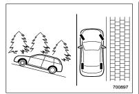
When parking on a hill, always turn the steering wheel. When the vehicle is headed up the hill, the front wheels should be turned away from the curb.
