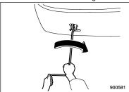
4. Tighten the towing hook securely using the jack handle.
