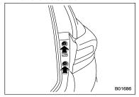
2. Using a Phillips screwdriver, remove the upper and lower screws that secure
