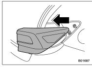
3. Slide the rear combination light assembly rearward and remove it from the vehicle.
