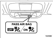
ON / 💸: Front passenger's frontal airbag ON indicator
