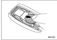
4. Insert a new battery with its positive (+) side facing upward as shown in the figure.
