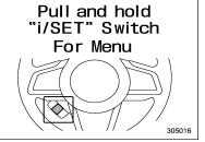
While this screen is selected, pull and hold the "[i]/SET" switch to enter the menu screen.
