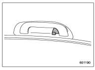
A coat hook is attached to the rear passenger's hand grip.
