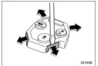
3. Open the transmitter case by releasing the hooks.
