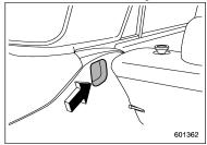
2. Insert both ends of the cover housing into the recesses of the retainers.
