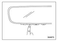
7. Return to the vehicle and firmly press, hold for two seconds and release the HomeLink button up to three times. At this point programming is complete and your device should operate when the HomeLink button is pressed and released.
