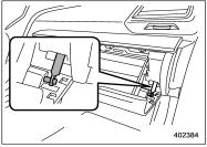
(2) Remove the damper shaft from the glove box.
