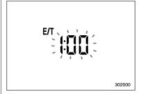
The journey time indication flashes each time a complete hour has elapsed. If the display is giving a reading other than the iourney time, the display switches to the iourney time, flashes for 5 seconds, and returns to its original reading each time a complete hour has elapsed.
