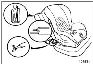
Some types of child restraint systems can be installed on the rear seat of your vehicle without use of the seatbelts. Such child restraint systems are secured to the designated anchorages provided on the vehicle body. The lower and tether anchorages are sometimes referred to as the LATCH system (Lower Anchors and Tethers for CHildren).
