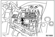
The fuse puller is stored in the main fuse
