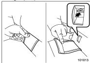
Remove the covers and locate the lower anchorages (bars).
