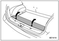
1. Raise and fold the rear end of the cargo floor board.
