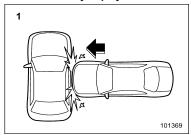
1) A severe side impact near the front seat.
