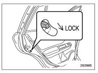
Each rear door has a child safety lock. When the child safety lock lever is in the lock position, the door cannot be opened from inside. The door can only be opened from the outside.
