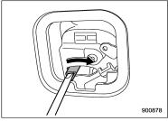
3. To open the rear gate, turn the lever to the right position using a flat-head screw-driver or a similar tool.
