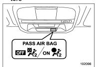
ON 3: Front passenger's frontal airbag ON indicator
