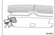
1. Apply a flat-head screwdriver to the light cover as shown in the illustration, and pry the light cover off from the rear gate trim.
