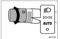
To turn on the headlights, turn the knob on the end of the turn signal lever.
