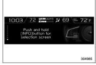
When the INFO button on the steering wheel is pressed and held on this screen, the setting screen can be displayed. For details, refer to "Setting screen" \$\tilde{x}^3-58.
