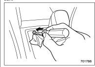
Wrap the tip of a flat-head screwdriver with vinyl tape or a cloth and use it to remove the shift lock cover. The shift lock release button is located under the shift lock cover
