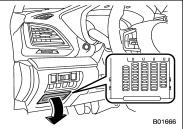
One is located under the instrument panel behind the fuse box cover on the driver's seat side. To remove the cover, pull it out.
