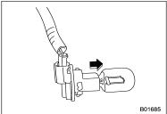
3. Pull the bulb out of the bulb socket and replace it with a new one.
