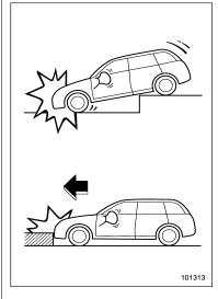
Only the driver's SRS frontal airbag or both driver's and front passenger's SRS frontal airbags may be activated when the vehicle sustains a hard impact in the undercarriage area from the road surface (such as when the vehicle plunges into a deep ditch, is severely impacted or knocked hard against an obstacle on the road such as a curb).
