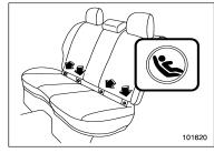
2. You will find marks "a" at the bottom of the rear seat seatbacks. These marks indicate the positions of the lower anchorages (bars).
