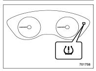
The tire pressure monitoring system provides the driver with a warning message when tire pressure is severely low.
