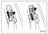
The shoulder belt anchor height should be adjusted to the position best suited for the driver/front passenger. Always adjust the anchor height so that the shoulder belt passes over the middle of the shoulder without touching the neck.
