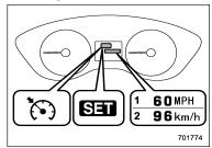
Cruise control set indicator light (type A) When setting the displayed unit as "MPH".
