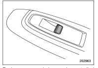
Each passenger window can be controlled by the power window switch located on the door.
