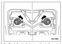
2. For left side light, turn the bulb socket clockwise and remove it.
