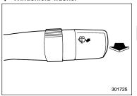
To wash the windshield, pull the wiper control lever toward you. The washer fluid sprays until you release the lever. The wipers operate while you pull the lever.
