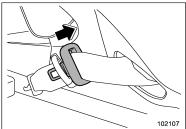
2. Remove the tongue plate from the belt holder on the right side of the cargo area and pull out the seatbelt slowly.
