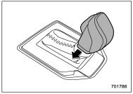
With the vehicle either moving or stationary, move the select lever from the "D" position to the "M" position to select the manual mode
