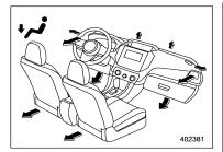
(Heat): Foot outlets, both side outlets of the instrument panel and some through windshield defroster outlets (A small amount of air flows to the windshield and both side windows to prevent fogging.)
