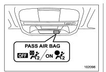
ON / : Front passenger's frontal airbag ON indicator
