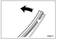
1. Pull out the end of the blade rubber assembly to unlock it from the plastic support.
