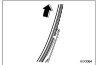
2. Pull the blade rubber assembly out of the plastic support.
