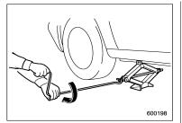
Insert the jack handle into the jackscrew, and turn the handle until the tire clears the ground. Do not raise the vehicle higher than necessary.
