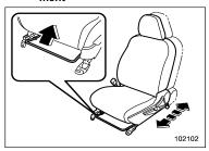
Pull the lever upward and slide the seat to the desired position. Then release the lever and try to move the seat back and forth to make sure that it is securely locked into place.
