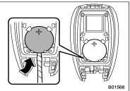
3. Take out the battery using a flat-head screwdriver with vinyl tape or a cloth.
