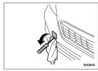
Cover the tip of a flat-head screwdriver with vinyl tape or cloth so that it will not scratch the bumper. Insert the flat-head screwdriver into the cutout of the cover and pry open the cover.
