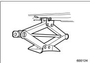
Turn the jackscrew by hand until the jack head engages firmly into the jack-up point.
