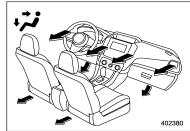
(Bi-level): Instrument panel outlets and foot outlets
