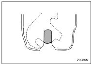
3. Pull the release handle upward and check that the latch is released.
