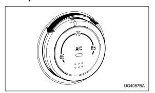
This dial is used to set the desired interior temperature. With the dial set to your desired temperature, the system automatically adjusts the temperature of air supplied from the outlets such that the desired temperature is achieved and maintained. If the dial is turned fully counterclockwise, the system gives maximum cooling performance. If the dial is turned fully clockwise, the system gives maximum heating performance.
