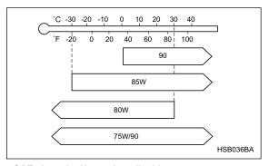
SAE viscosity No. and applicable temperature
