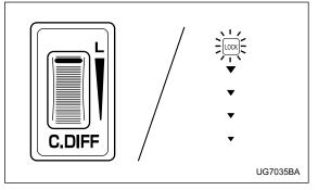
Turn the dial forward to increase the differential-action limiting factor. If the white line on the dial reaches the frontmost position, the center differential will be almost completely locked and the "LOCK" indicator light will come on.
