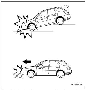
The SRS frontal airbag may be activated when the vehicle sustains a hard impact in the undercarriage area from the road surface (such as when the vehicle
