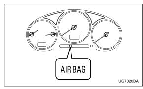
A diagnostic system continually monitors the readiness of the SRS airbag system while the vehicle is being driven. The SRS airbag system warning light "AIR-BAG" will show normal system operation by lighting for about 6 seconds when the ignition key is turned to the "ON" position.
