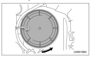
1. Remove the bulb cover, by turning it counterclockwise.
