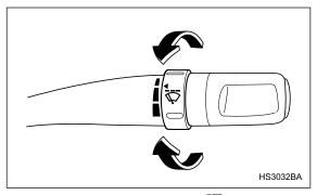
When the wiper switch is in the " \( \overline{\times} \) " position, turn the dial to adjust the operating interval of the wiper.
