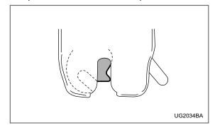
Move the release handle, from outside the vehicle, in the direction of the arrow to check if the latch is released.
