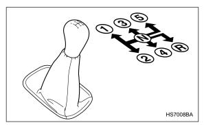
The manual transmission is a fully synchromeshed, 5-forward-speed and 1-reverse-speed transmission. The shift pattern is shown on the shift lever knob. When shifting from 5th gear to reverse gear, first return the shift lever to the neutral position then shift into reverse gear.
