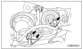
1. Remove two bolts and disconnect connectors.
