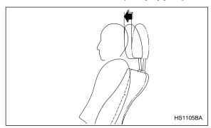
The front seats of your vehicle are equipped with active head restraints. They automatically tilt forward slightly in the event the vehicle is struck from the rear, decreasing the amount of rearward head movement and thus reducing the risk of whiplash. For maximum effectiveness the head restraint should be adjust so that the center of the head restraint is closest to the top of the occupant's ears.
