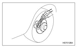
The disc brake pad wear warning indicators on the disc brakes give a warning noise when the brake pads are worn.
