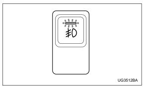
The fog lights operate only when the headlights are on low beam. Push the fog light button to turn the fog lights on.
