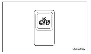
Water is sprayed for approximately two seconds every time the switch is pressed and then released.
