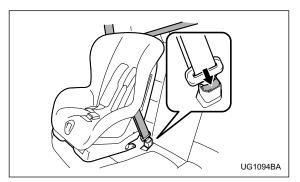
9. To remove the child restraint system, press the release button on the seatbelt buckle and allow the belt to retract completely. The belt will return to the ELR mode.
