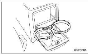
A dual cup holder is located at the back of the center console. To use the cup holder, open the lid by pulling its upper edge.
