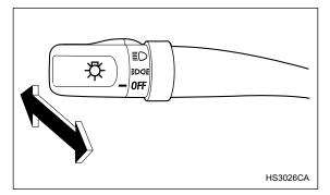
To change from low beam to high beam, push the turn signal lever forward. When the headlights are on high beam, the high beam indicator light "
