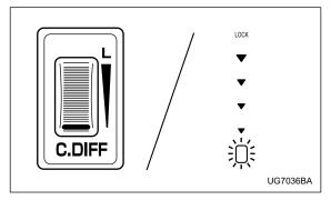
Turn the dial rearward to reduce the differential-action limiting factor. If the white line on the dial reaches the rearmost position, the factor will be minimal and the " " indicator light will come on.
