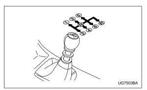
The manual transmission is a fully synchromeshed, 6-forward-speed and 1-reverse-speed transmission. The shift pattern is shown on the shift lever knob.
