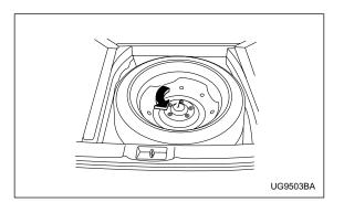
**Sedan:** Remove the floor cover from the trunk. Remove the storage compartment (if so equipped). Turn the attaching bolt counterclockwise, then take the spare tire out.
