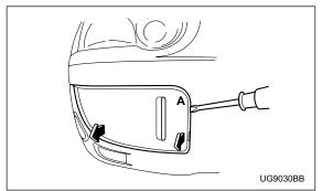
2. Insert a flat-head screwdriver into the slot at point A on the front passenger side fog light cover, then use it to pry the cover upward. The tabs at point A on the fog
