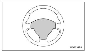
To sound the horn, push the horn pad.
