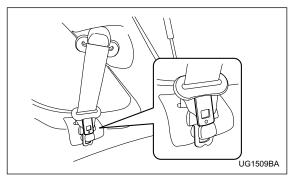
2. Allow the retractor to roll up the belt. You should hold the webbing end and guide it back into the retractor while it is rolling up. Insert the tongue plate into the belt holder.
