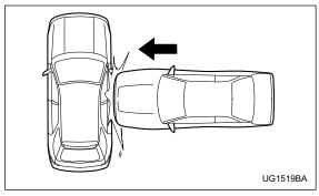
A severe side impact near the front seat activates the SRS side airbag.
