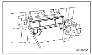
2. Unhook the hooks of the air filter cover and remove the cover.
