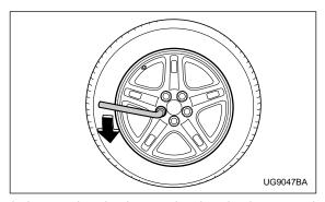
6. Loosen the wheel nuts using the wheel nut wrench but do not remove the nuts.
