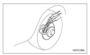
The right front disc brake and the right rear disc brake have an audible wear indicators on the brake pads. If the brake pads wear close to their service limit, the wear indicator makes a very audible scraping noise when the brake pedal is applied.
