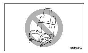
Do not put any kind of cover or clothes or other objects over either front seatback and do not attach labels or stickers to the front seat surface on or near the SRS side airbag. They could prevent proper deployment of the SRS side airbag, reducing protection available to the front seat's occupant.
