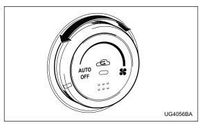
The fan operates only with the ignition switch in the ON position. The fan speed control dial is used to select the AUTO (automatic control) mode or to select the desired fan speed. The dial's positions and their functions are as follows:
