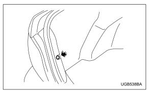
1. Remove the clip from the rear trunk trim with a screwdriver.
