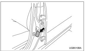
The load capacity of your vehicle is determined by weight, not by available cargo space. The maximum load you can carry in your vehicle is shown on the vehicle placard attached to the driver's side door pillar. It includes the total weight of driver and all passengers and their belongings, any optional equipment such as a trailer hitch, roof rack or bike carrier, etc., and the tongue load of a trailer.
