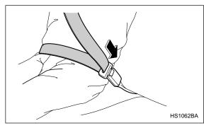
Push the release button of the center seatbelt buckle (on the left hand side) to unfasten the seatbelt.
