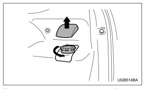
The tank is located on the right hand side of the trunk.
