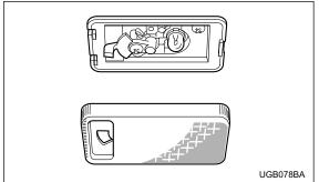
1. Remove the lens by prying the edge of the lens with
