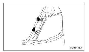
2. Remove the upper and lower screws. Then, slide the rear combination lamp assembly to the rear and remove it from the vehicle.
