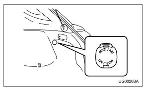
Accessory power outlet is provided in the cargo area (if equipped).
