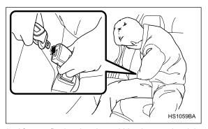
3. After confirming that the webbing is not twisted, insert the connector (tongue) attached at the webbing end into the buckle on the right hand side until a click is heard.
