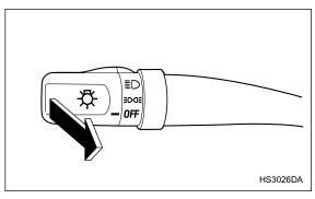
To flash the headlights, pull the lever toward you and then release it. The high beam will stay on for as long as you hold the lever. The headlight flasher works even though the lighting switch is in the "OFF" position.
