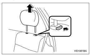
1. Remove the headrest at the window-side seating position where the child restraint system has been installed with the lower anchorages or seatbelt; lift up the headrest while pressing the release button. Store the headrest in the cargo area. Avoid placing the headrest in the passenger compartment to prevent it from being thrown around in the passenger compartment in a sudden stop or a sharp turn.
