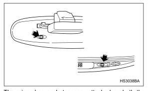
The mirror has a photosensor attached on both the front and back sides. If the glare from the headlights of vehicles behind you strikes the mirror, these sensors
