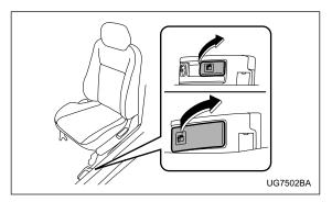
To open the fuel filler lid, pull the lid release lever up.
