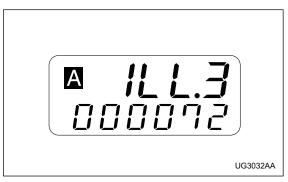
The brightness of the combination meter can be adjusted in five steps with the headlight switch either the OFF position or the " <sub>■DOE</sub> " or " <u>■</u>○ " position.
