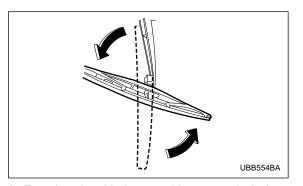
2. Turn the wiper blade assembly counterclockwise.
