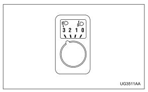
The WRX-STi version has High-Intensity Discharge (HID) headlights on the low beam setting. The HID headlights generate more light than conventional halogen headlights. Therefore a driver of an oncoming vehicle may experience too much glare when your headlight beam height adjustment is high due to the vehicle carrying heavy load.
