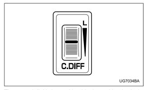
The control dial is located beside the parking-brake lever. By turning the control dial forward and rearward, it is possible to change the differential-action limiting factor of the center differential.
