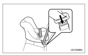
8. To remove the child restraint system, press the release button on the seatbelt buckle and allow the belt to retract completely. The belt will return to the ELR mode.
