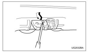
2. Use a screwdriver with a thin blade. Slide the screwdriver blade from the slit aperture of the lock assembly fully to the end until you hear a click.
