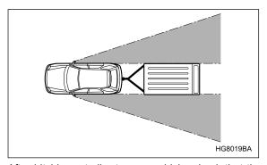
After hitching a trailer to your vehicle, check that the standard side mirrors provide a good rearward field of view without significant blind spots. If significant blind spots occur with the vehicle's standard side mirrors,
