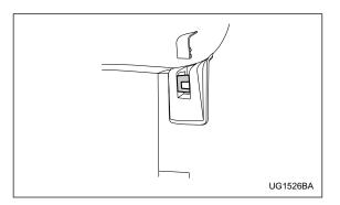
2. (For both window-side seating positions) Remove the cap from the anchor fitting cover by prying it with a screwdriver.
