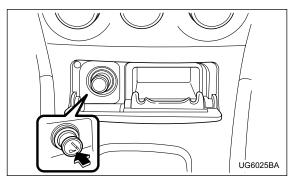
The cigarette lighter operates only when the ignition switch is in the "ON" and "ACC" positions.
