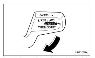
Push the control lever downward in the "SET/ COAST" direction and release it. Then release the accelerator pedal.
