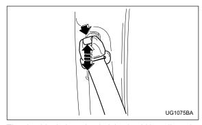
The shoulder belt anchor height should be adjusted to the position best suited for you. To adjust the anchor height, push the release button and slide the anchor up or down. Pull down on the anchor to make sure that it is locked in place.
