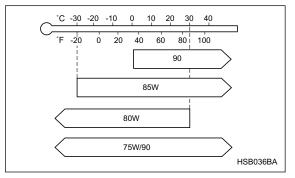
SAE viscosity No. and applicable temperature
