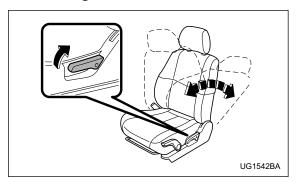
Pull the reclining lever up and adjust the seatback to the desired position. Then release the lever and make sure the seatback is securely locked into place.
