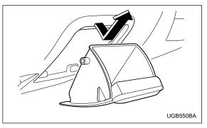
To remove the coin tray, open the cover and pull the coin tray out.
