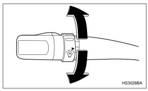
When the headlight switch is in the " <code>=DOE</code> " or " <code>=DO</code> " position, you can adjust brightness of the instrument panel illumination for better visibility.
