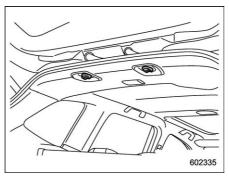
There are two hooks on the lining in the cargo area. Use them to hang or secure lightweight objects when the vehicle is stopped.
