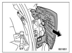
Slide the rear combination light assembly rearward to remove it from the vehicle.
