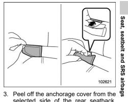
selected side of the rear seatback. Fold the peeled anchorage cover in half and affix it with hook and loop tape to expose the anchorages (bars) to be used for installation of the child restraint system.
