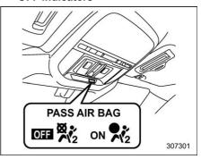
oN ♠ Front passenger's frontal airbag ON indicator
