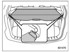
To extend the cover, pull the end of the cover out of the housing, then insert its hooks into the catches as shown. To rewind it, unhook it from the catches and it will rewind automatically. You should hold on to the cover and guide it back into the cover housing while it is rewinding.
