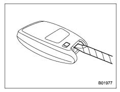
Wrap a flat-head screwdriver with vinyl tape or a cloth, and insert it in the gap to remove the cover.
