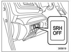
You can turn the SRH function on or off by pressing the SRH OFF switch.
