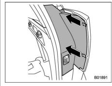
2. Push and move the cover to the forward to unlock the 2 tabs.
