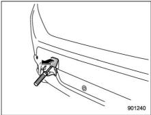
Cover the tip of a flat-head screwdriver with vinyl tape or cloth so that it will not scratch the bumper. Pry off the cover on the rear bumper using a screwdriver, and you will find a threaded hole for attaching the towing hook.
