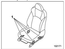
1 Occupant detection system sensors
