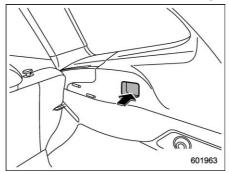
Insert the protrusion located on the right end of the sleeve into the recess of the retainer.
