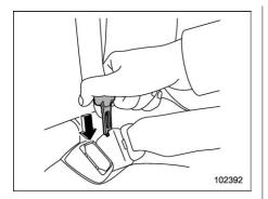
Insert a tongue plate or other hard pointed object into the slot in the anchor buckle on the right-hand side and push it in. The anchor tongue plate will then disconnect from the buckle.
