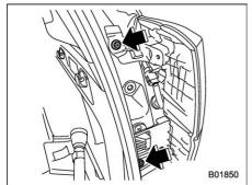
Using a Phillips screwdriver, remove the screws that secure the rear combination light assembly.
