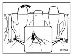
Pull the strap and adjust the seatback to the desired position.
