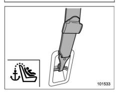
1. Attach the top tether hook to the appropriate upper anchorage.
