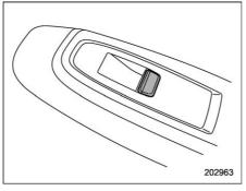
Each passenger's window can be controlled by the power window switch located on the door.
