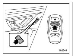
Hold the access key fob and press and hold the "SET" button, then press the "1" button of the access key fob.
