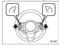
To upshift to the next higher gear position, pull the shift paddle that has "+" indicated on it. To downshift to the next lower gear position, pull the shift paddle that has "-" indicated on it
