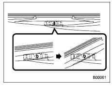
2. Turn the wiper blade assembly counterclockwise.
