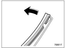
Pull out the end of the blade rubber assembly to unlock it from the plastic support.
