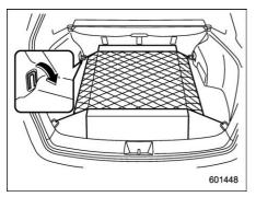
The cargo area is equipped with several tie-down hooks so that cargo can be secured with a cargo net or ropes.
