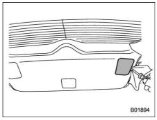
1. Apply a flat-head screwdriver to the light cover as shown in the illustration, and pry the light cover off from the rear gate trim.
