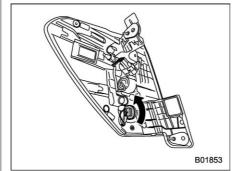
Remove the bulb socket from the rear combination light assembly by turning it counterclockwise.
