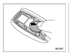
4. Insert a new battery with its positive (+) side facing upward as shown in the figure.
