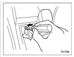
Wrap the tip of a flat-head screwdriver with vinyl tape or a cloth and use it to remove the shift lock cover. The shift lock release button is located under the shift lock cover
