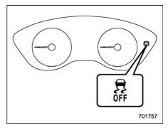
When the switch is pressed or turned during engine operation, the Vehicle Dynamics Control OFF indicator light "#" on the combination meter illuminates. The Vehicle Dynamics Control system will be deactivated and the vehicle will behave like a model not equipped with the Vehicle Dynamics Control system. When the switch is pressed again (type A) or turned to the "NORMAL" side (type B) to reactivate the Vehicle Dynamics Control system, the Vehicle Dynamics Control OFF indicator light turns off.
