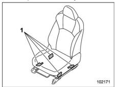
1 Occupant detection system sensors
