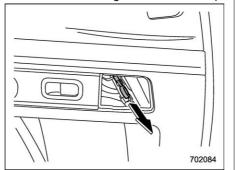
3. Pull the orange knob to unlock the fuel filler lid.
