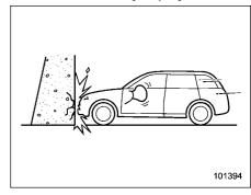
A head-on collision against a thick concrete wall at a vehicle speed of 12 to 19 mph (20 to 30 km/h) or higher activates only the driver's SRS frontal airbag or both driver's and front passenger's SRS frontal airbags. The airbag(s) will also be acti-
