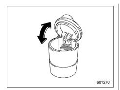
The portable ashtray can be installed in each cup holder or bottle holder. For the locations of the cup holders, refer to "Cup holders" \*P283. For the locations of the bottle holders, refer to "Bottle holders" \*P283.
