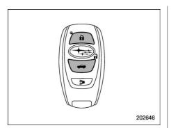
3. Press and hold the " $\mathbf{A}$ " button and " $\mathbf{A}$ " button on the access key fob simultaneously for more than 5 seconds.
