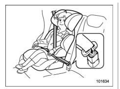
To remove the booster seat/cushion, press the release button on the seatbelt buckle and allow the belt to retract.
