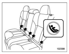
2. You will find "Q" marks at the bottoms of the rear seatback. These marks indicate the positions of the lower anchorages (bars).
