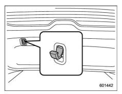
A convenience hook is attached to the rear gate trim. When the rear gate is open, you can hang a lantern, wet suit, etc. on the hook.
