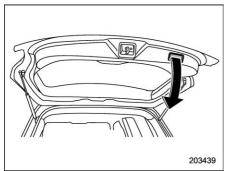
Lower the rear gate slowly and push down firmly until the latch engages.
