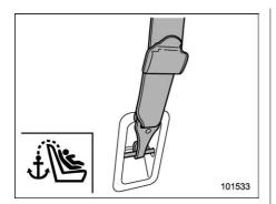
10. Latch the top tether hook onto the tether anchorage that is located behind the rear seat and tighten the top tether firmly. For additional instructions, refer to "Top tether anchorages" P75.
