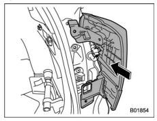
11. Put the rear combination light assembly into place while aligning the 2 pins with the holes and secure to the vehicle.
