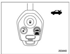
Power rear gate button on the transmitter
