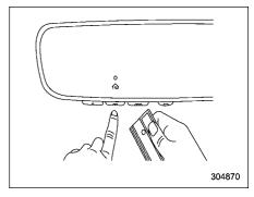
While the HomeLink indicator light is flashing orange, press and hold the hand-held remote button. Continue pressing the hand-held remote button until the HomeLink indicator light changes from orange to green. You may now release the hand-held remote button.
