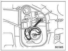
Install the light cover on the rear gate.
