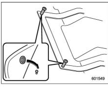
Retaining pins are located on the driver's side floor.
