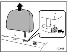
Remove the head restraint of the rear seating position where the child restraint system is to be installed. For details, refer to "Head restraints" P43.
