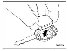
Remove the transmitter case from the key head.
