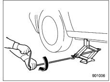
10. Insert the jack handle into the jackscrew, and turn the handle until the tire clears the ground. Do not raise the vehicle higher than necessary.
