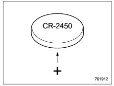
3. Remove the circuit board from the bottom half of the case and remove the battery and replace with new one. Be sure to observe the (+) sign on the old battery before removing it to ensure that the new battery is inserted prop-
