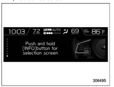
When the INFO button on the steering wheel is pressed and held on this screen, the setting screen can be displayed. For details, refer to "Setting screen" P214.
