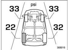
This screen displays each tire pressure. When a tire is deflated, the deflated tire and the tire pressure will be displayed on the screen in vellow.
