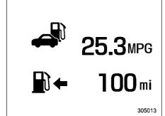
: Current fuel consumption □ ←: Driving range on remaining fuel
