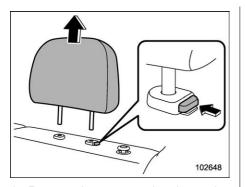
Remove the rear seat head restraint. For details, refer to "Head restraints" P43.
