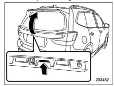
Keep pressing the rear gate opener button until it is unlocked (for approximately 5 seconds) and lift up the rear
