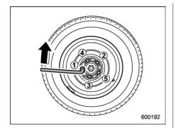
15. Use the wheel nut wrench to securely tighten the wheel nuts to the specified torque, following the tightening order in the illustration.
