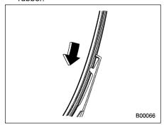
Align the claws of the plastic support with the grooves in the blade rubber assembly, then slide the blade rubber assembly into place.
