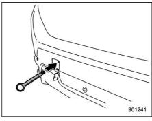
Screw the towing hook into the thread hole until its thread can no longer be seen.
