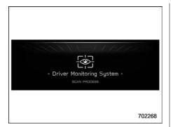
When the door is opened and the push-button ignition switch is OFF, the user recognition screen appears and the Driver Monitoring system starts user recognition.
