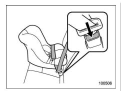
To remove the child restraint system, press the release button on the seatbelt buckle and allow the belt to retract completely. The belt will return to the FLR mode.
