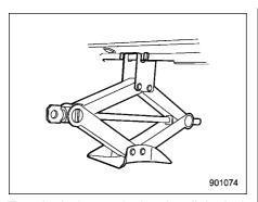
Turn the jackscrew by hand until the jack head engages firmly into the jack-up point.
