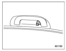
The coat hook is attached to each rear passenger's assist grip.
