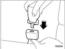
After confirming that the webbing is not twisted, insert the anchor tongue plate attached at the webbing end into the buckle on the right-hand side until a click sounds.
