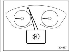
The indicator light on the combination meter will illuminate when the front fog lights are illuminated.
