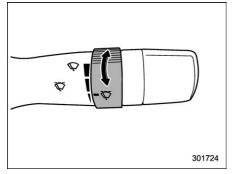
When the wiper switch is in the "Q" position, turn the dial to adjust the operating interval of the wiper. The operating interval can be adjusted in several steps from the shortest interval to the longest.
