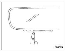
Return to the vehicle and firmly press, hold for two seconds and release the HomeLink button up to three times. At this point programming is complete and your device should operate when the HomeLink button is pressed and released.
