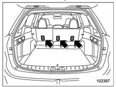
The tether anchorages (upper anchorages) are provided at the locations shown in the above illustration. For details, refer to "Top tether anchorages" @P75.
