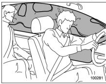
Models with SRS side airbags and SRS curtain airbags
