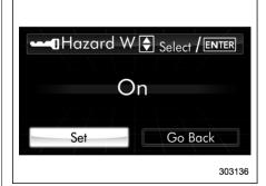
5. Select "Set" by operating the "▼" switch, and confirm the setting by pushing the witch.
