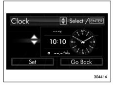
4. Select "Type A clock", "Type B clock", "Calendar" or "OFF" by operating the "▲" or "▼" switch and then push the ENTER button.
