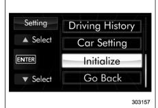
3. After the selection screen is displayed. operate the "A" or "V" switch to show the "Initialize" item. Then, push the enter button.
