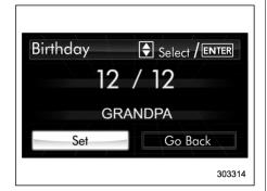
8. After entering the name by repeating step 7, select "Set" by operating the "\nleft\" switch and confirm the setting by pushing the \( \text{INTER} \) button.
