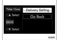
2. Operate the " $\blacktriangle$ " or " $\blacktriangledown$ " switch to select the "Delivery Setting" item, and then push the enter button.
