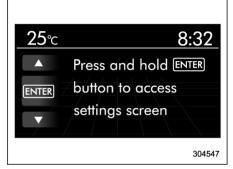
When the ENTER button is pushed and held, the selection screen can be displayed.
