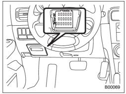
One is located under the instrument panel behind the cover on the driver's seat side. To remove the cover, pull it out.
