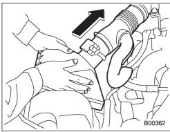
2. Push the air cleaner case cover in the direction of the arrow shown in the
