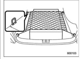
The cargo area is equipped with four tiedown hooks so that cargo can be secured with a cargo net or ropes.
