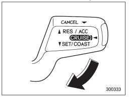
3. Push the control lever downward in the "SET/COAST" direction and release it. Then release the accelerator pedal.
