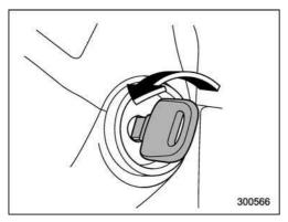
The key can be turned from "Acc" to "LOCK" only when the selector lever is in the "P" position.
