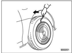
6. If your vehicle has wheel covers, insert the wheel cover remover into the notch provided in the wheel cover, and pry it off.
