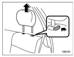
1. Remove the head restraint at the seating position where the child restraint system has been installed with the lower anchorages or seatbelt; lift up the head restraint while pressing the release button. Store the head restraint in the cargo area. Avoid placing the head restraint in the passenger compartment to prevent it from being thrown around in the passenger compartment in a sudden stop or a sharp turn.
