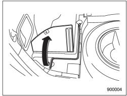
The jack handle is stowed under the rearleft and center lids in the cargo area.
