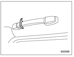
The coat hook is attached to the rear left passenger's hand grip.
