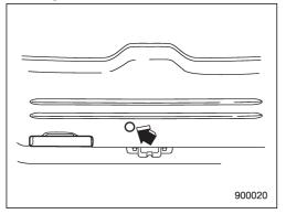
1. Remove the access cover at the bottom-center of the rear gate trim.
