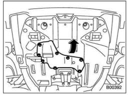
4. Open the access cover by removing the eight clips and turning the access cover counterclockwise. The drain plug will be exposed.
