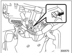
3. Turn the ignition key while pressing the key interlock release lever.
