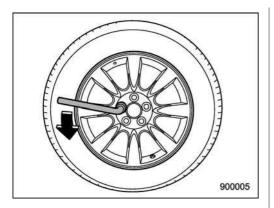
7. Loosen the wheel nuts using the wheel nut wrench but do not remove the nuts.
