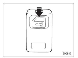
5. Before the electronic tone stops sounding, push the "LOCK" side of the power door lock switch the same number of times as the leftmost digit of the transmitter code. For example, push the lock switch 8 times if the leftmost digit of the code is 8.
