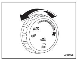
The fan operates only with the ignition switch in the "ON" position. The fan speed control dial is used to select the AUTO (automatic control) mode or to select the desired fan speed. The dial's positions and their functions are as follows:
