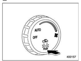
**ON position (Recirculation):** Interior air is recirculated inside the vehicle. Push the air inlet selection button to the ON position
