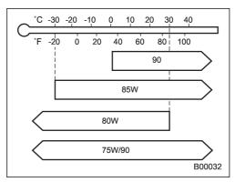
SAE viscosity No. and applicable temperature
