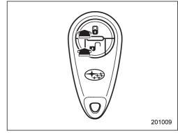
LOCK/ARM button Press to Lock all doors. Press and Hold to activate panic alarm. Press 3 times in a 5-second period to use vehicle finder function.
