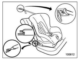
Some types of child restraint systems can be installed on the rear seat of your vehicle without use of the seatbelts. Such child restraint systems are secured to the designated anchorages provided on the vehicle body.
