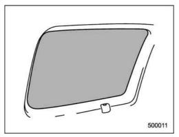
The antenna is printed on the inner surface of the left side rear quarter window glass.
