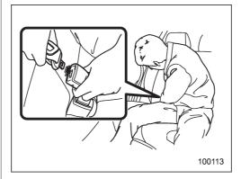
4. After confirming that the webbing is not twisted, insert the connector (tongue) attached at the webbing end into the buckle on the right-hand side until a click is heard.
