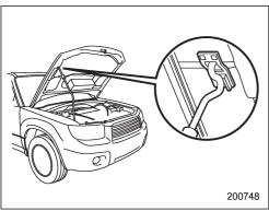
Lift up the hood, release the hood prop from its retainer and put the end of the
