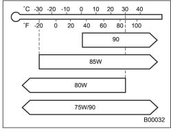
SAE viscosity No. and applicable temperature
