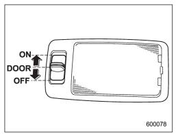
The dome light switch has three positions:
