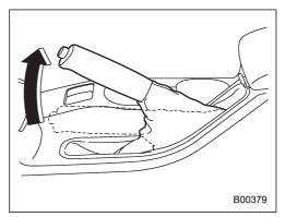
Check the parking brake stroke according to the maintenance schedule in the "Warranty and Maintenance Booklet". When the parking brake is properly adjusted, braking power is fully applied by pulling the lever up seven to eight notches gently but firmly (approximately 44 lbs, 196 N, 20 kg). If the parking brake lever stroke is not within the specified range, have the brake system checked and adjusted at your SUBARU dealer.
