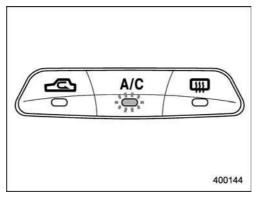
The air conditioner operates only when the engine is running.
