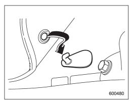
A retaining pin is located on the driver's side of the vehicle next to the fuel filler door release.
