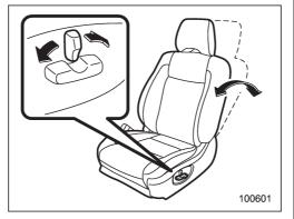
To adjust the angle of the seatback, move the control switch forward or backward.
