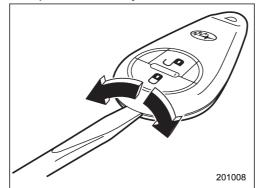
1. Open the transmitter case using a flathead screwdriver.
