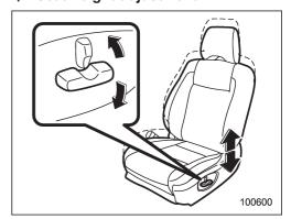
To adjust the seat height, pull up or push down the rear end of the control switch.
