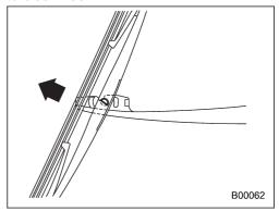
3. Having turned the wiper blade assembly to the angle shown in the illustration, pull it in the direction of the arrow to remove it from the wiper arm.
