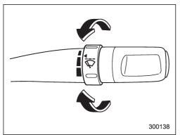
When the wiper switch is in the "\overline{\sigma}" position, turn the dial to adjust the operating interval of the wiper.
