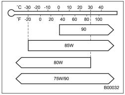
SAE viscosity No. and applicable temperature
