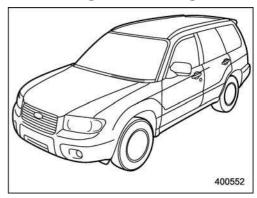
Always keep the front ventilation inlet grille free of snow, leaves, or other obstructions to ensure efficient heating and defrosting. Since the condenser is located in front of the radiator, this area should be kept clean because cooling performance is impaired by any accumulation of insects and leaves on the condenser
