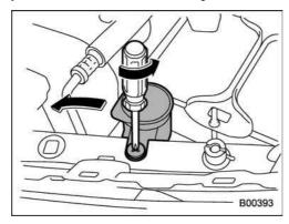
Before replacing the left-hand (battery-side) low- or high-beam light bulb, remove
