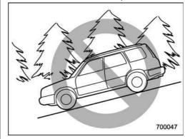
The Hill holder does not operate when the vehicle is facing downhill. And the Hill holder may not operate on slight grades.
