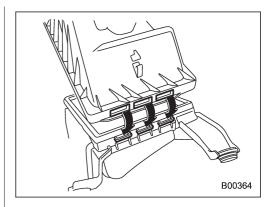
5. To install the air cleaner case cover, insert the three projections on the air cleaner case into the slits on the air cleaner case cover and then snap the two clamps on the air cleaner case cover.
