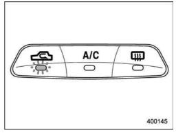
**ON position (Recirculation):** Interior air is recirculated inside the vehicle. Push the air inlet selection button to the ON position. The indicator light will come on.
