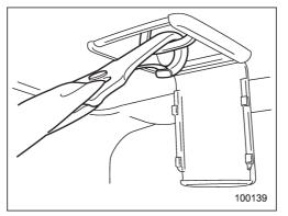
8. If the child restraint system requires a top tether, latch the hook onto the top tether anchor and tighten the top tether. See the "Top tether anchorages" for additional instructions.
