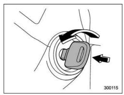
The key can be turned from "Acc" to "LOCK" only when the key is pushed in
