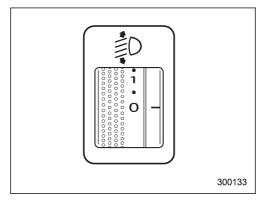
The HID headlights generate more light than conventional halogen headlights. Therefore a driver of an oncoming vehicle may experience too much glare when your headlight beam height adjustment is high due to the vehicle carrying a heavy load.
