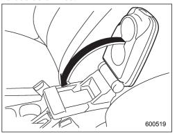
1. Tip the console top forward from its vertical position.
