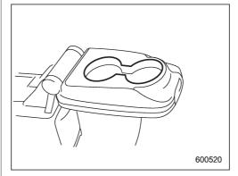
With the console top tipped toward the rear seat, it can be used as a cup holder.
