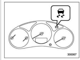
The indicator light turns on when the ignition switch is turned to the "ON" position; it turns off approximately 2 seconds later. This indicator light flashes during activation of the skid suppression function and is illuminated steadily during
