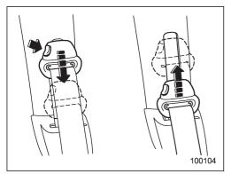
The shoulder belt anchor height should be adjusted to the position best suited for the driver/front passenger.
