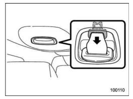
Rear center seatbelt is stowed in the recess of the ceiling.
