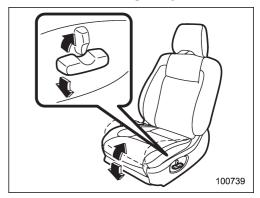
To adjust the seat cushion angle, pull up or push down the front end of the control switch.
