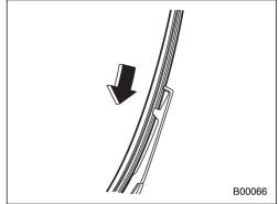
7. Align the claws of the plastic support with the grooves in the blade rubber assembly, then slide the blade rubber assembly into place.
