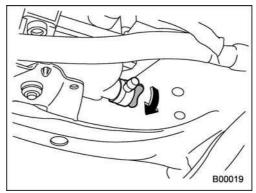
Always add genuine Subaru cooling system conditioner whenever the coolant is replaced.
