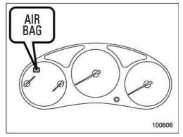
A diagnostic system continually monitors the readiness of the SRS airbag system (including front seatbelt pretensioners) while the vehicle is being driven. The SRS airbag system warning light "AR" will show normal system operation by lighting for approximately 6 seconds when the ignition switch is turned to the "ON" position.
