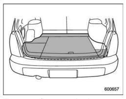
There are five trays in the storage compartment underneath the floor of the cargo area. They can be used to store
