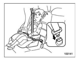
1. Place the booster seat in the rear seating position and sit the child on it. The child should sit well back on the booster
