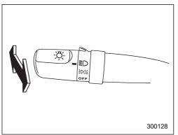
To change from low beam to high beam, push the turn signal lever forward. When the headlights are on high beam, the high beam indicator light "≣()" on the instrument panel is also on.
