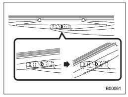
2. Turn the wiper blade assembly counterclockwise.
