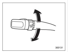
When the headlight switch is in the "soos" or "≣()" position, you can adjust brightness of the instrument panel illumination for better visibility.
