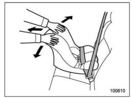
6. Push and pull the child restraint system forward and from side to side to check if it is firmly secured.
