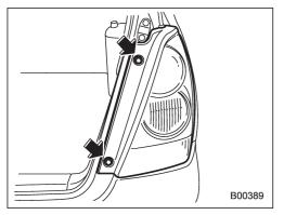
1. Remove the upper and lower screws. Then, slide the rear combination lamp assembly to the rear and remove it from the vehicle.
