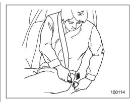
5. Insert the center seatbelt tongue plate into the center seatbelt buckle marked "CENTER" on the left-hand side until it clicks.
