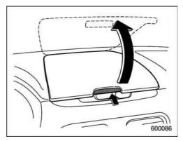
To open the dashboard compartment, push the button on the lid and the lid will automatically open. Be sure to close the compartment fully before driving.
