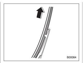
5. Pull the blade rubber assembly out of the plastic support.
