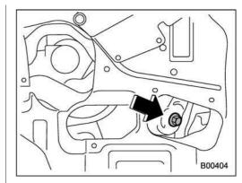
5. Drain out the engine oil by removing the drain plug while the engine is still warm. The used oil should be drained into an appropriate container and disposed of properly.
