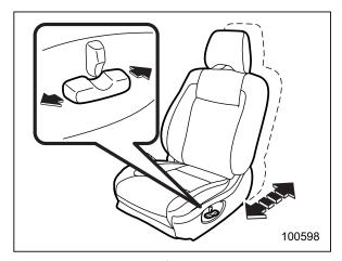
To adjust the seat forward or backward, move the control switch forward or backward.
