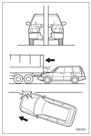
There are many types of collisions which might not necessarily require deployment
