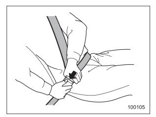
Push the button on the buckle. Before closing the door, make sure that the belts are retracted properly to avoid catching the belt webbing in the door.
