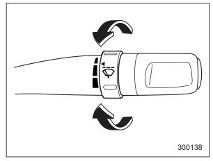
When the wiper switch is in the " \( \opi \) " position, turn the dial to adjust the operating interval of the wiper.
