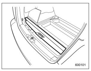
On models having a temporary spare tire, the cargo area cover can be stowed under the cargo floor.
