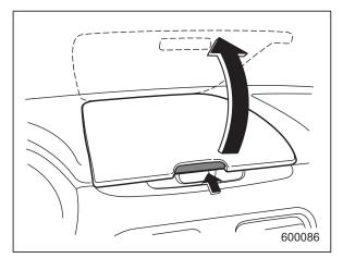
To open the dashboard compartment, push the button on the lid and the lid will automatically open. Be sure to close the compartment fully before driving.
