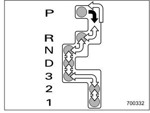
With the brake pedal depressed, move the lever along the gate.
