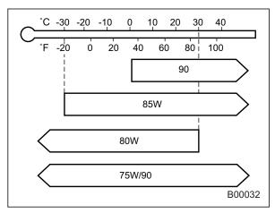
SAE viscosity No. and applicable temperature
