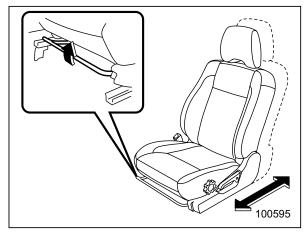
Pull the lever upward and slide the seat to the desired position. Then release the lever and move the seat back and forth to make sure that it is securely locked into place.
