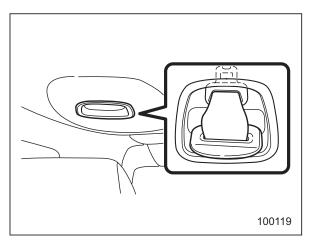
2. Allow the retractor to roll up the belt. You should hold the webbing end and guide it back into the retractor while it is rolling up. Neatly store the tongue plates in the recess on the ceiling and then insert the connector (tongue) plate into the slot located at the front of the recess.
