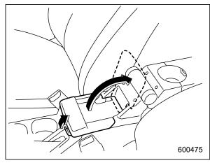
Raise the console top to the vertical position or tip it toward the rear seat. Then, pull up the lock button of the console box and open the lid.
