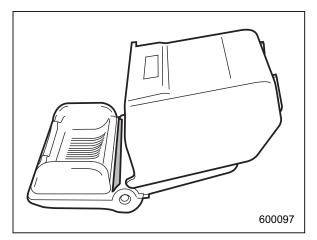
Particles of ash and tobacco will accumulate around the hinges of the ashtray's in-
