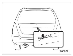
To open the rear gate, first unlock the rear gate lock then pull the outside handle up. Then, hold the rear gate and raise it as high as it will go.
