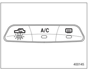
**ON position (Recirculation):** Interior air is recirculated inside the vehicle. Push the air inlet selection button to the ON position. The indicator light will come on.
