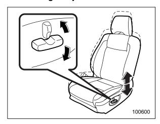
To adjust the seat height, pull up or push down the rear end of the control switch.
