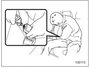
4. After confirming that the webbing is not twisted, insert the connector (tongue) attached at the webbing end into the buckle on the right-hand side until a click is heard. If the belt stops before reaching the buckle, return the belt slightly and pull it out more slowly. If the belt still cannot be unlocked, let the belt retract slightly after giving it a strong pull, then pull it out slowly again.
