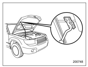
Lift up the hood, release the hood prop from its retainer and put the end of the hood prop into the slot in the hood. To close the hood:
