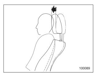
The front seats of your vehicle are equipped with active head restraints. They automatically tilt forward slightly in the event the vehicle is struck from the rear, decreasing the amount of rearward head movement and thus reducing the risk of whiplash. For maximum effectiveness the head restraint should be adjust so that the center of the head restraint is closest to the top of the occupant's ears.
