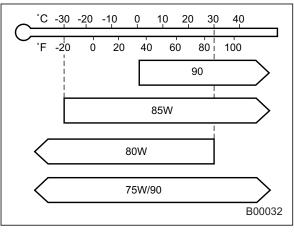
SAE viscosity No. and applicable temperature
