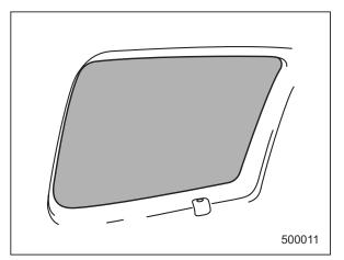
The antenna is printed on the inner surface of the left side rear quarter window glass.
