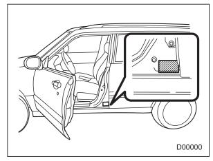
The certification plate attached to the driver's side door jamb shows GVWR (Gross Vehicle Weight Rating) and GAWR (Gross Axle Weight Rating).
