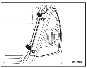
1. Remove the upper and lower screws. Then, slide the rear combination lamp assembly to the rear and remove it from the vehicle.
