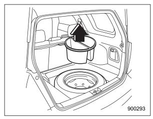
2. Remove the storage compartment bucket (Canada spec. non-turbo models).
