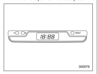
To set the hour, press the "H" button. To set the minutes, press the "M" button. To reset the minutes to "00" with a radio time signal, push the "Reset" button.
