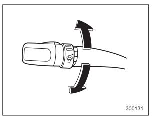
When the headlight switch is in the " ≡DOE" or " ≣D " position, you can adjust brightness of the instrument panel illumination for better visibility.
