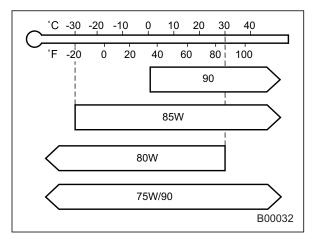
SAE viscosity No. and applicable temperature
