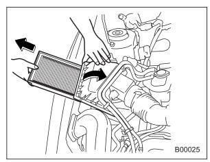
2. Open the air cleaner case cover and remove the air cleaner element.
