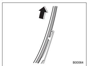
5. Pull the blade rubber assembly out of
