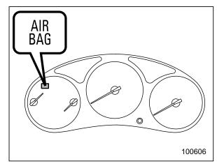
A diagnostic system continually monitors the readiness of the SRS airbag system (including front seatbelt pretensioners) while the vehicle is being driven. The SRS airbag system warning light "AIR Williams show normal system operation by lighting for approximately 6 seconds when the ignition switch is turned to the "ON" position.
