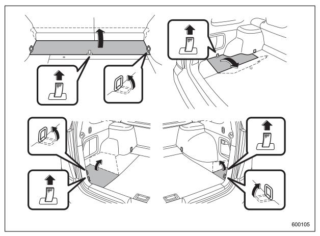
To open the lid, raise the cargo tie-down hooks and pull the tab up. The jack and jack handle are stored in the left side storage compartment.
