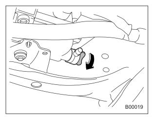
Always add genuine Subaru cooling system conditioner whenever the coolant is replaced.
