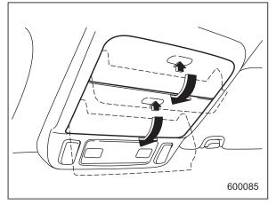
To open the console, push on the console lid lightly and the lid will automatically open.
