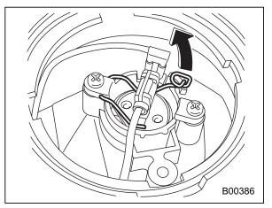
2. Remove the retainer spring, then pull out the bulb and electrical connector unit.
