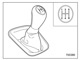
The shift pattern is shown on the shift lever knob. When shifting from 5th gear to reverse gear, first return the shift lever to the neutral position then shift into reverse gear.
