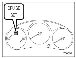
At this time, the "SET" indicator light is illuminated in the combination meter.
