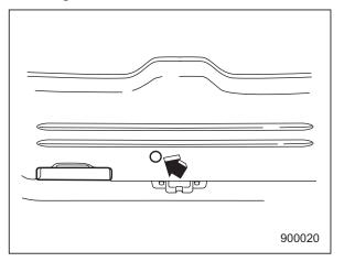
1. Remove the access cover at the bottom-center of the rear gate trim.
