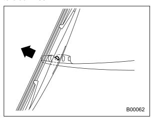
3. Having turned the wiper blade assembly to the angle shown in the illustration, pull it in the direction of the arrow to remove it from the wiper arm.
