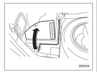
To take out the jack handle: Open the rear-left and center lids in the cargo area by pulling their tabs.
