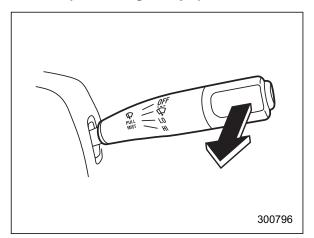
For a single wipe of the wipers, pull the lever toward you. The wipers operate until you release the lever.
