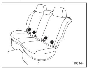
The lower anchorages (bars) are used for installing a child restraint system only on the rear seat window-side seating positions. For each window-side seating position, two lower anchorages are provided. Each anchor bar is located where the seat cushion meets the seatback.
