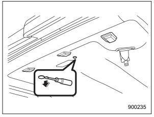
1. Remove the plug on the roof trim located to the rear of the moonroof by inserting the end of the flat-head screwdriver between the roof and plug and prying it off.
