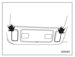
To turn on the map light, push the switch. To turn it off, push the switch again.
