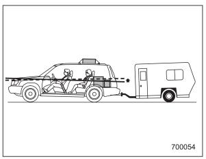
The self-leveling system is incorporated in the rear suspension shock absorber and operates only when the vehicle is in motion.
