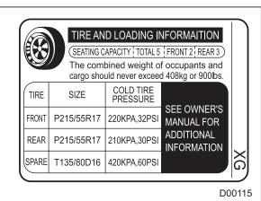
The vehicle placard shows original tire size, recommended cold tire inflation pressure on each tire at maximum loaded vehicle weight, seating capacity and loading information.
