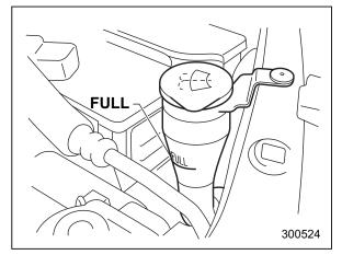
Remove the washer tank filler cap, then check the fluid level indicated by the level gauge (attached to the inside of the cap). If the level is near the "Low" mark, add flu-
