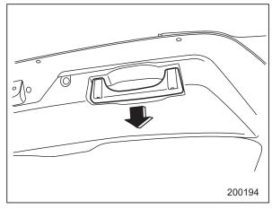
To close the rear gate, lower it slowly and push down firmly until the latch engages. The rear gate can be lowered easily if you pull down holding the recessed grip.
