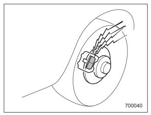
The disc brake pad wear warning indicators on the disc brakes give a warning noise when the brake pads are worn. If a squeaking or scraping noise is heard from the disc brakes while braking, immediately have your vehicle checked by your SUBARU dealer.
