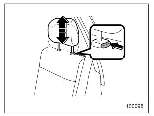
To raise the head restraint, pull it up. To lower it, push the head restraint down while pressing the release button on the top of the seatback.
