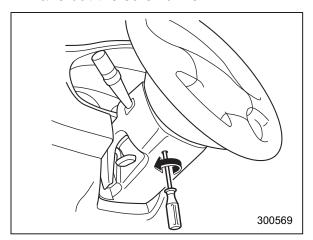
2. Remove the cover under the steering column using a Phillips screwdriver.
