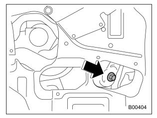
5. Drain out the engine oil by removing
