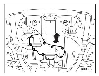
4. Open the access cover by removing the eight clips and turning the access cover counterclockwise. The drain plug will be exposed.
