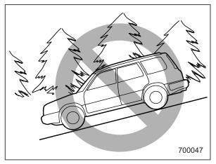
The Hill holder does not operate when the vehicle is facing downhill. And the Hill holder may not operate on slight grades.
