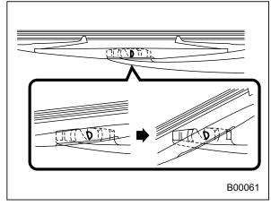
2. Turn the wiper blade assembly counterclockwise.
