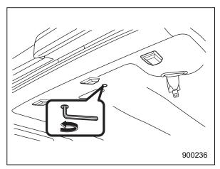
2. Insert a hex-headed wrench in the end of the motor shaft.
