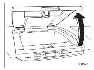
To adjust the clock, open the small article storage compartment in the dashboard with the vehicle parked in a safe place.
