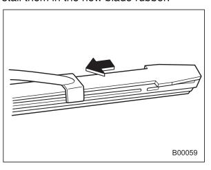
5. Align the claws of the metal support with the grooves in the rubber and slide the blade rubber assembly into the metal support until it locks.
