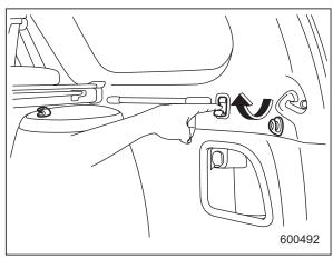
To use either of the retractable hooks, pull the lower portion out.
