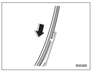
7. Align the claws of the plastic support with the grooves in the blade rubber assembly, then slide the blade rubber assembly into place.
