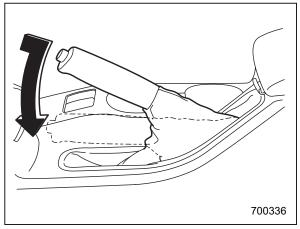
To release the parking brake, pull the lever up slightly, press the release button, then lower the lever while keeping the button pressed.
