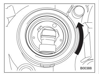
2. Remove the bulb from the headlight assembly by turning it counterclockwise.
