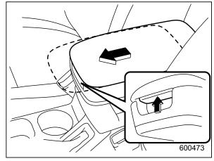
2. Push the armrest part of the console top forward to the desired position while pulling up the knob at the front end of the armrest and lock it in position by releasing the knob. Adjust the position of the armrest to suit your driving position. Make sure the armrest is securely retained.
