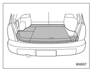
There are five trays in the storage compartment underneath the floor of the cargo area. They can be used to store small items.
