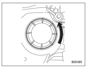
1. Remove the bulb cover, by turning it counterclockwise.
