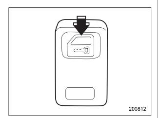
5. Before the electronic tone stops sounding, push the "LOCK" side of the power door lock switch the same number of times as the leftmost digit of the transmitter code. For example, push the lock switch eight times if the leftmost digit of the code is 8.
