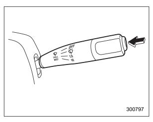
To wash the windshield, push the washer button at the end of the wiper control lever. The washer fluid sprays until you release the washer button. The wipers operate while you push the button.
