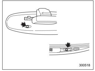
The mirror has a photosensor attached on both the front and back sides. If the glare from the headlights of vehicles behind you strikes the mirror, these sensors detect it and make the reflection surface of the mirror dimmer to help prevent you from being blinded. For this reason, use care not to
