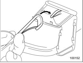
2. Open the cover flaps to use the anchorages. Fasten the top tether hook of the child restraint system to the appropriate top tether anchorage.
