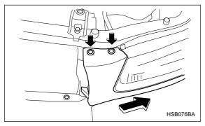
2. Remove the grille side cover by undoing the two clips and sliding the grille side cover toward the headlight.
