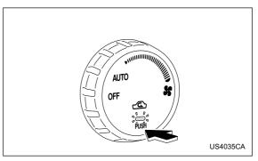
**ON position (Recirculation):** Interior air is recirculated inside the vehicle. Push the air inlet selection button to the ON position for fast cooling with the air conditioner or when driving on a dusty road. The indicator light will come on.
