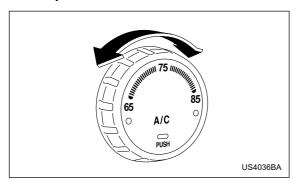
This dial is used to set the desired interior temperature. With the dial set to your desired temperature, the system automatically adjusts the temperature of air supplied from the outlets such that the desired temperature is achieved and maintained.
