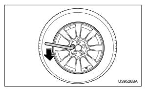
6. Loosen the wheel nuts using the wheel nut wrench but do not remove the nuts.
