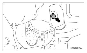
5. Drain out the engine oil by removing the drain plug while the engine is still warm. The used oil should be drained into an appropriate container and disposed of properly.
