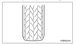
Roadholding is good, and steering is responsive. Rolling resistance is low, so fuel consumption is also lower.
