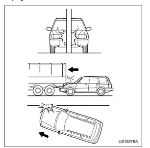
There are many types of collisions which might not necessarily require SRS frontal airbag deployment. If the vehicle strikes an object, such as a telephone pole or sign pole, or if it slides under a truck's load bed, or if it sustains an oblique offset frontal impact, the SRS frontal airbag may not deploy depending on the level of accident forces involved.
