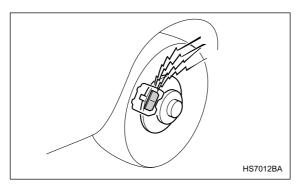
The right front disc brake and the right rear disc brake have audible wear indicators on the brake pads. If the brake pads wear close to their service limit, the wear indicator makes a very audible scraping noise when the brake pedal is applied.
