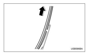
5. Pull the blade rubber assembly out of the plastic support.
