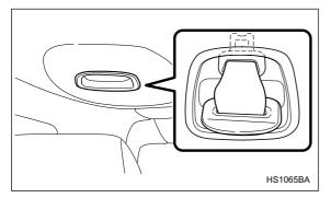
2. Allow the retractor to roll up the belt. You should hold the webbing end and guide it back into the retractor while it is rolling up. Neatly store the tongue plates in the recess in the retractor and then insert the connector (tongue) plate into the slot located at the front of the recess.
