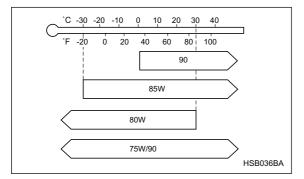
SAE viscosity No. and applicable temperature
