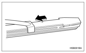
5. Align the claws of the metal support with the grooves in the rubber and slide the blade rubber assembly into the metal support until it locks.
