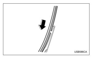
7. Align the claws of the plastic support with the grooves in the blade rubber assembly, then slide the blade rubber assembly into place.
