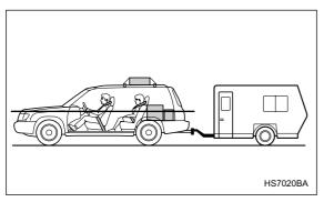
Owing to the self-leveling suspension, the vehicle body is adjusted to the proper position after several drive trips, even if the rear of the vehicle is lowered by loaded cargos or a coupled trailer.
