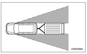
After hitching a trailer to your vehicle, check that the standard side mirrors provide a good rearward field of view without significant blind spots. If significant blind spots occur with the vehicle's standard side mirrors, use towing mirrors that conform with Federal, state/province and/or other applicable regulations.
