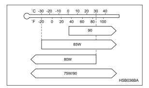
SAE viscosity No. and applicable temperature
