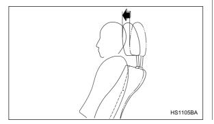
The front seats of your vehicle are equipped with active head restraints. They automatically tilt forward slightly in the event the vehicle is struck from the rear, decreasing the amount of rearward head movement and thus reducing the risk of whiplash. For maximum effectiveness the head restraint should be adjust so that the center of the head restraint is closest to the top of the occupant's ears.
