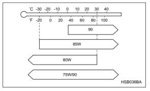
SAE viscosity No. and applicable temperature
