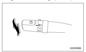
To change from low beam to high beam, push the turn signal lever forward. When the headlights are on high beam, the high beam indicator light " ≣⊘ " on the instrument panel is also on.
