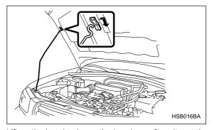
Lift up the hood, release the hood prop from its retainer and put the end of the hood prop into the slot in the hood.
