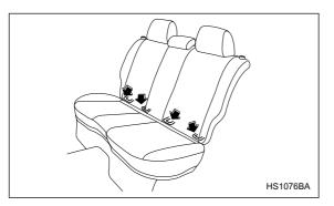
The lower anchorages (bars) are used for installing a child restraint system only on the rear seat window-side seating positions. For each window-side seating position, two lower anchorages are provided. Each anchor bar is located where the seat cushion meets the seatback.
