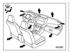
Heat-def: Windshield defroster outlets. foot outlets and both side outlets of the instrument panel (Refer to "Defrosting" ☞P278.)
