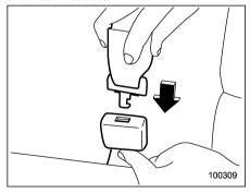
3. After confirming that the webbing is not twisted, insert the anchor tongue plate attached at the webbing end into the buckle on the right-hand side until a click
