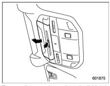
To open the console, push up the lid lightly that is located on the "PUSH" mark and it will automatically open.
