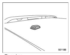
Mouse type The roof antenna is installed on the roof.
