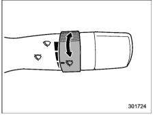
When the wiper switch is in the position, turn the dial to adjust the operating interval of the wiper. The operating interval can be adjusted in several steps from the shortest interval to the longest.
