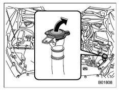
Remove the washer tank filler cap, then add windshield washer fluid.
