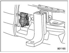
Hitch harness connector (7-pin type)
