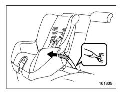
6. If your child restraint system is a flexible attachment type (which uses tether belts to connect the child restraint system properly to the lower anchorages).
