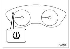
The tire pressure monitoring system provides the driver with the warning message indicated by sending a signal from a sensor that is installed in each wheel when tire pressure is severely low.
