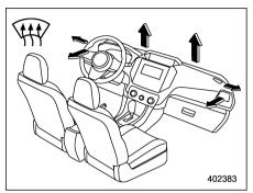
**Defrost:** Windshield defroster outlets and both side outlets of the instrument panel (Refer to "Defrosting" P278.)
