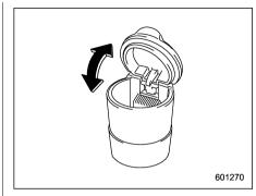
The portable ashtray can be installed in each cup holder or bottle holder. For the locations of the cup holders, refer to "Cup holders" P293. For the locations of the bottle holders, refer to "Bottle holders" ₱P294.
