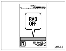
After the brake pedal is depressed, the Reverse Automatic Braking system OFF indicator will illuminate and the system will temporarily stop operating. The Reverse Automatic Braking system OFF indicator will turn off when the select lever is shifted to a position other than the "R" position.
