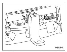
Hitch harness connector (4-pin type)
