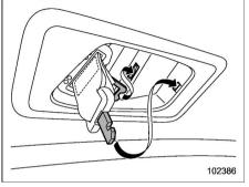
3. With the belt held by hand, allow the retractor to roll up the belt slowly. You should hold the webbing end and guide it back into the retractor while it is rolling up. Neatly store the tongue plate in the recess on the ceiling and then insert the tongue plate and anchor tongue plate into the slot as shown in the illustration.
