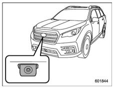
The image from the camera mounted inside the front grille is displayed in the multi-function display (color LCD).
