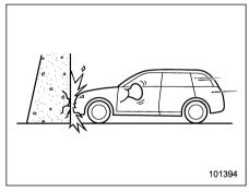
A head-on collision against a thick concrete wall at a vehicle speed of 12 to 19 mph (20 to 30 km/h) or higher activates only the driver's SRS frontal airbag or both driver's and front passenger's SRS frontal
