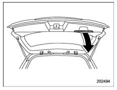
Lower the rear gate slowly and push down firmly until the latch engages.
