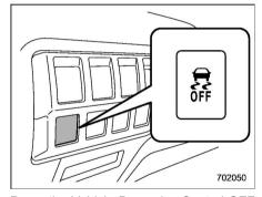
Press the Vehicle Dynamics Control OFF switch to deactivate the Vehicle Dynamics Control system. Creating adequate driving wheel slip by deactivating the Vehicle Dynamics Control system may help to recover from the loss of traction. Use the Vehicle Dynamics Control OFF switch as necessary.
