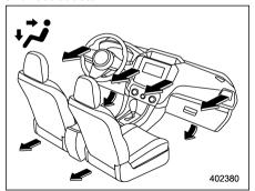
Bi-level: Instrument panel outlets and foot outlets
