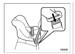
9. To remove the child restraint system, press the release button on the seatbelt buckle and allow the belt to retract completely. The belt will return to the ELR mode.
