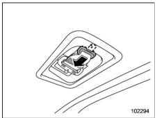
The center seatbelt is stowed in the recess of the ceiling.
