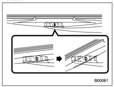
2. Turn the wiper blade assembly counterclockwise.
