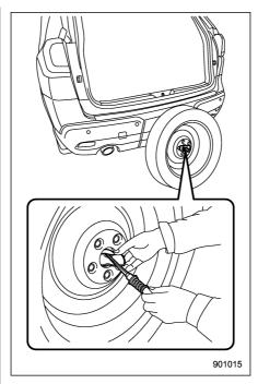
2. Insert the retainer through the center hole of the temporary tire as showing in the figure.
