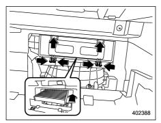
Replace the cabin air filter with a new one and then reinstall the cover.
