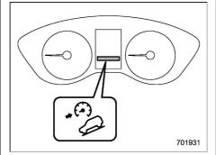
This indicator appears while the hill descent control function is in the standby mode. It flashes while the function is
