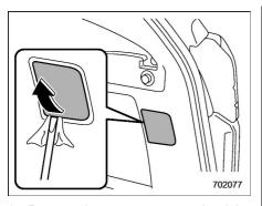
1. Remove the access cover at the rightside of the cargo area trim using a flathead screwdriver.
