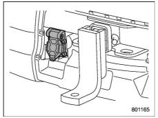
Hitch harness connector (7-pin type)
