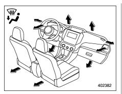
Heat-def: Windshield defroster outlets. foot outlets and both side outlets of the instrument panel (Refer to "Defrosting" @P274.)
