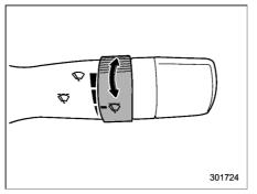
When the wiper switch is in the "\subsetep" position, turn the dial to adjust the operating interval of the wiper. The operating interval can be adjusted in several steps from the shortest interval to the longest.
