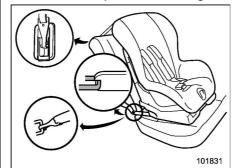
Some types of child restraint systems can be installed on the rear seat of your vehicle without use of the seatbelts. Such child restraint systems are secured to the designated anchorages provided on the seat. The lower and top tether anchorages are sometimes referred to as the LATCH system (Lower Anchors and Tethers for CHildren).
