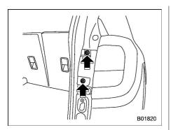
2. Using a Phillips screwdriver, remove the upper and lower screws that secure the rear combination light assembly.
