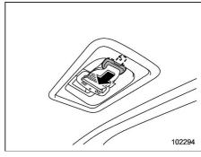
Center seatbelt is stowed in the recess of the ceiling.
