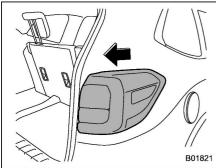
3. Slide the rear combination light assembly rearward and remove it from the vehicle.
