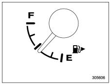
The fuel gauge shows the approximate amount of fuel remaining in the tank. When the ignition switch is in the "LOCK"/ "OFF" or "ACC" position, the fuel gauge shows "E" even if the fuel tank contains fuel
