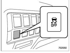
Press the Vehicle Dynamics Control OFF switch to deactivate the Vehicle Dynamics Control system. Creating adequate driving wheel slip by deactivating the Vehicle Dynamics Control system may help to recover from the loss of traction. Use the Vehicle Dynamics Control OFF switch as necessary.
