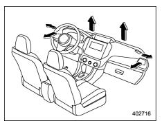
Select the "\(\vec{\psi}\)" or "\(\vec{\psi}\)" mode to defrost or dehumidify the windshield and front door windows
