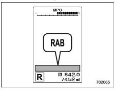
If the Reverse Automatic Braking System malfunctions, the above indicator illuminates on the combination meter. Contact the nearest SUBARU dealer for details.
