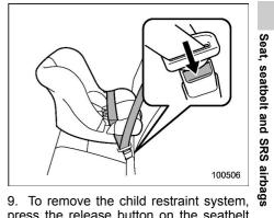
press the release button on the seatbelt buckle and allow the belt to retract completely. The belt will return to the FIR mode.
