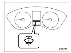
When there is only a small amount of washer fluid remaining, the windshield washer fluid warning light will illuminate. When this occurs, refill the washer fluid.
