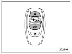
3. Press and hold the "♠" button and "➡" button on the access key fob simultaneously for more than 5 seconds.
