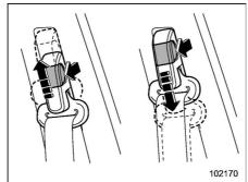
The shoulder belt anchor height should be adjusted to the position best suited for the driver/front passenger. Always adjust the anchor height so that the shoulder belt passes over the middle of the shoulder without touching the neck.
