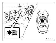
2. While holding the access key fob and pressing the "SET" button, press the "a" button of the access key fob.
