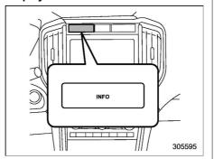
Pressing the INFO button on the instrument panel changes the display to the following sequence.
