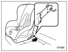
5. While following the instructions supplied by the child restraint system manufacturer, connect the lower hooks onto the lower anchorages located at "©" marks on the bottom of the rear seatback. When the hooks are connected, make sure the adjacent seatbelts are not caught.
