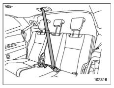
3. Insert the tongue plate into the buckle and position the seatbelt comfortably.
