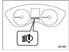
The LED headlight warning light illuminates if the LED headlights malfunction. Have your vehicle inspected at a SUBARU dealer as soon as possible.
