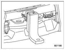
Hitch harness connector (4-pin type)
