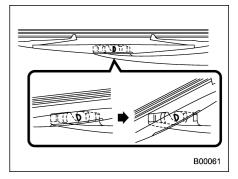
2. Turn the wiper blade assembly counterclockwise
