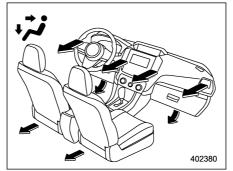
Bi-level: Instrument panel outlets and foot outlets
