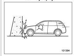
A head-on collision against a thick concrete wall at a vehicle speed of 12 to 19 mph (20 to 30 km/h) or higher activates only the driver's SRS frontal airbag or both driver's and front passenger's SRS frontal
