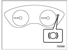
Auto Vehicle Hold operation indicator light While the vehicle is kept held by the Auto
