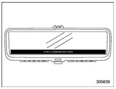
When the vehicle communication error. the warning indicators will appear as shown in the illustration.
