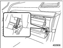
(2) Remove the damper shaft from the glove box.
