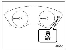
When the switch is pressed with the ignition switch in the "ON" position, the Vehicle Dynamics Control OFF indicator light "A" on the combination meter illuminates. The Vehicle Dynamics Control system will be deactivated and the vehicle will behave like a model not equipped with the Vehicle Dynamics Control system. When the switch is pressed again to reactivate the Vehicle Dynamics Control system, the Vehicle Dynamics Control OFF indicator light turns off.
