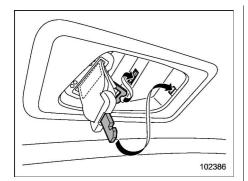
3. With the belt held by hand, allow the retractor to roll up the belt slowly. You should hold the webbing end and guide it back into the retractor while it is rolling up. Neatly store the tongue plate in the recess on the ceiling and then insert the tongue plate and connector (tongue) plate into the slot as shown in the following illustration.
