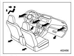
Ventilation 2: Instrument panel outlets and foot outlets
