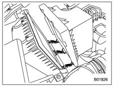
5. To install the air cleaner case (rear), insert the three projections on the air cleaner case (rear) into the slits on the air cleaner case (front).
