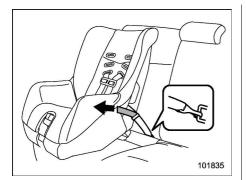
6. If your child restraint system is a flexible attachment type (which uses tether belts to connect the child restraint system properly to the lower anchorages).
