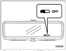
**Dimming mirror mode OFF indicator**When turning the dimming mirror mode
