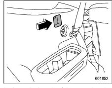
3. Insert both ends of the cover housing into the recesses of the retainers.
