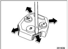
3. Open the transmitter case by releasing the hooks.
