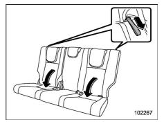
4. While pulling the straps, fold down the seatbacks.
