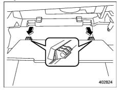
(4) Pull out the glove box horizontally and remove the hinge portion. When
