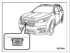
The image from the camera mounted inside the front grille is displayed in the multi-function display (color LCD).
