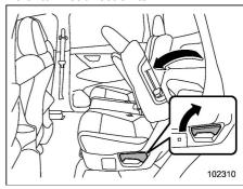
5. Pull the lever and tilt the seatback forward.
