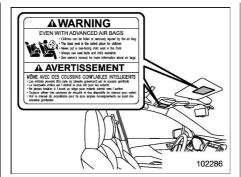
Your vehicle has warning labels on the driver's and front passenger's sun visors beginning with the phrase "EVEN WITH ADVANCED AIR BAGS" and a tag attached to the glove box lid beginning with the phrase "Even with Advanced Air Bags". Make sure that you carefully read the instructions on the warning labels and tag.
