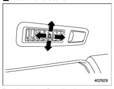
To adjust the airflow direction, move the tab. To close the ventilator, move the tab all the way rearward.
