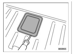
4. Open the cover located at the center of the luggage floor by screwdriver.
