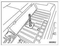
6. Fit the two extensions onto the hexhead hoist shaft end.
