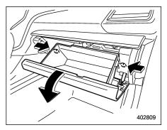
(3) Push in the stoppers located on both sides of the glove box and then pull down the glove box as far as it will go.
