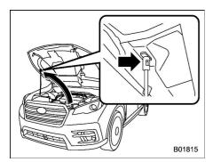
4. Lift up the hood, release the hood prop from its retainer and put the end of the hood prop into the slot in the hood.
