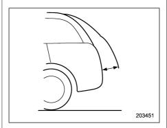
The rear gate cannot be paused when it is in the approximately 2 in (5 cm) range from the fully closed position. The system will ignore any button operation and the rear gate will continue to open.
