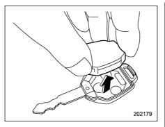
2. Remove the transmitter case from the key head.
