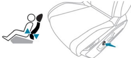
The control allows independent adjustment of the depth and vertical position of the lumbar support.
