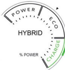
**POWER** **High power demand, using the combined capabilities of the petrol engine and the electric motor.**
