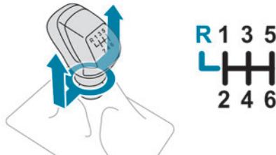
► Raise the ring under the knob and move the gear selector to the left, then forwards.
