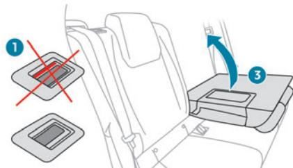
▶ Straighten the backrest 3 and push it firmly to latch it into place.
